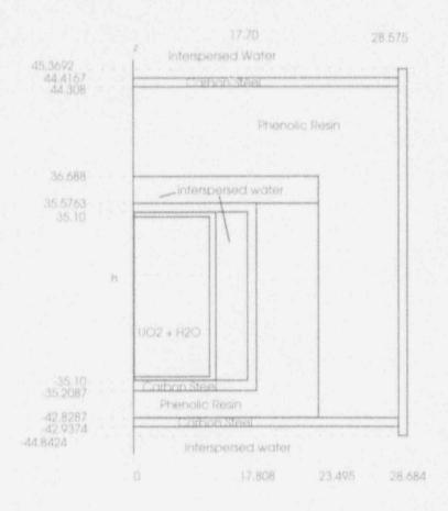
Figure 2. GEMER Geometry Model for BU-7 Container
