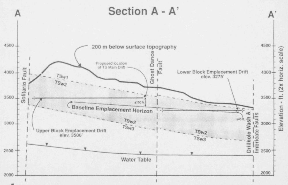
Note: Plane of section cuts through lowest emplacement drift in step-block layout.
