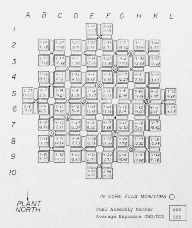
FIGURE 4 - EXPECTED FUEL EXPOSURE DISTRIBUTION NEAR END OF CYCLE 8. CORE AVERAGE EXPOSURE SHOWN IS 12,890 MWD/MTU.
