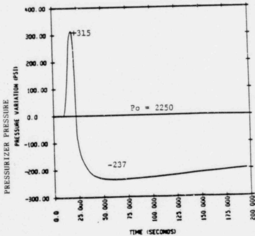
Figure 4-1 Overtemperature  $\Delta T$  Trip - Reference Case
