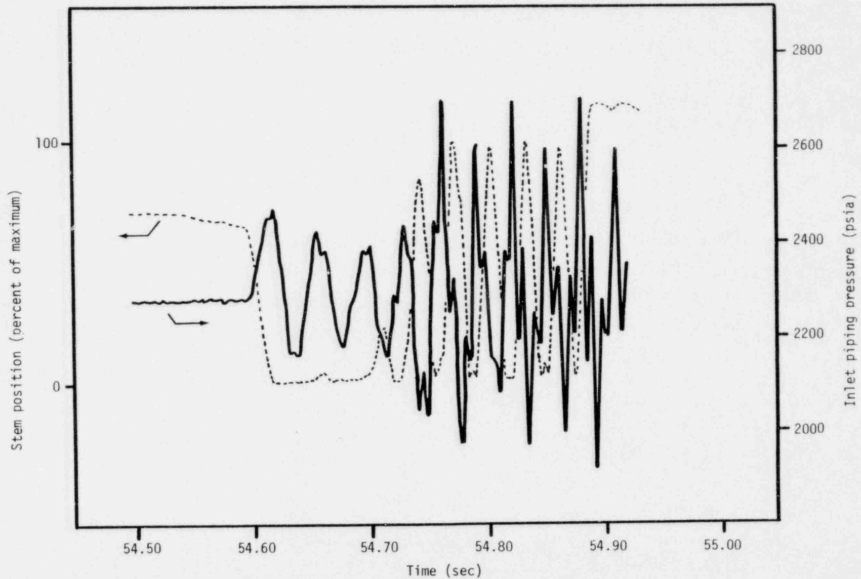
FIGURE 3-13. ONSET OF CHATTER FOLLOWING CLOSING FOR CROSBY 6M6 VALVE
