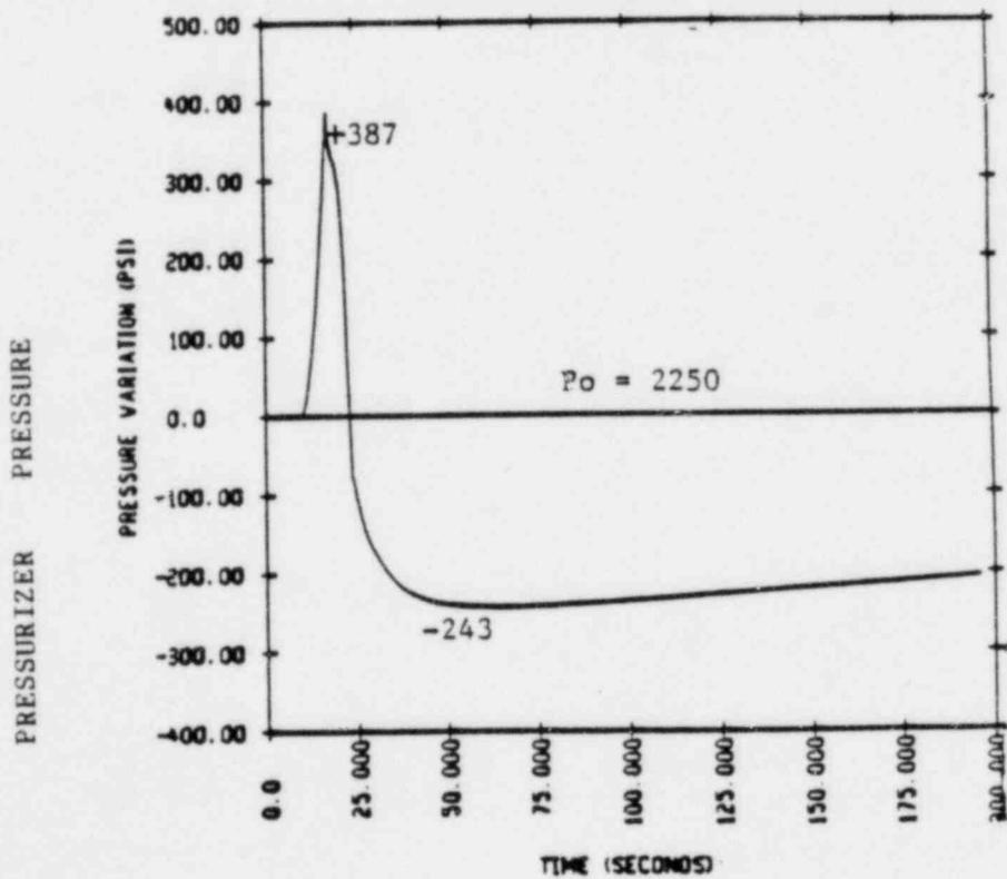
Figure 4-4 Overtemperature  $\Delta T$  Trip - 1.6 Sec Delay
