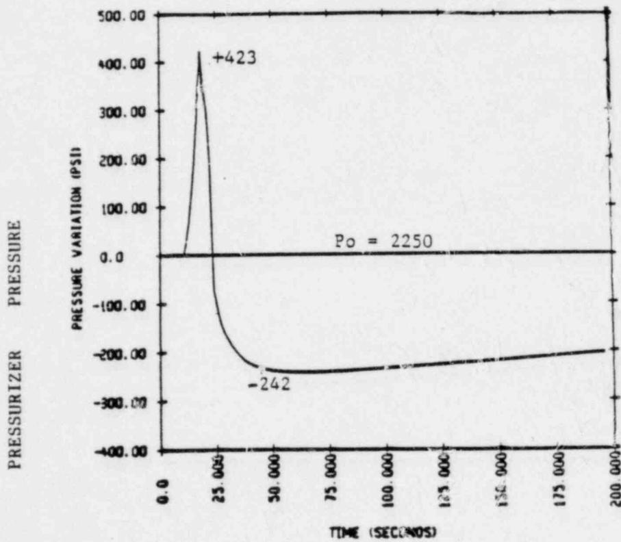
Figure 4-5 Overtemperature  $\Delta T$  Trip - 2.0 Sec Delay
