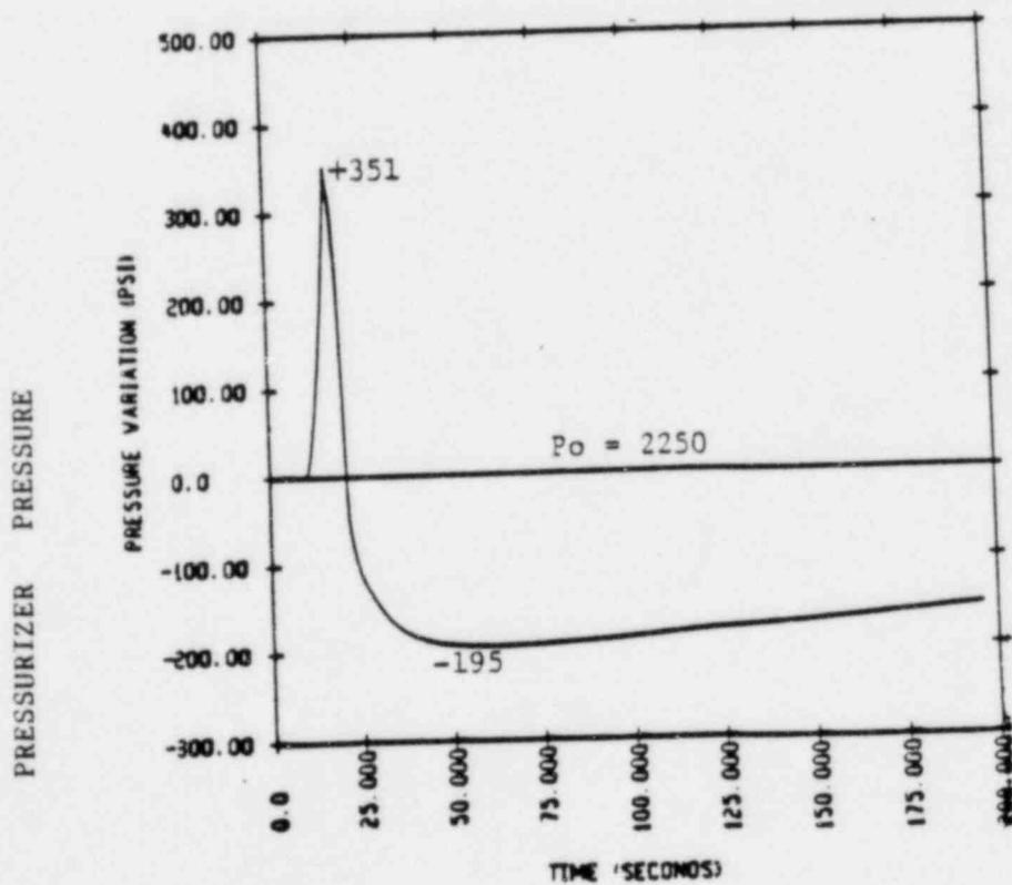
Figure 4-2 High Pressurizer Pressurer Trip - 1.2 Sec Delay
