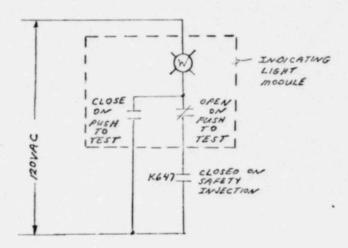
The K647 Relay is the Output Latch Relay for the Safety Injection Latch Relay K602 as shown in the following sketch:
