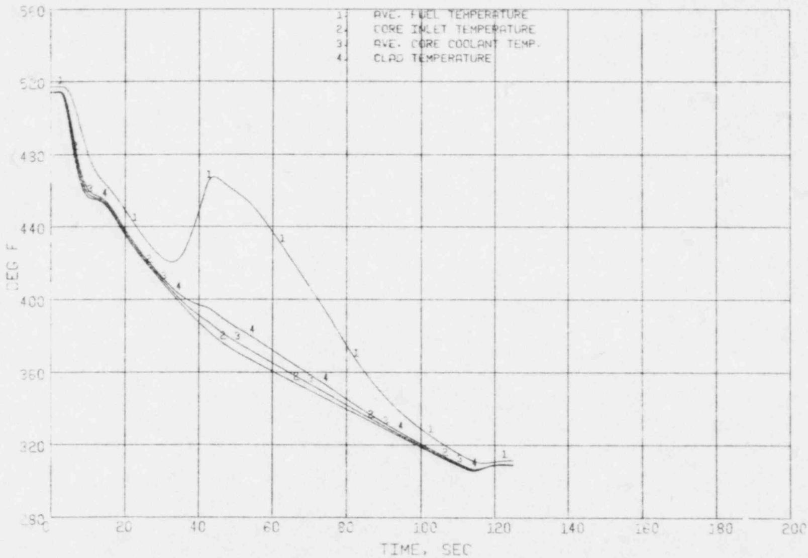
Figure 3.41 Large Steam Line Break (514°) - Core Temperature Response
