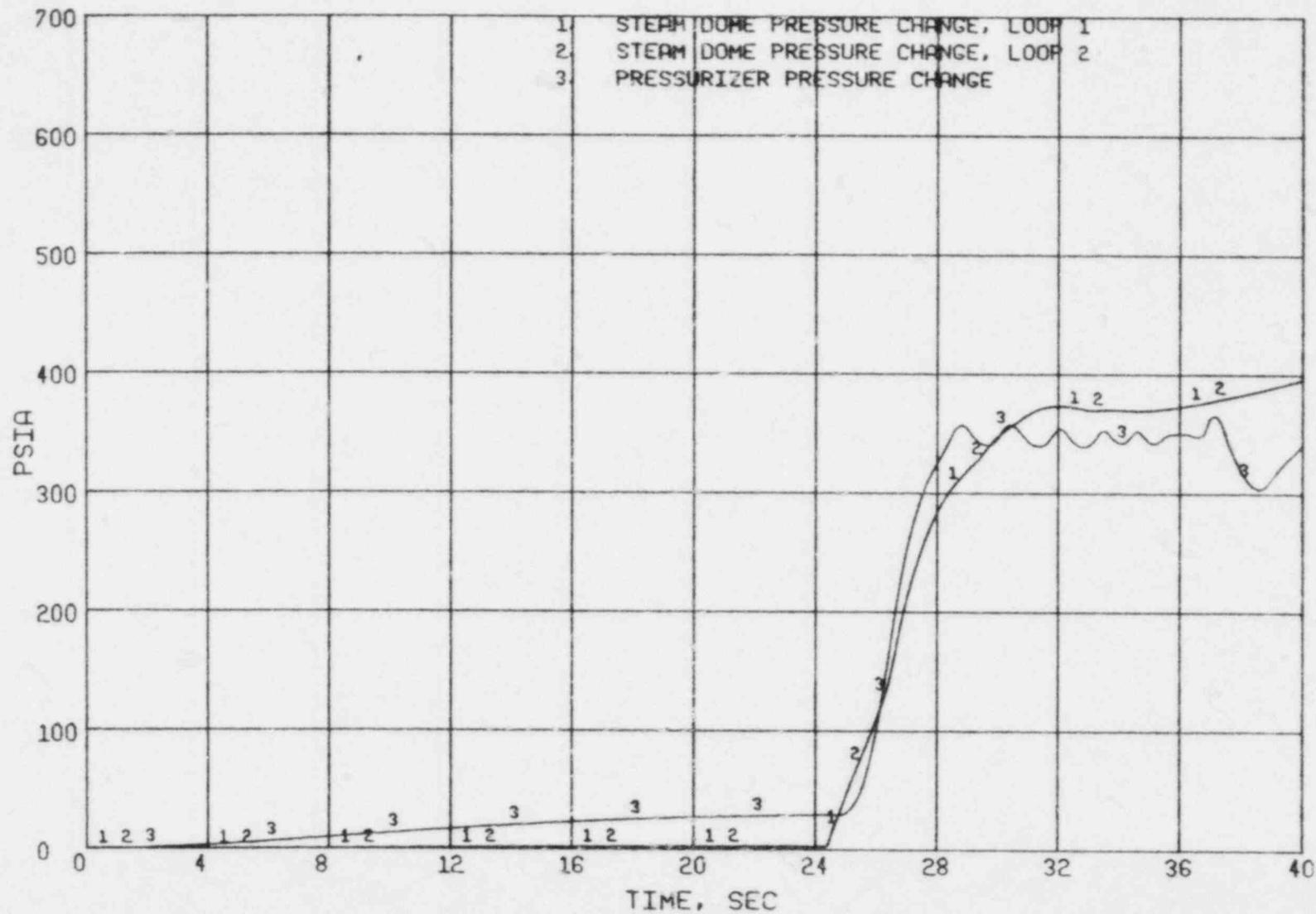
Figure 3.11 Uncontrolled Rod Withdrawal (Slow) - Pressure Changes
