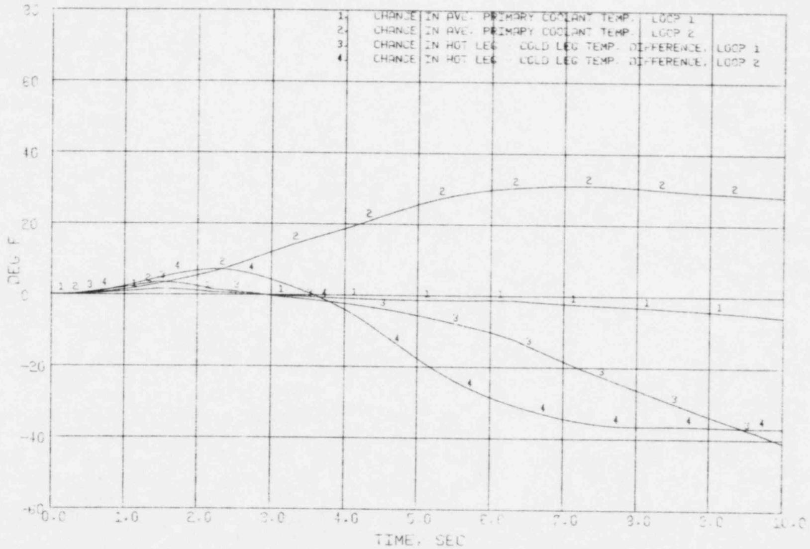
Figure 3.22 Locked Rotor - Primary Loop Temperature Changes
