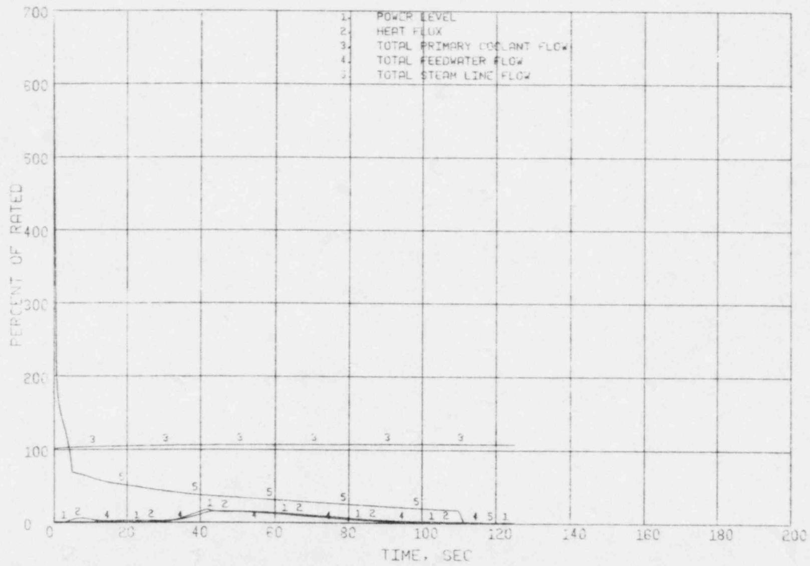
Figure 3.40 Large Steam Line Break (514°) - Power, Heat Flux and System Flows
