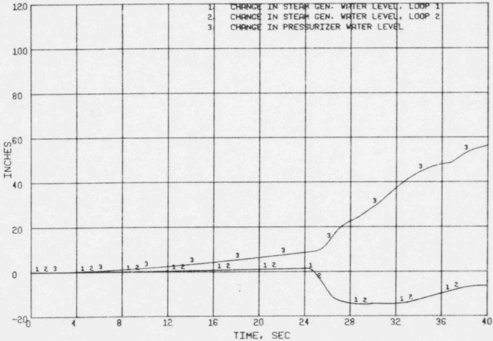
Figure 3.12 Uncontrolled Rod Withdrawal (Slow) - Level Changes
