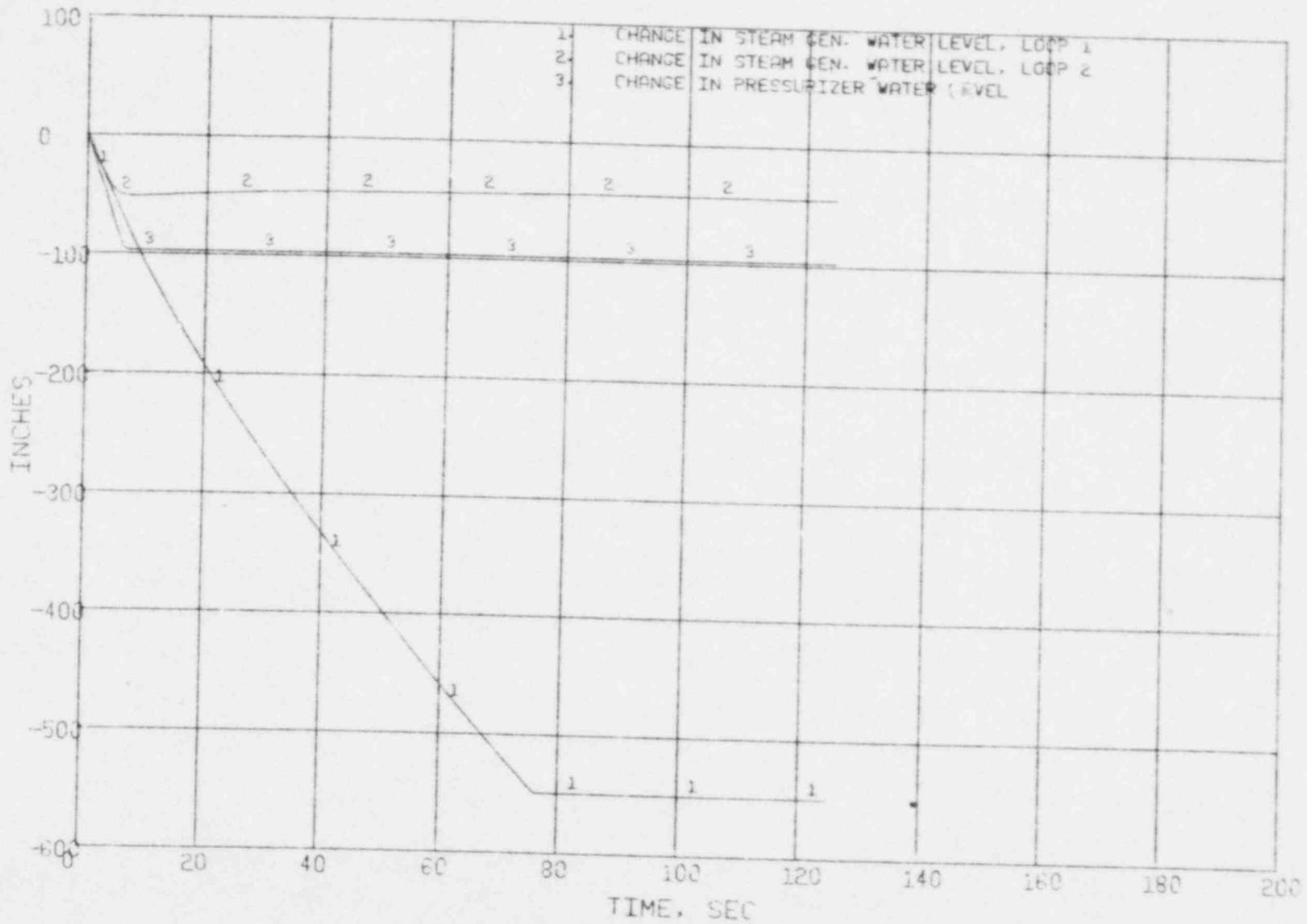
Figure 3.38 Large Steam Line Break (547°) - Level Changes
