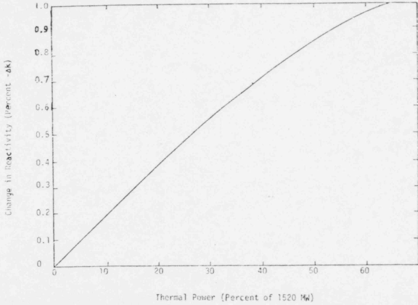
Figure 3.32 Variation of Reactivity with Power At Constant Core Average Temperature
