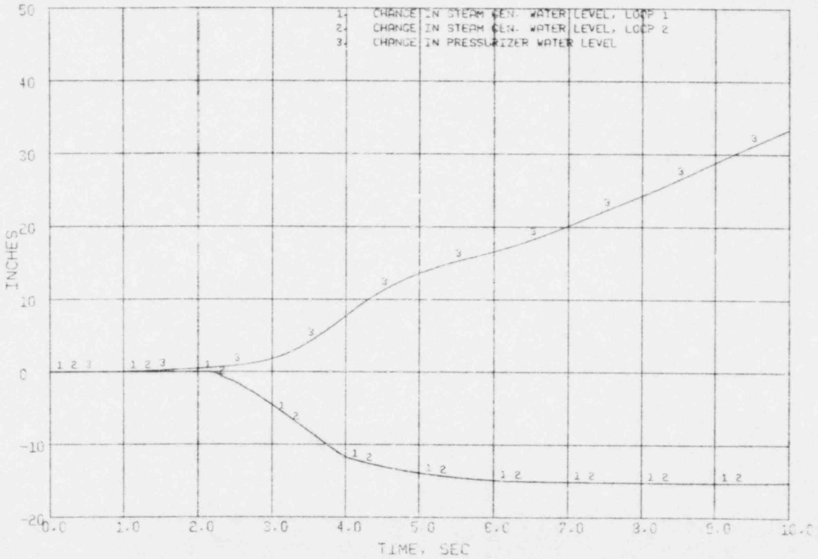
Figure 3.5 Uncontrolled Rod Withdrawal (Fast) Level Changes
