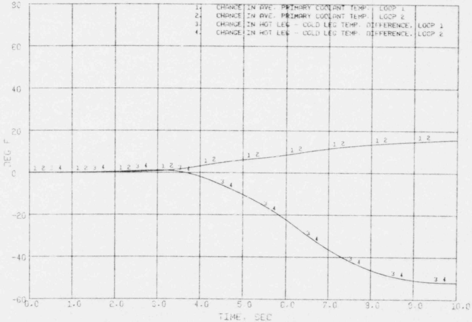
Figure 3.3 Uncontrolled Rod Withdrawal (Fast)
