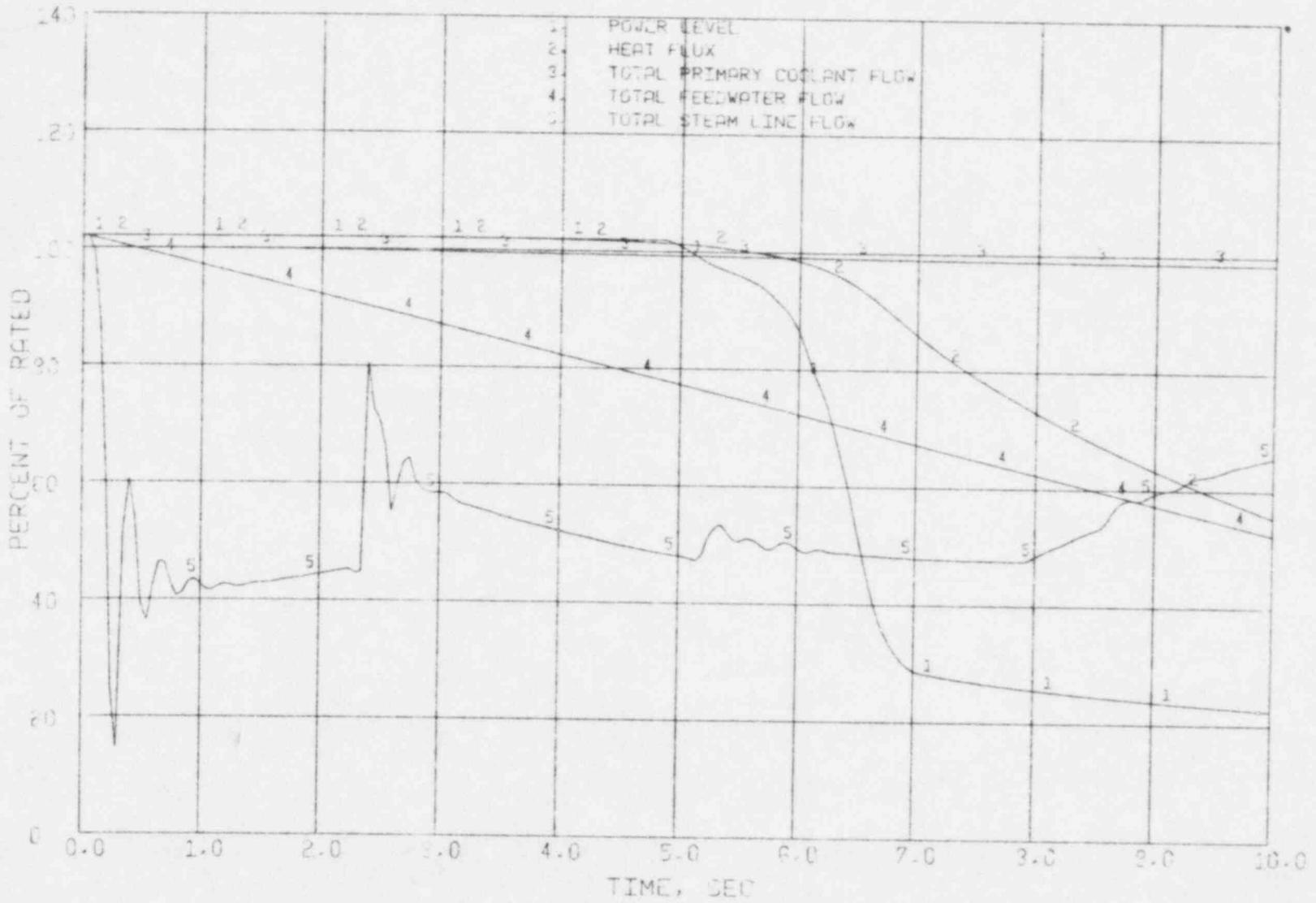
Figure 3.26 Loss of Electric Load
