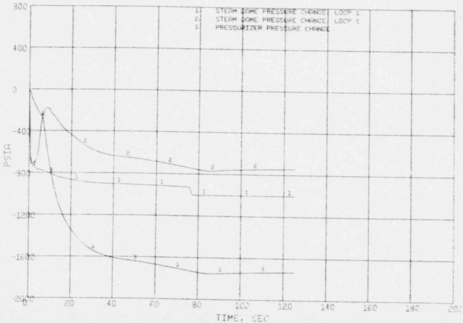
Figure 3.37 Large Steam Line Break (547°) - Pressure Changes
