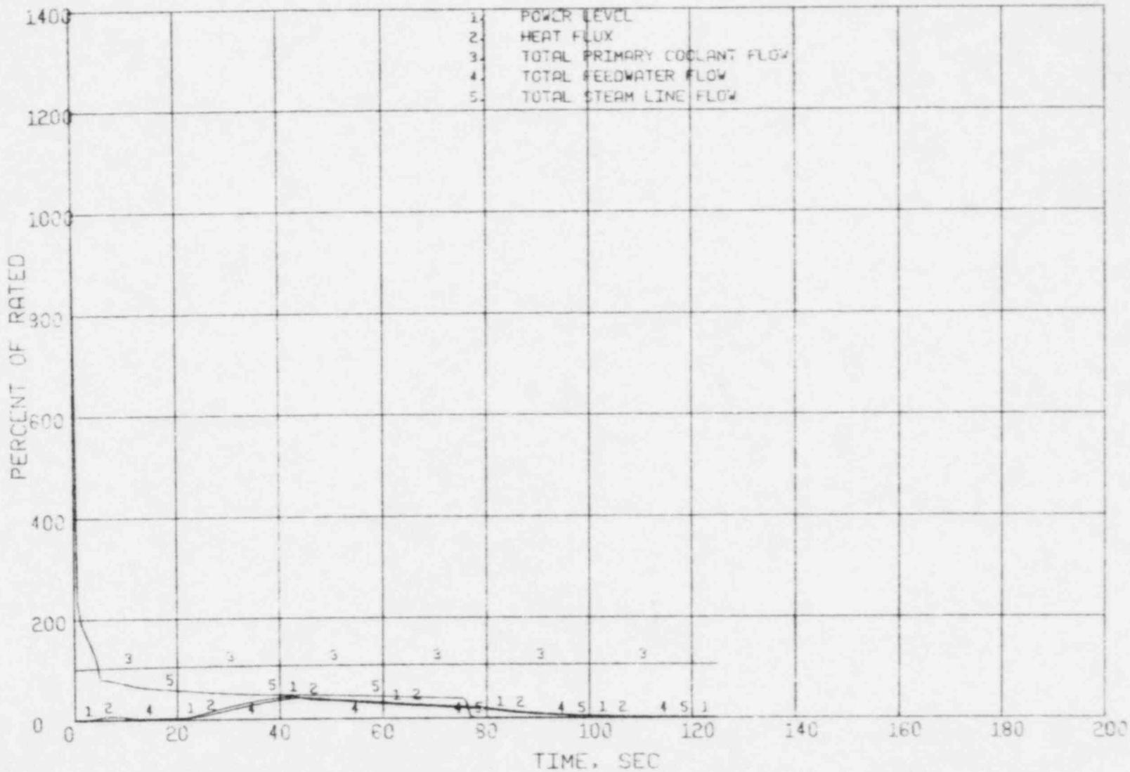
Figure 3.34 Large Steam Line Break (547') - Power, Heat Flux and System Flows
