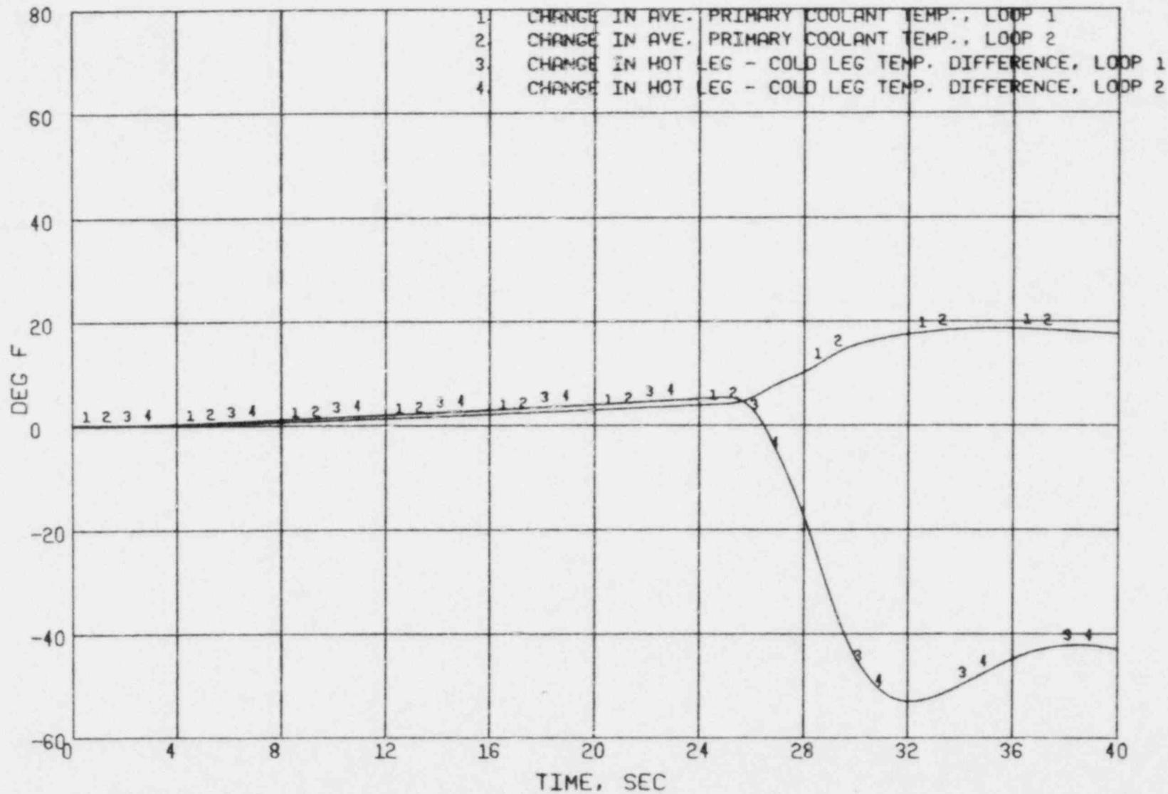
Figure 3.10 Uncontrolled Rod Withdrawal (Slow) - Primary Loop Temperature Changes
