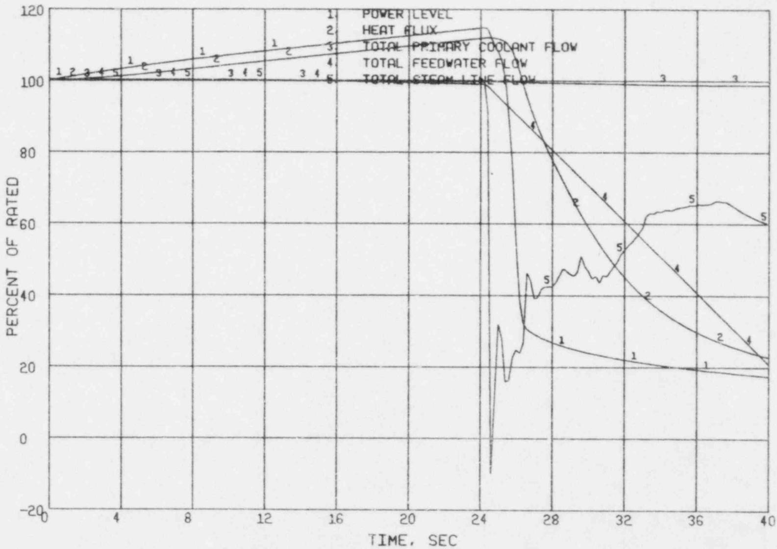
Figure 3.8 Uncontrolled Rod Withdrawal (Slow) - Power, Heat Flux and System Flows
