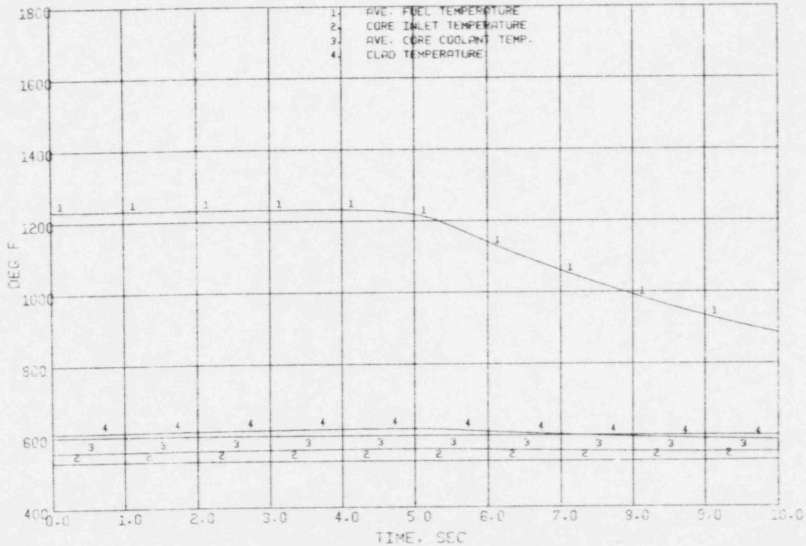
Figure 3.15 Loss of Coolant Flow - Core Temperature Response
