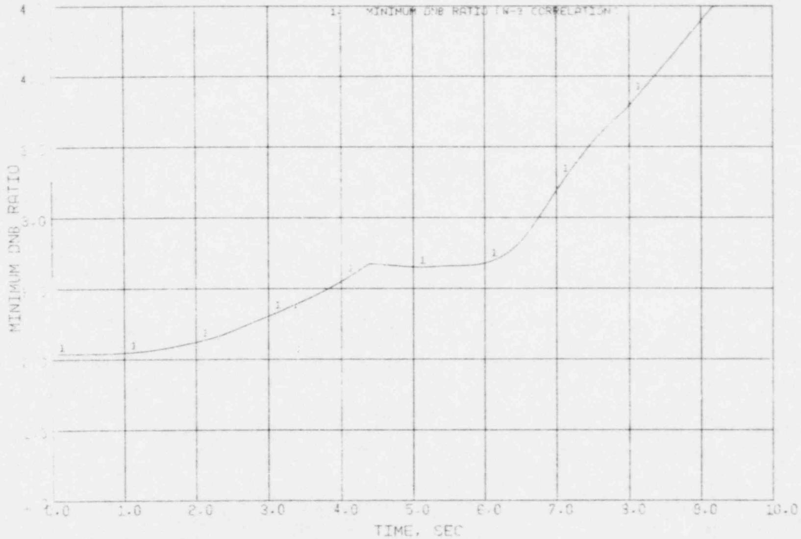
Figure 3.31 Loss of Electric Load - Minimum DNB Ratio
