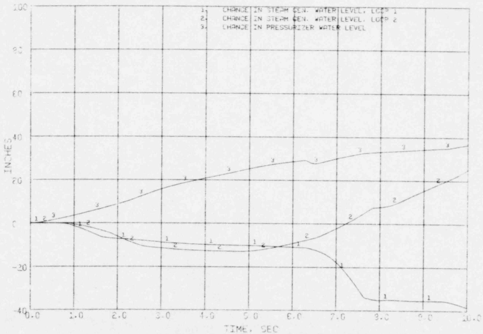
Figure 3.24 Locked Rotor - Level Changes
