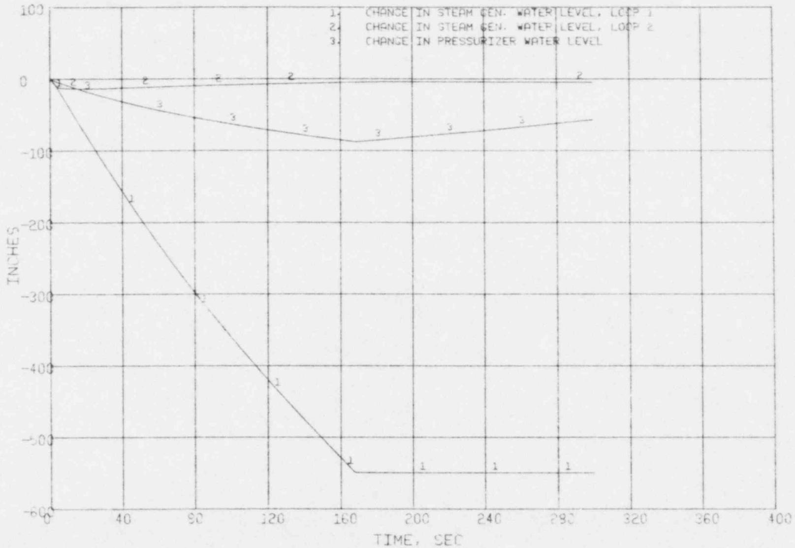
Figure 3.50 Small Steam Line Break (547) - Level Changes
