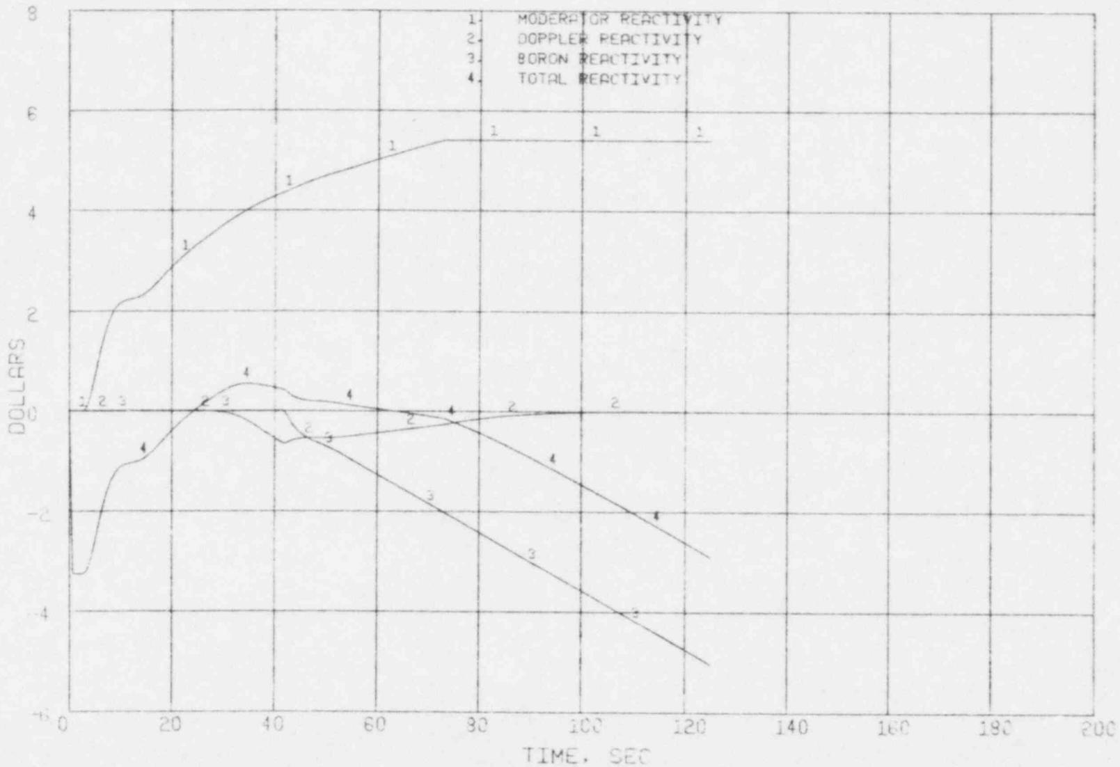
Figure 3.45 Large Steam Line Break (514<sup>0</sup>) - Reactivity
