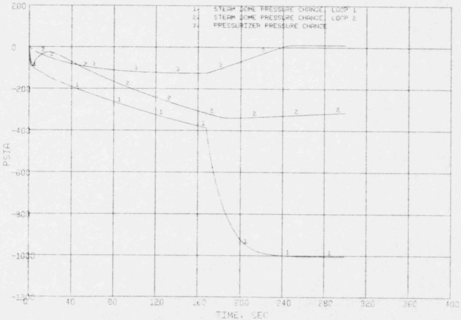
Figure 3.49 Small Steam Line Break (547<sup>0</sup>) - Pressure Changes
