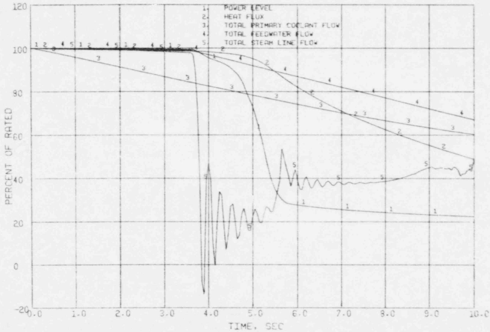
Figure 3.14 Loss of Coolant Flow - Power, Heat Flux and System Flows
