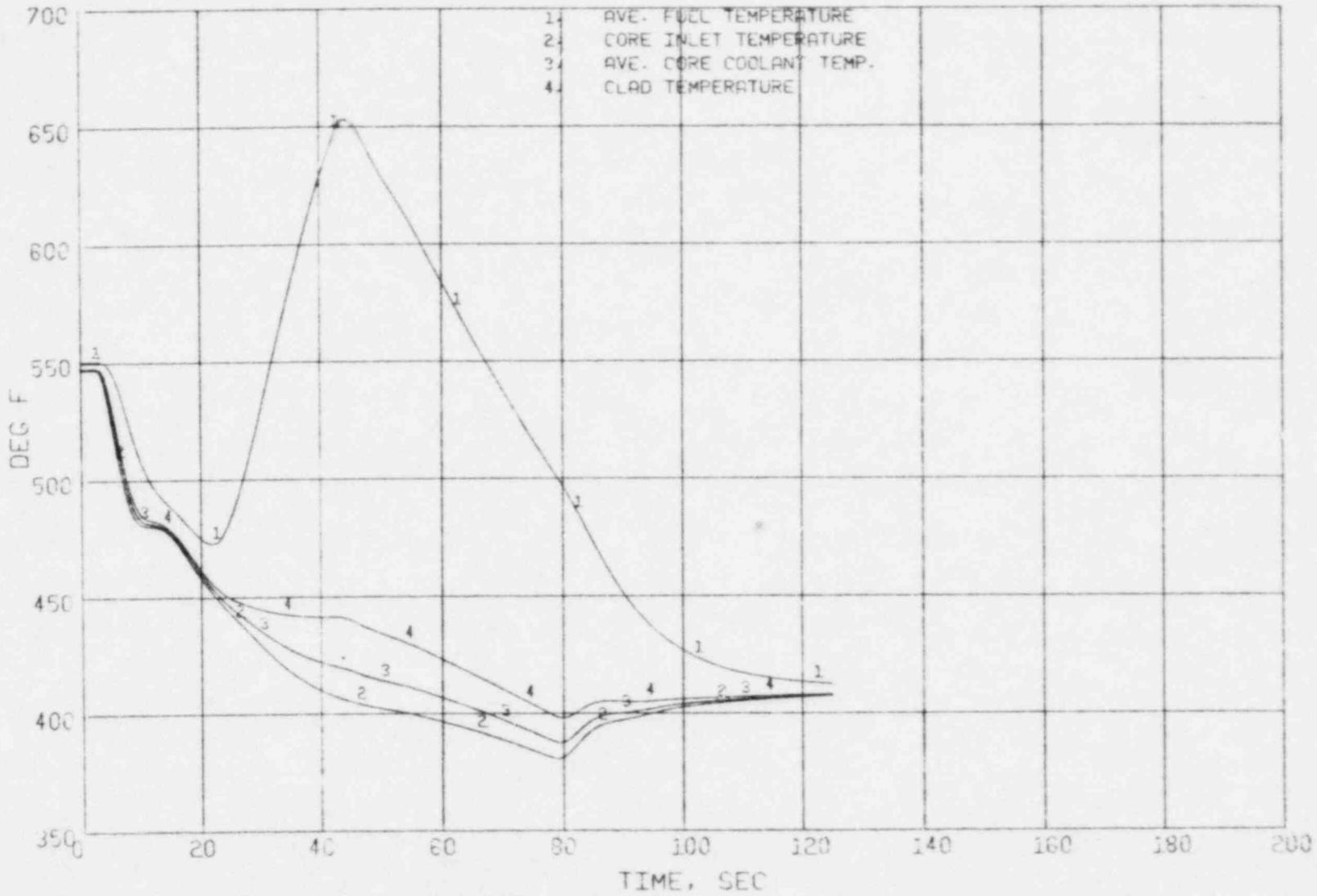
Figure 3.35 Large Steam Line Break (547<sup>0</sup>) - Core Temperature Response
