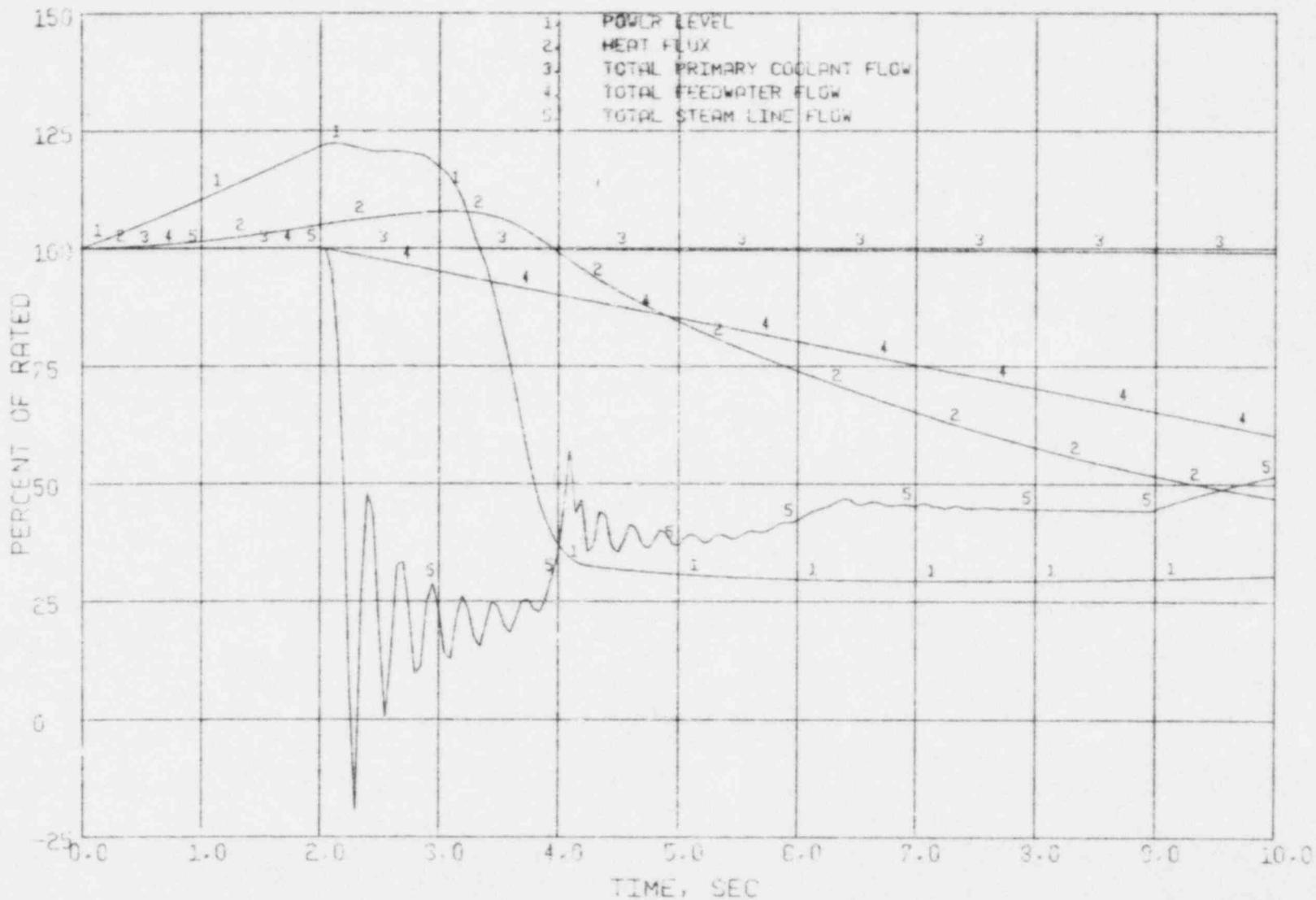
Figure 3.1 Uncontrolled Rod Withdrawal (Fast)
