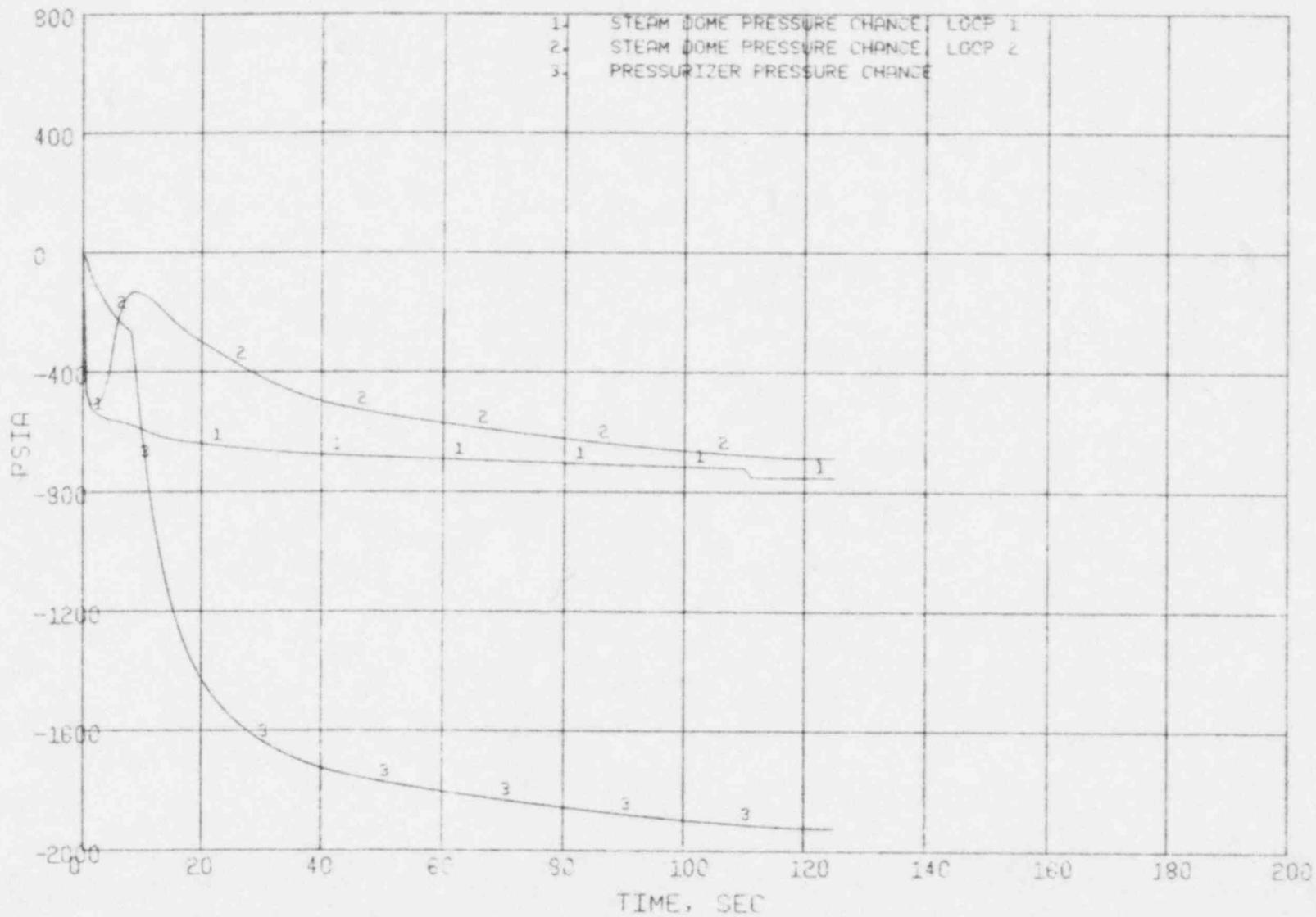
Figure 3.43 Large Steam Line Break (514<sup>0</sup>) - Pressure Changes
