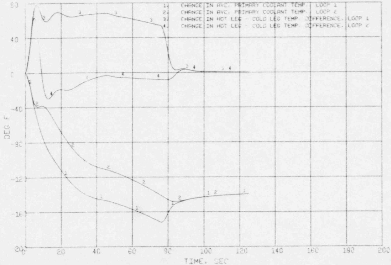
Figure 3.36 Large Steam Line Break (547<sup>D</sup>) - Primary Loop Temperature Changes
