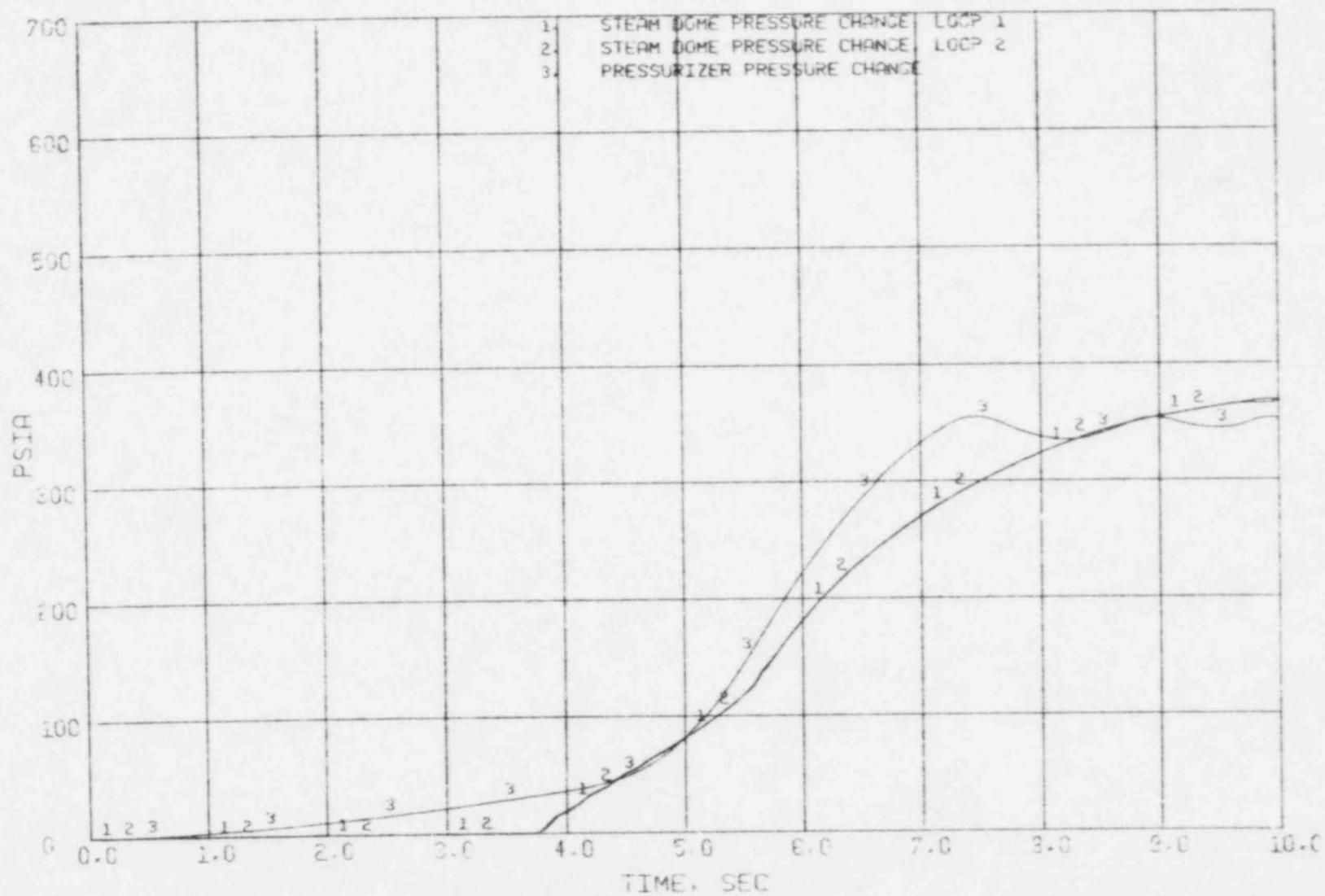
Figure 3.17 Loss of Coolant Flow - Pressure Changes
