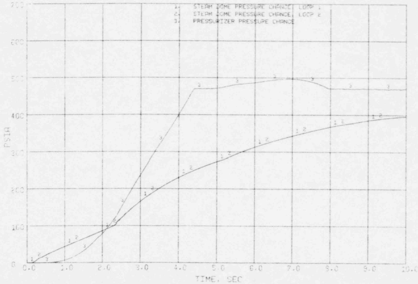
Figure 3.29 Loss of Electric Load - Pressure Changes SEQ REG0565 21/08/82 20.24.59.
