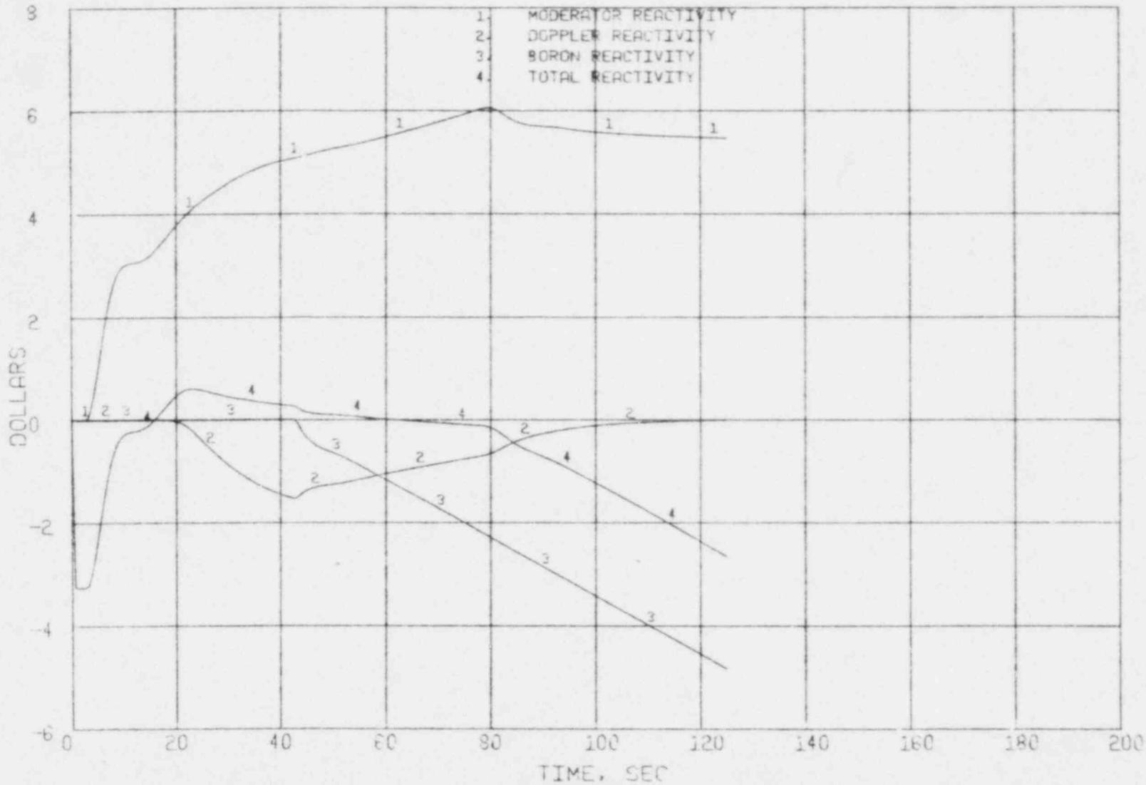
Figure 3.39 Large Steam Line Break (547<sup>0</sup>) - Reactivity
