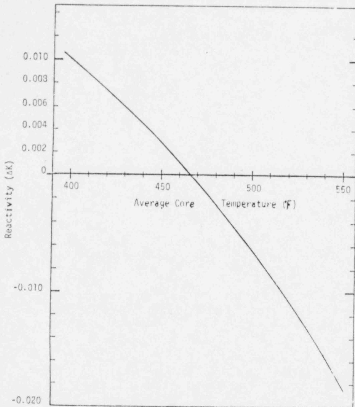
Figure 3.33 Variation of Reactivity with Core Average Temperature at the End of the Cycle
