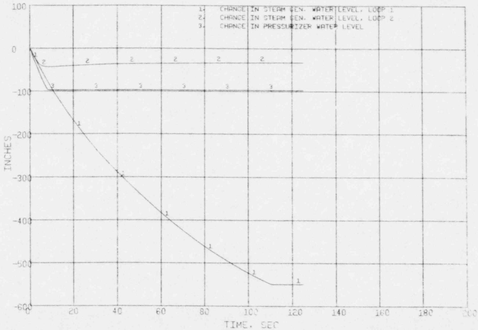
Figure 3.44 Large Steam Line Break (514<sup>0</sup>) - Level Changes
