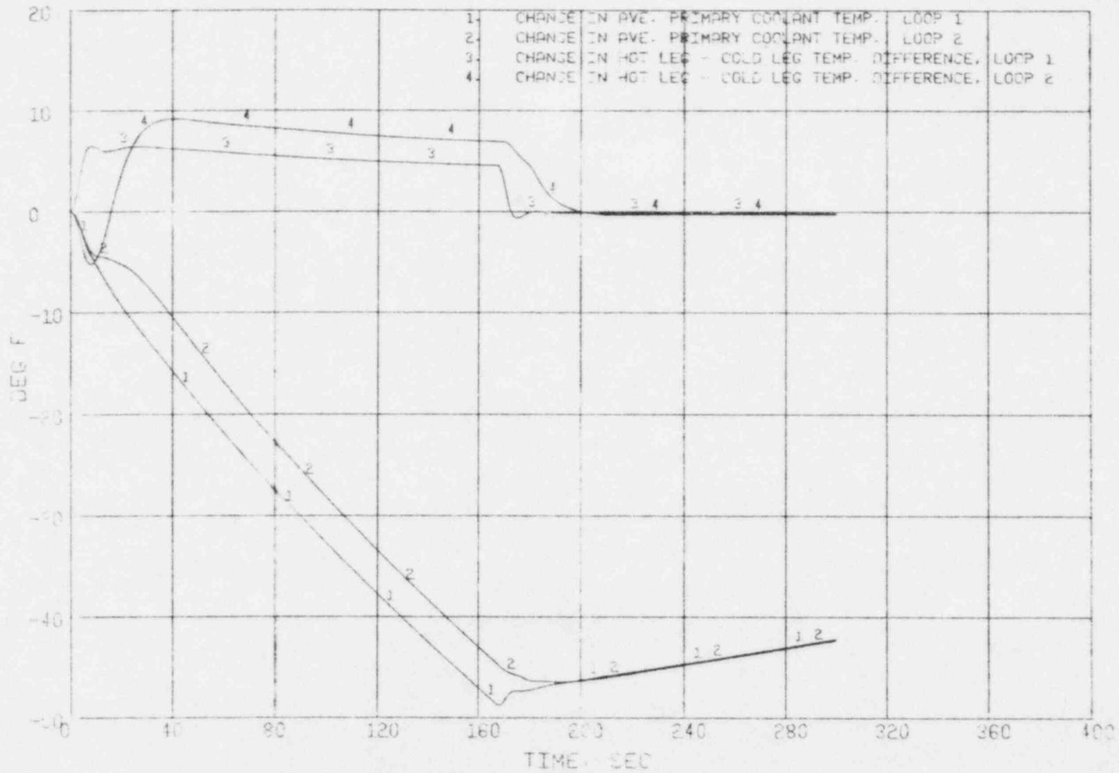
Figure 3.48 Small Steam Line Break (547<sup>0</sup>) - Primary Loop Temperature Changes
