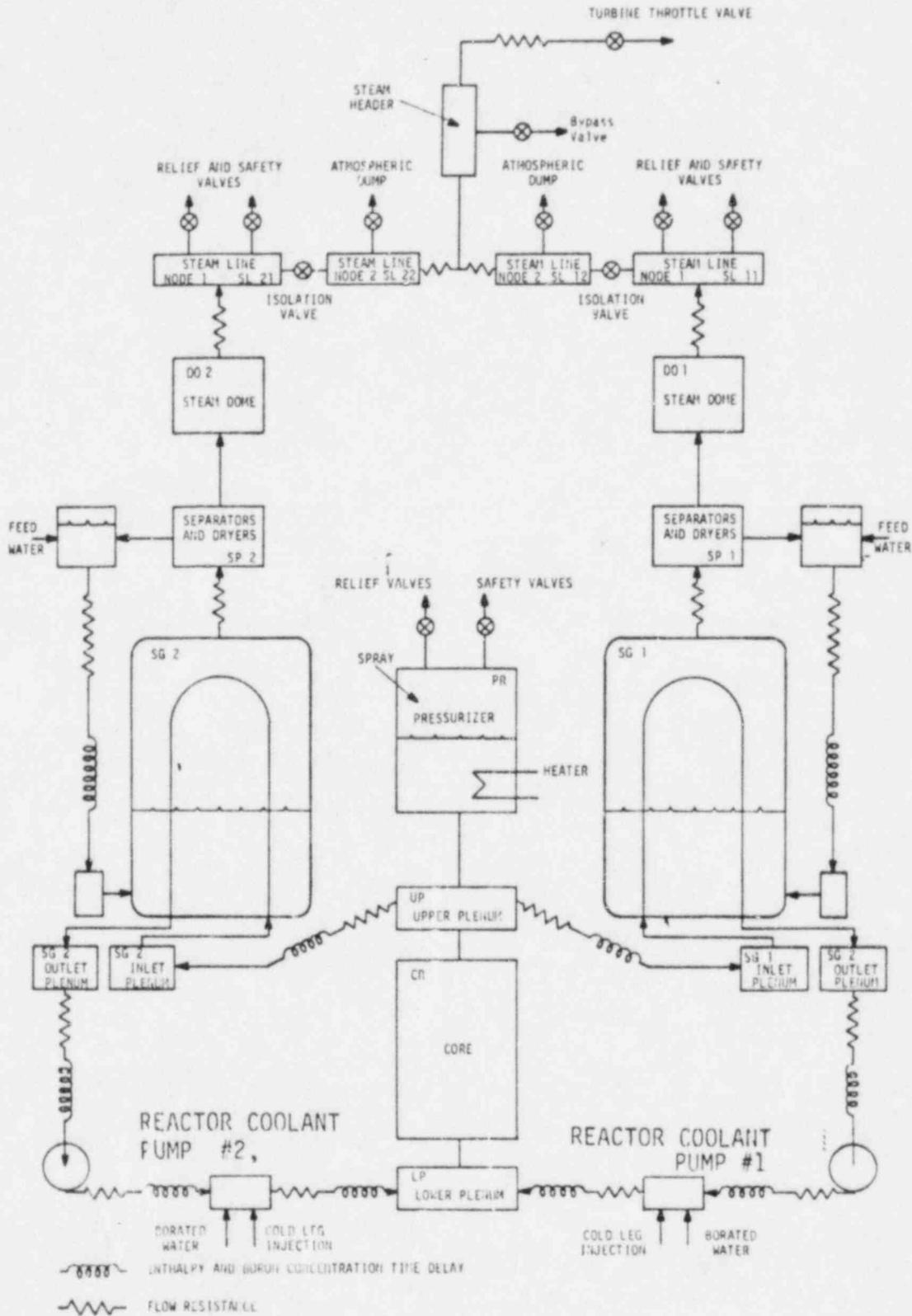
Figure 2.1 PTSPWR2 System Model
