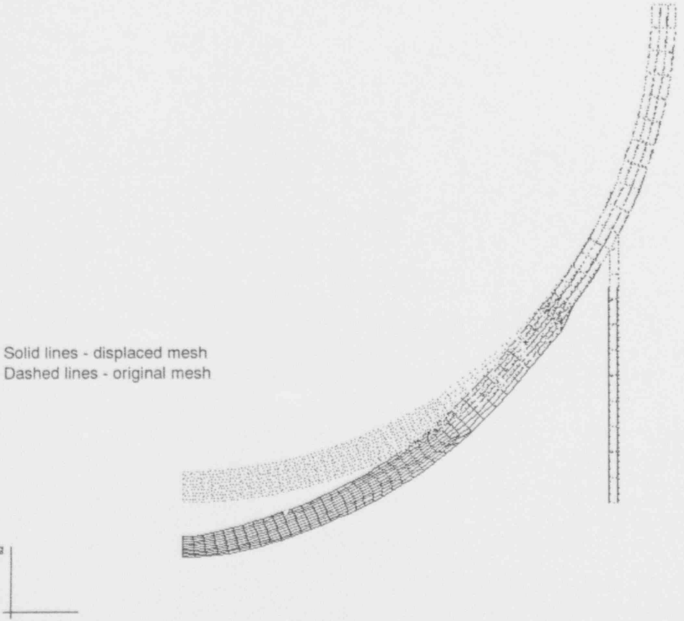
Figure 5-19. Deformed vessel (Ceramic Case II-1).
