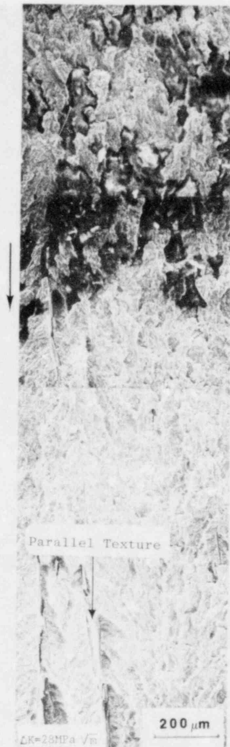
Fig. 7 Fracture surface of A302-B ferritic steel specimen cut along T-L direction (VAB1), tested in air at room temperature with the lower starting \Delta K value. Arrow shows direction of macroscopic crack propagation. Series of SEM micrographs show transition region corresponding to 25-30 \text{MPa}\sqrt{\text{m}} \Delta K value, where inclusion bands begin to appear in fracture surface.
