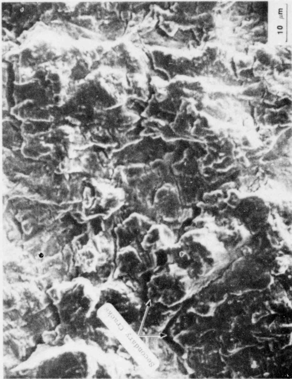
Fig. 8 Fracture surface of A302-B ferritic steel specimen cut along the L-T direction (VADA2), tested in air at room temperature with higher starting K value. Arrow shows direction of macroscopic crack propagation. SEM micrographs illustrate transgranular failure mode with fatigue striations and extensive secondary cracking perpendicular to main crack path. These fractographic features are typical of ferritic steels tested under analogous conditions.
