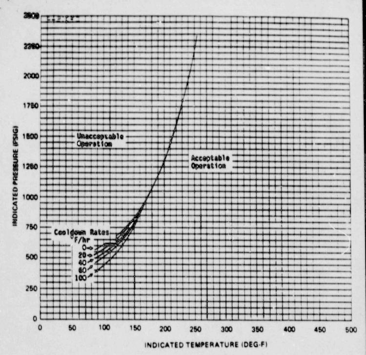
CURVES APPLICABLE FOR COOLDOWN RATES UP TO 180°PF AND FOR THE SERVICE PERIOD UP TO 18 SEPPY AND CONTAINS MARGINS OF 18°P AND 60 POSSIBLE INSTRUMENT SERVICES.
