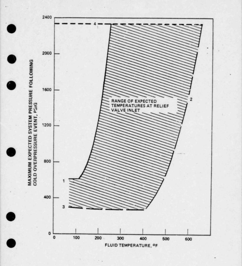
Figure 5-1 (Revised) Potential Cold Overpressure Fluid Conditions at the Relief Valve Inlet
