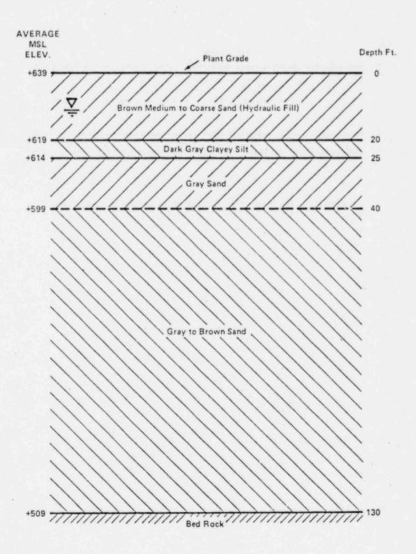
Figure 3 Generalized Soil Profile
