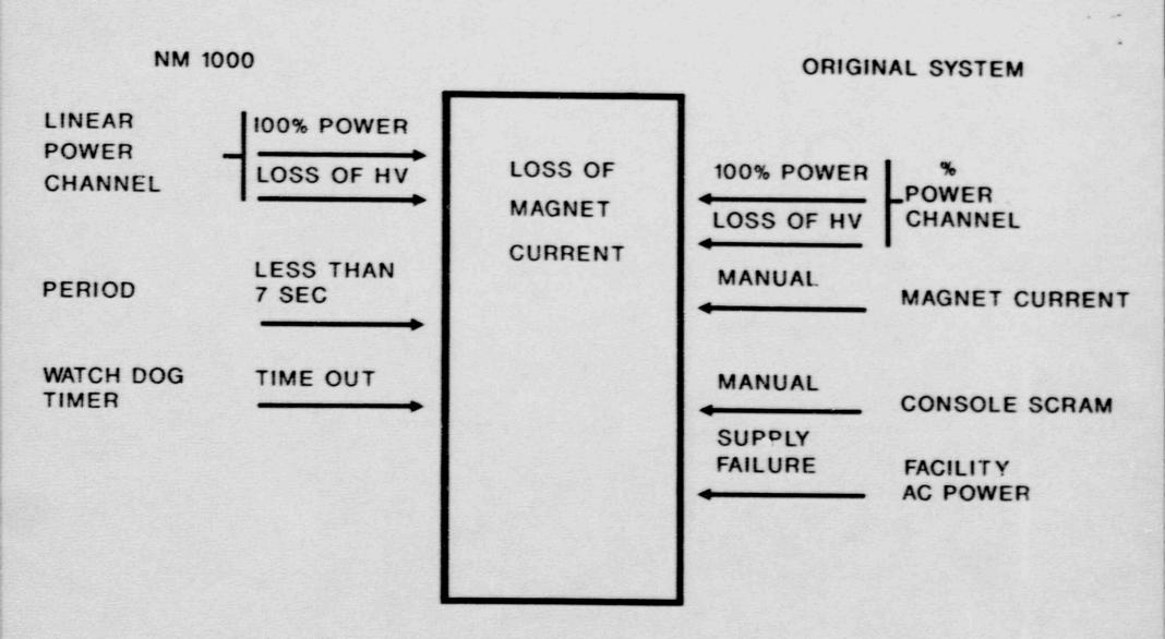
FIG. 7.3 SCHEMATIC REPRESENTATION OF CONDITIONS LEADING TO A SCRAM
