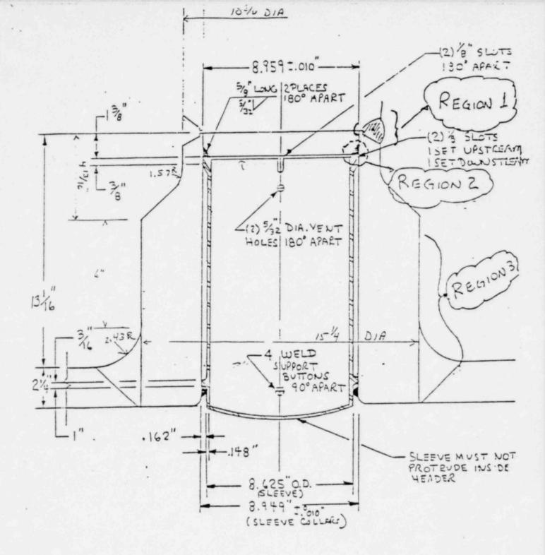
10" THERMAL SLEEVE ON 27 2" HEADER
