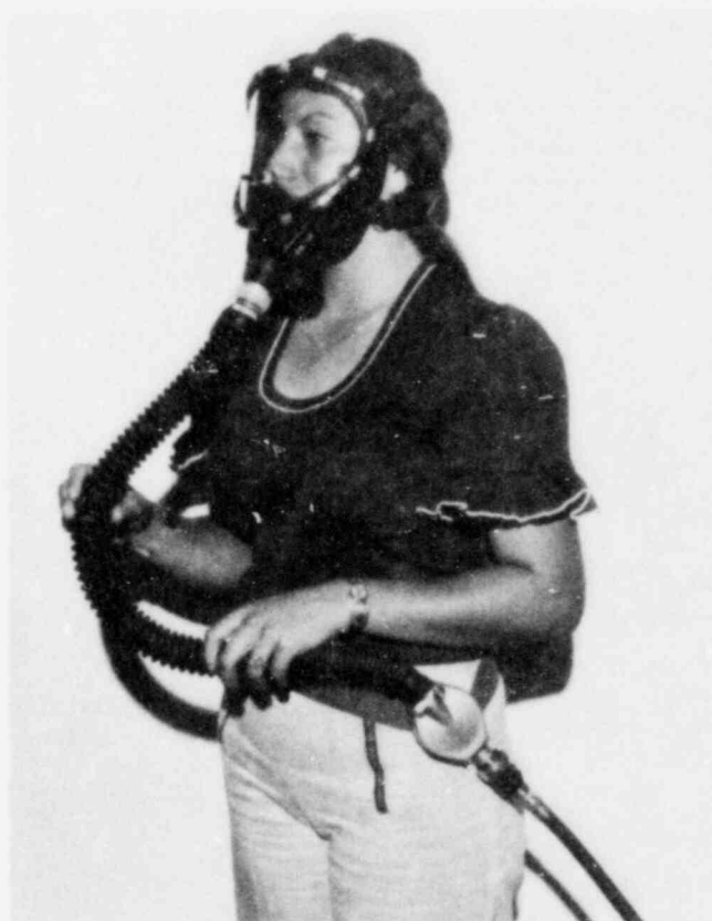
Shown above is a respiratory protective device provided by an airline. This type of device was discussed in an NRC training videotape produced by the Los Alamos National Laboratory. Below is the quantitative fit-testing instrument which gives quantitative estimates of the protection provided by various types of respiratory protective devices and is also used for routine checks of the face-to-facepiece fit of a respirator to a given individual.
