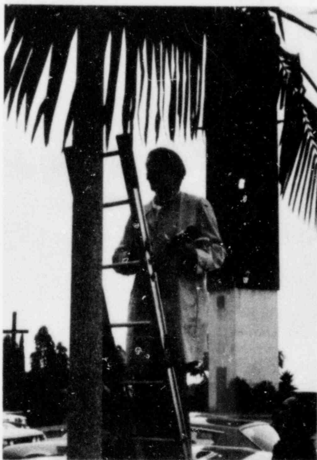
Radiation specialist Thomas Thompson collects a TLD radiation meter and replaces it with another. Thompson is at one of a network of TLD stations around the San Onofre nuclear power plant near San Clemente, Cal.
