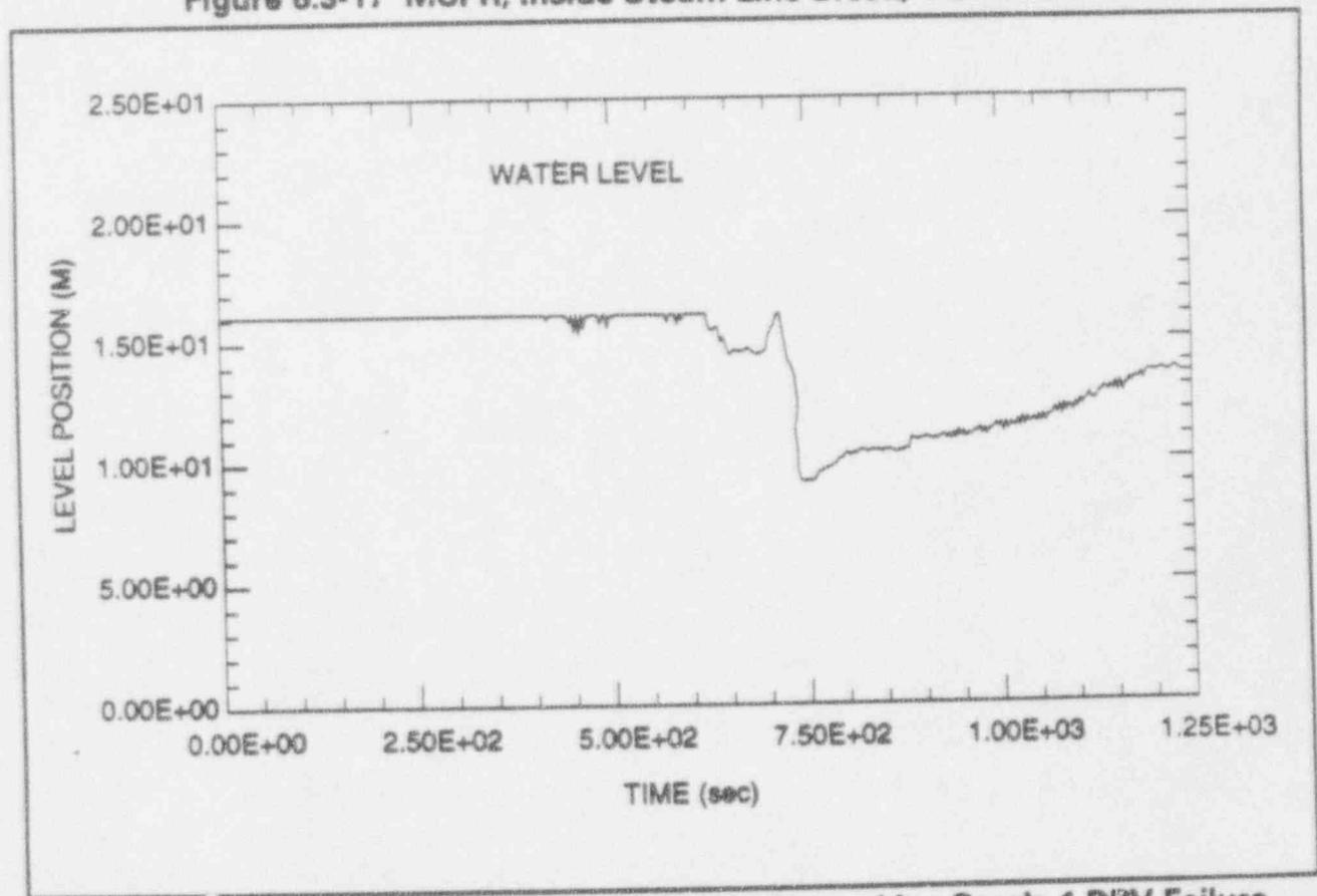
Figure 6.3-18 Chimney Water Level, Inside Steam Line Break, 1 DPV Failure
