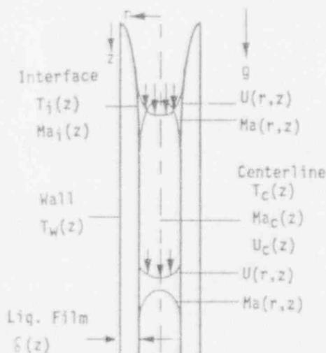
Figure 1 Developing Boundary Layers
