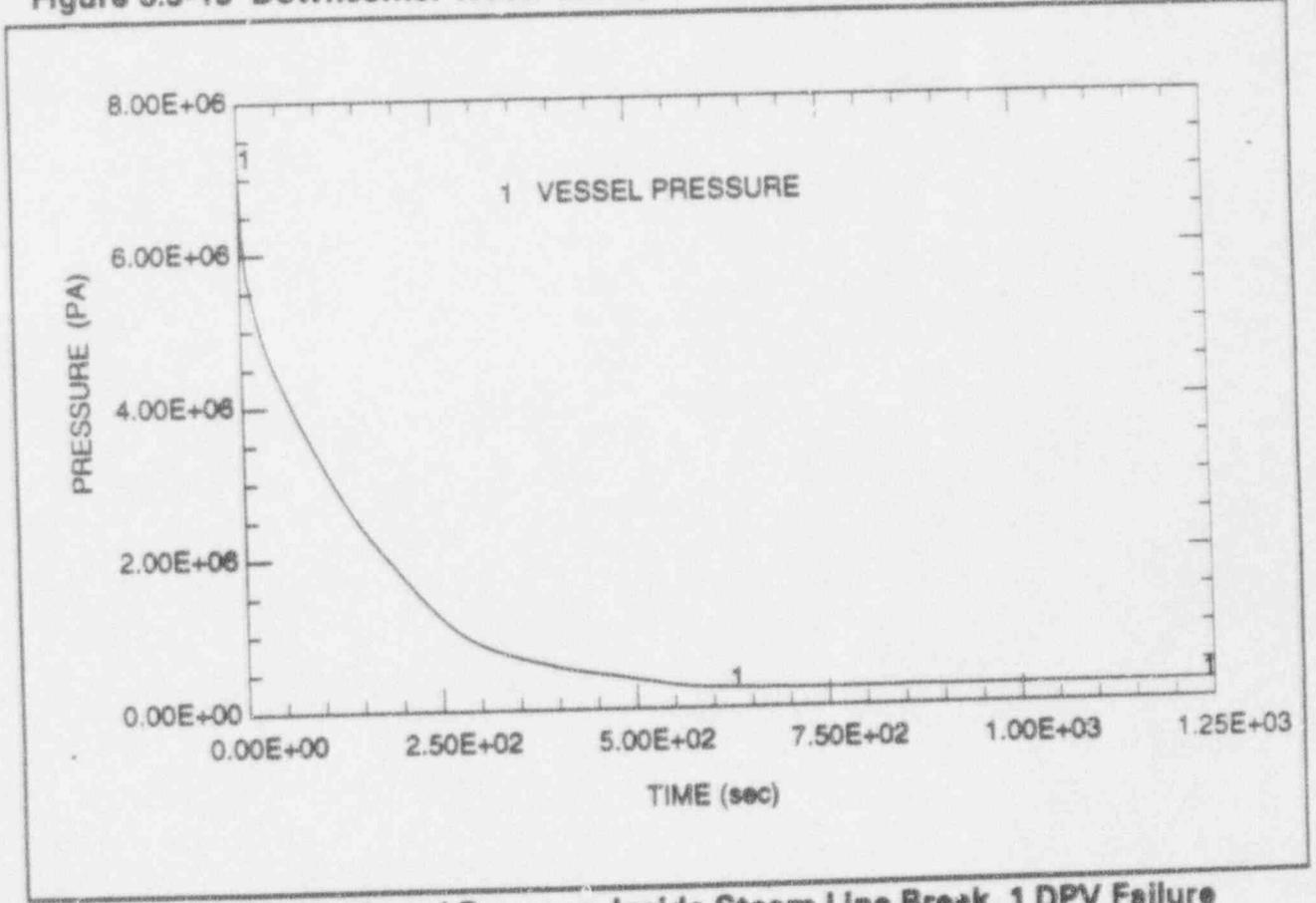
Figure 6.3-20 Vessel Pressure, Inside Steam Line Break, 1 DPV Failure
