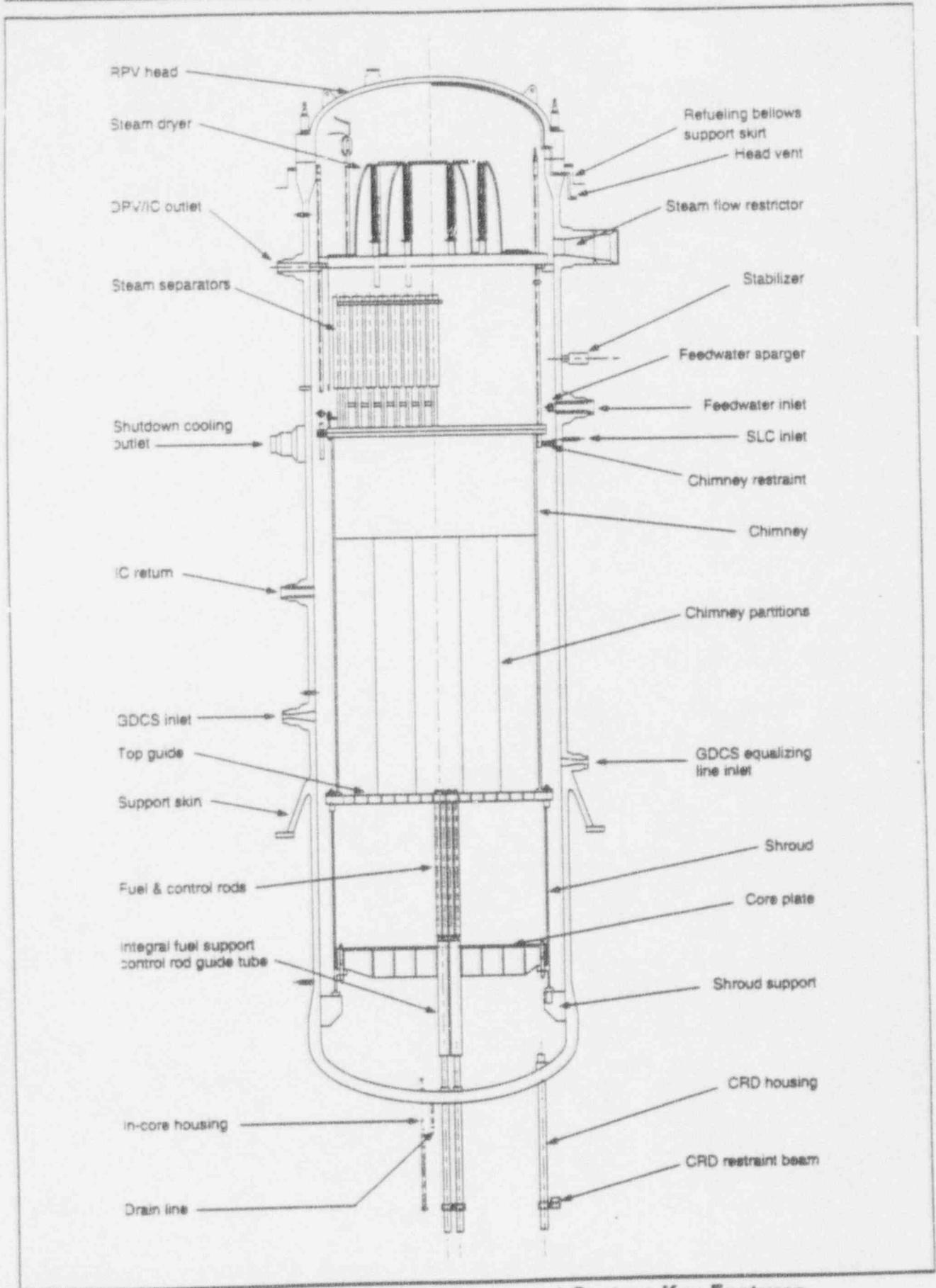
Figure 5.3-3 Reactor Pressure Vessel System Key Features
