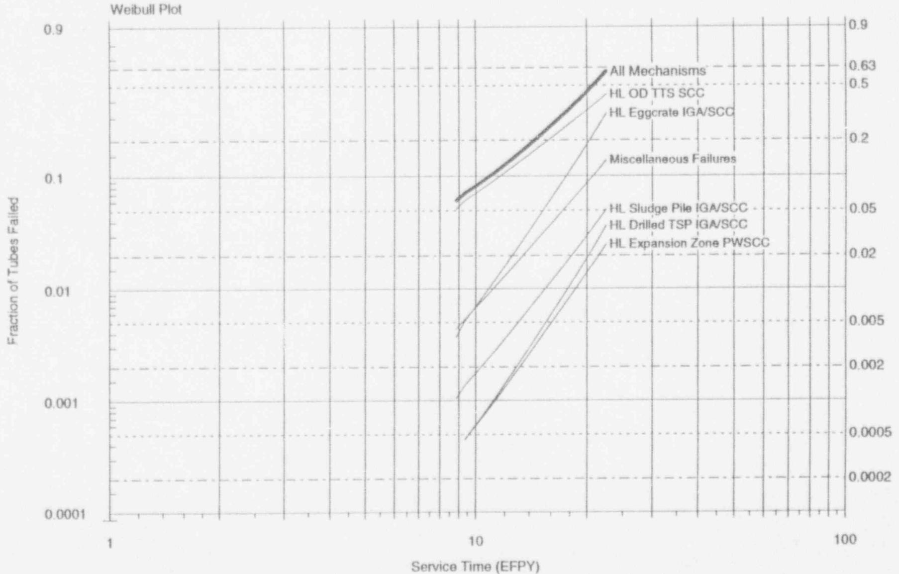
**ANO 2 - SG B - PREDICTED TUBE REPAIRS - PESSIMISTIC ESTIMATE - REDUCED Thot
