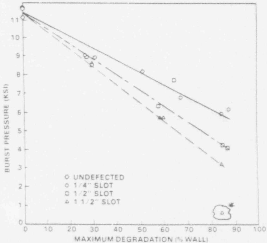
FIGURE 26. Burst Pressures for 0.750 x 0.050 in. EDM Slots
