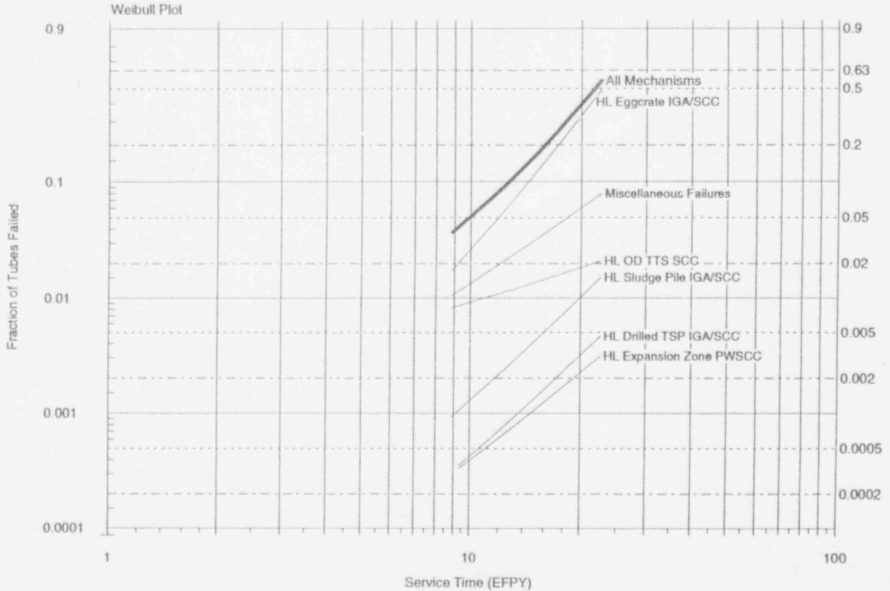
**ANO 2 - SG A - PREDICTED TUBE REPAIRS - OPTIMISTIC ESTIMATE - REDUCED THOT
