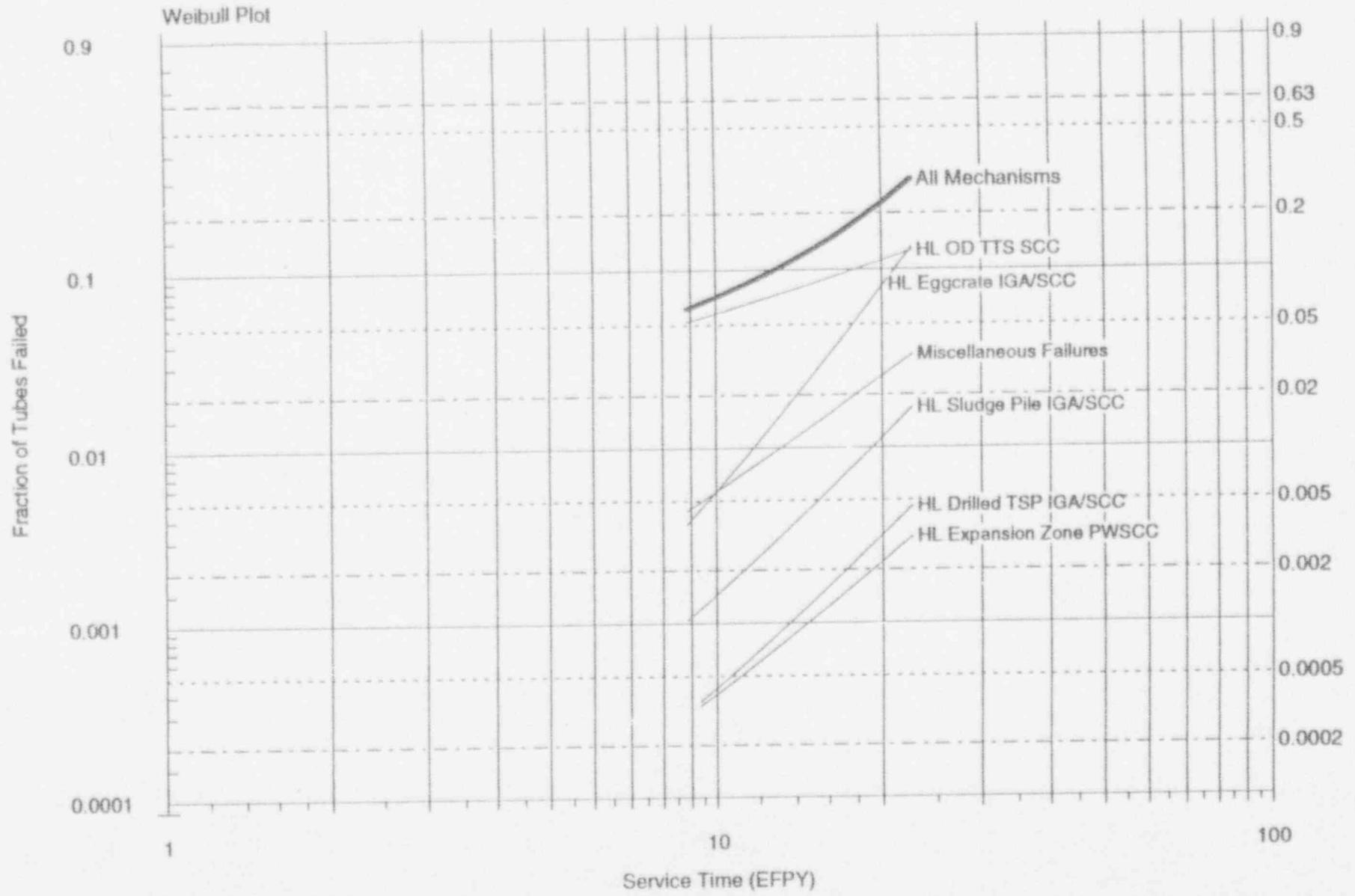
ANO 2 - SG B - PREDICTED TUBE REPAIRS - BEST ESTIMATE - REDUCED Thot (case 1)
