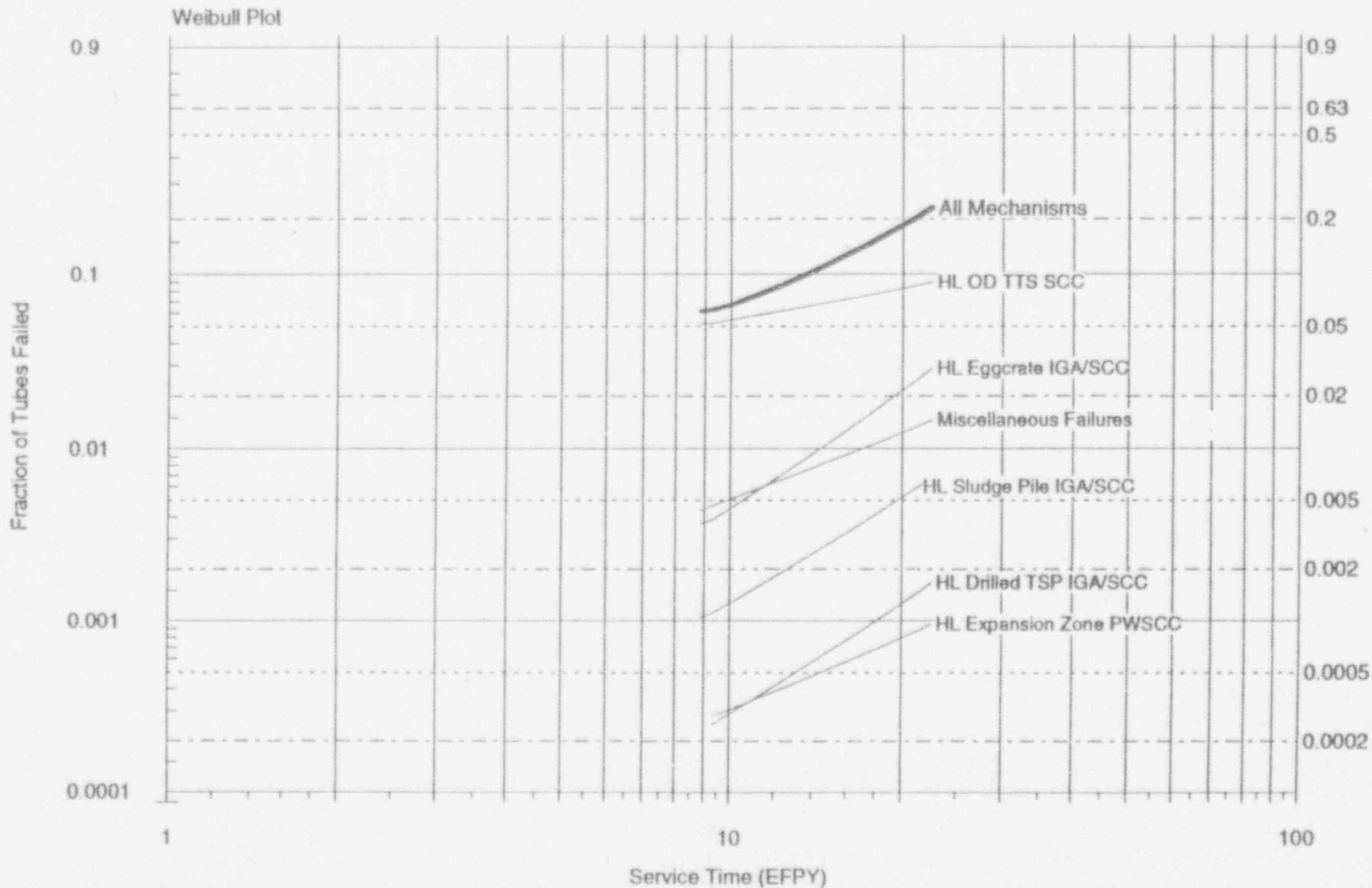
**ANO 2 - SG B - PREDICTED TUBE REPAIRS - OPTIMISTIC ESTIMATE - REDUCED Thor**
