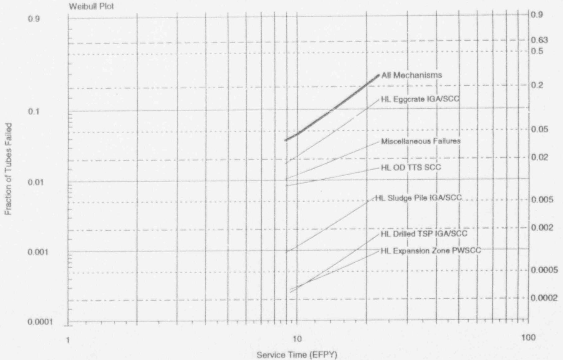
**ANO 2 - SG A - PREDICTED TUBE REPAIRS - PESSIMISTIC ESTIMATE - REDUCED Thot
