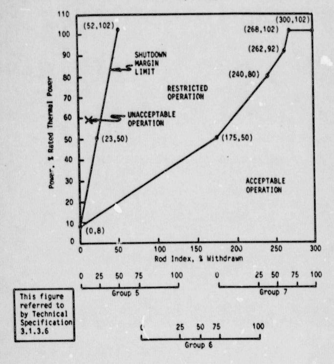
Note 1: A rod group overlap of 25 ± 5% between sequential withdrawn groups 5 and 6, and 6 and 7 shall be maintained.
