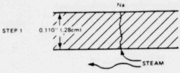
VERY SMALL INITIAL H<sub>2</sub>O LEAK FLOW
