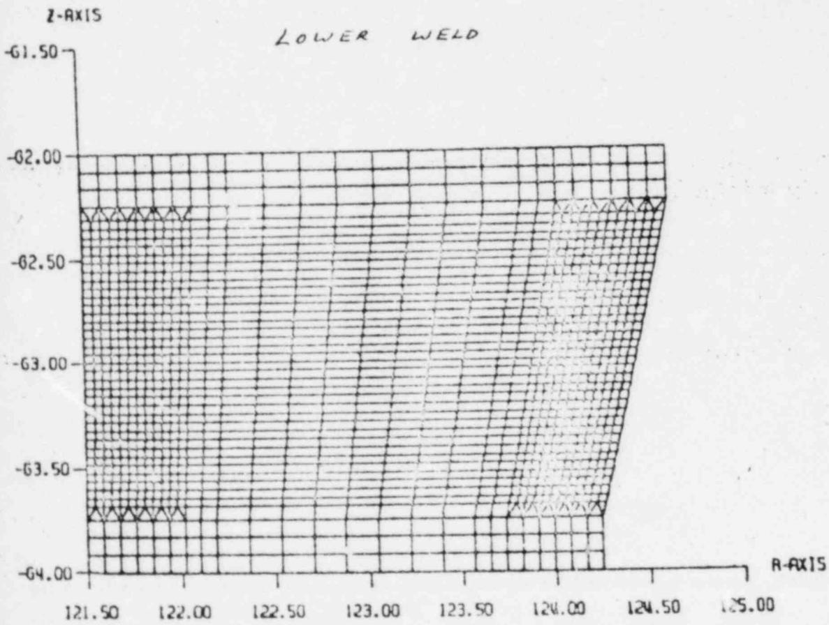
CIC VESSEL FLANGE CONVERGENCE STUDY AT DISSIMILAR WELD-DRD REFINEMENT
