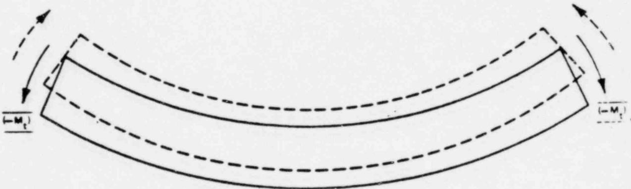
FINAL DEFORMED SHAPE AFTER LOAD REMOVAL
