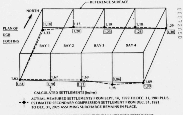
COMPARISON OF 40-YEAR ESTIMATED SETTLEMENT VALUES WITH SETTLEMENT VALUES RESULTING FROM A FINITE ELEMENT ANALYSIS OF THE ZERO SPRING CONDITION
