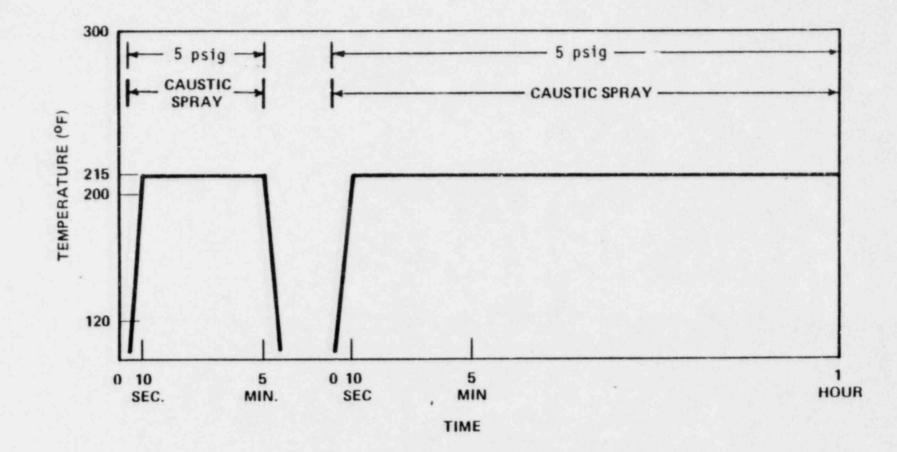
Figure 4. High Energy Line Break (HELB) Test Profile
