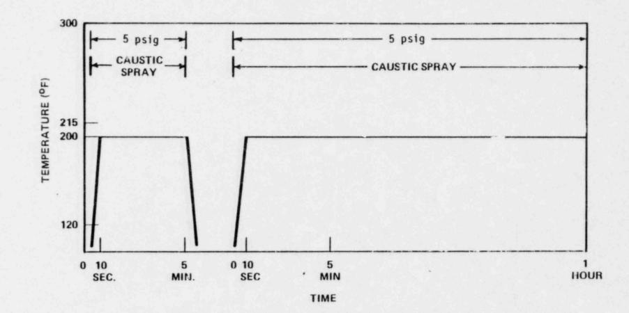
Figure 3. High Energy Line Break (HELB) Environmental Requirement
