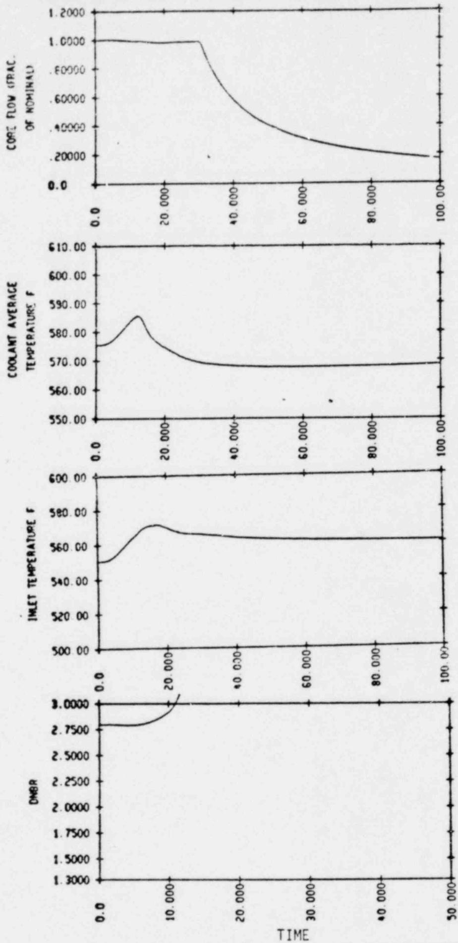
LOSS OF LOAD FROM 70 PERCENT POWER WITHOUT PRESSURE CONTROL
