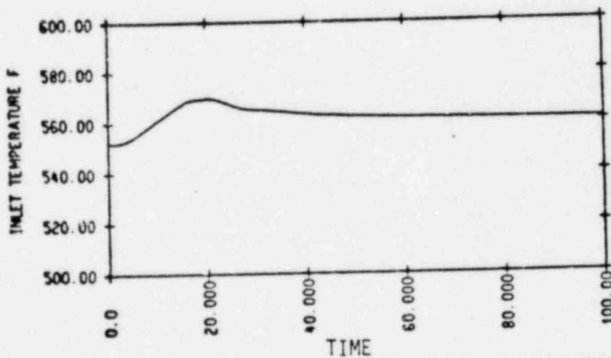
LOSS OF LOAD WITHOUT PRESSURE CONTROL, MINIMUM FEEDBACK
