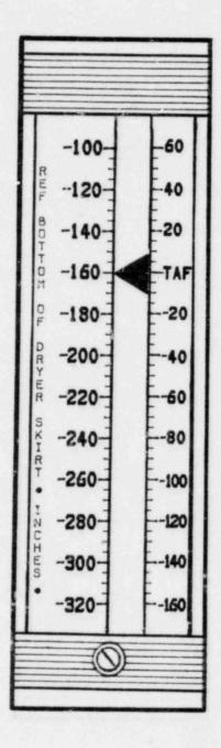
Main Control Room Fuel Zone Water Level Indicator Life-Size Dual Scales Mounted on GE Type 180 Instrument
