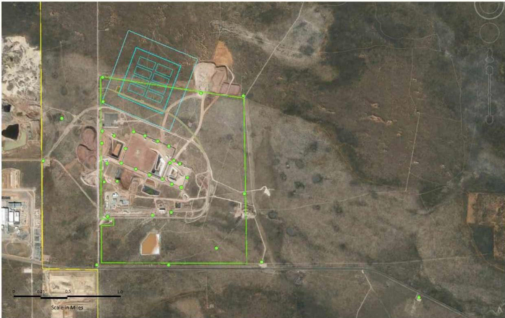
Figure 4.12-10 On-site Thermoluminescent dosimeters (TLDs) or Optically Stimulated Luminescent dosimeters (OSLs) monitoring locations (36 locations in 2014).
