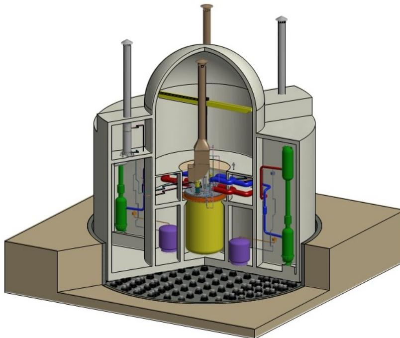
**Figure 2-4 – Illustration of SFR Reactor Building [20]**
