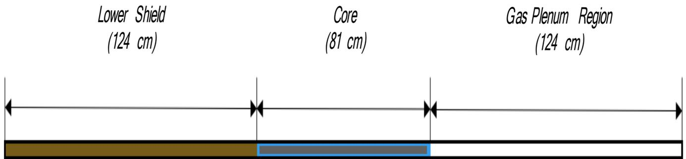
**Figure 4-10 – Illustration of SFR Reactor Fuel Pin [17]**
