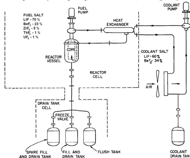
**Figure 2-5: MSRE Plant Layout [23, p. 6]**
