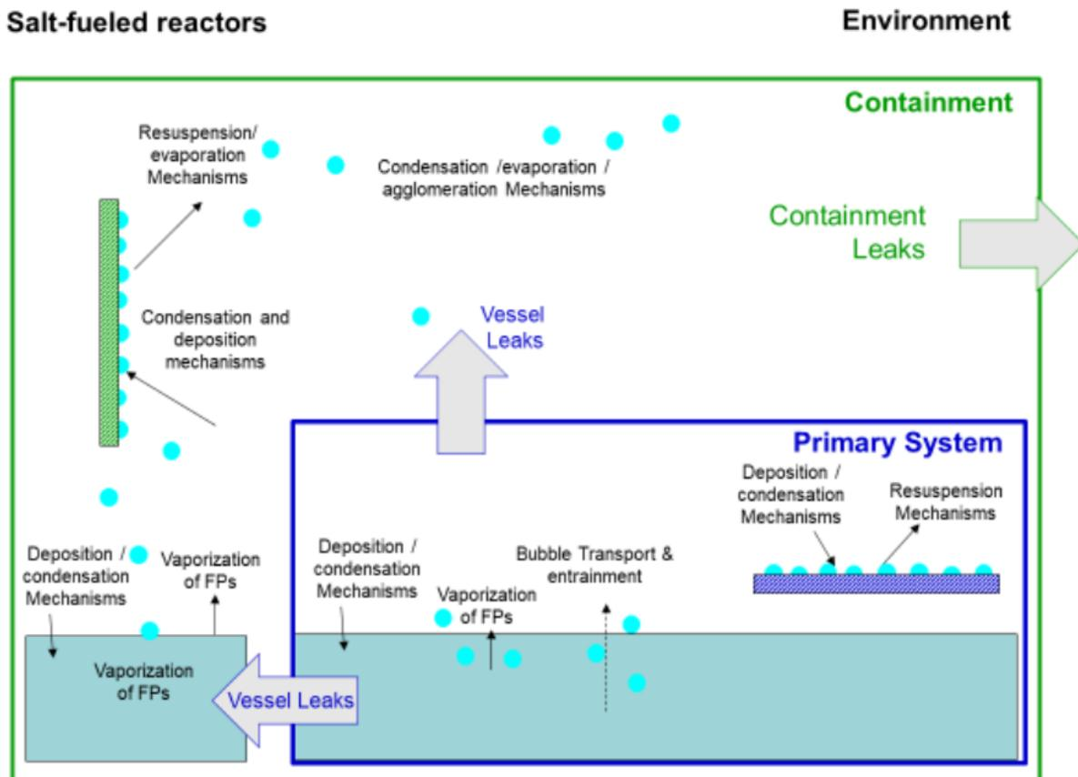
Figure 4-14 – Summary of Radionuclide Release and Transport Processes for Molten Salt Reactors [22]
