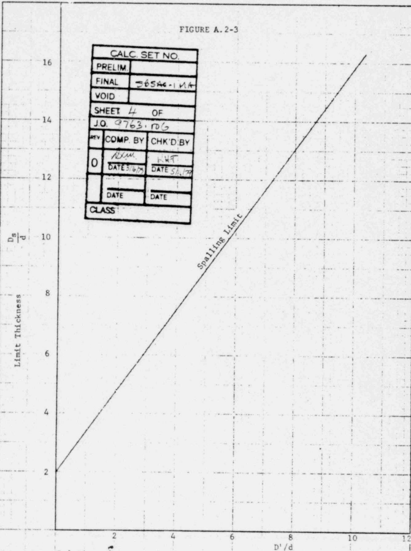
Relation of penetration to scabbing limit thickness.
