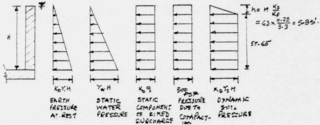
LATERAL PRESSURE COMPONENTS AT THE BASE OF WALL:EARTH PRESSURE AT REST
