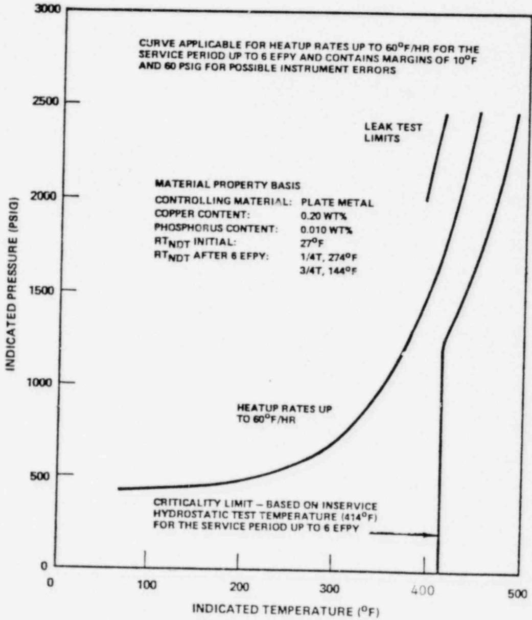
Figure 3.4-2 Beaver Valley Unit No. 1 Reactor Coolant System Heatup Limitations Applicable for the First 6 EPY
