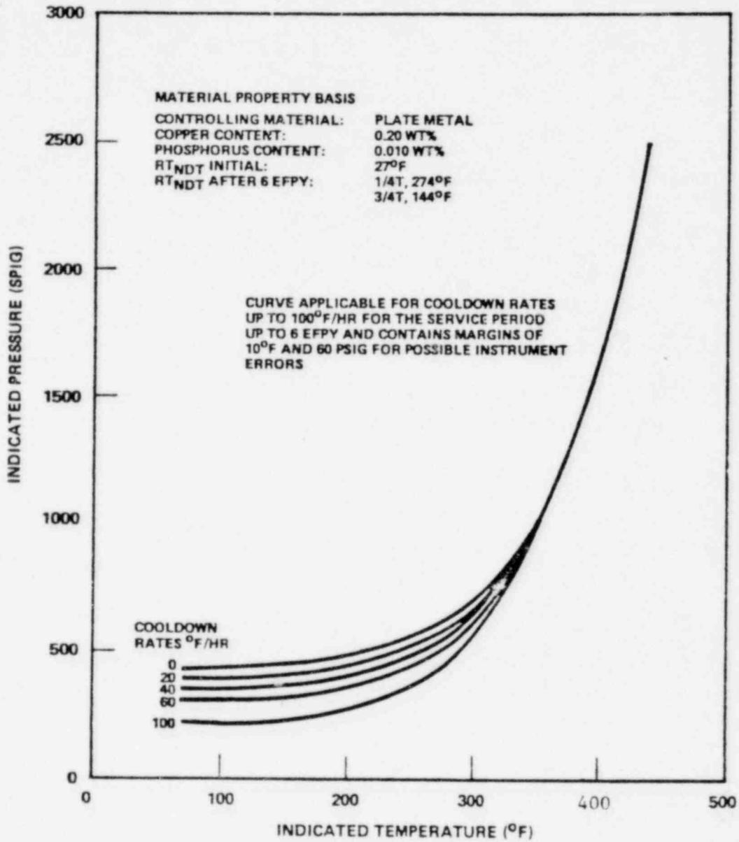
Figure 3.4-3 Beaver Valley Unit No. 1 Reactor Coolant System Cooldown Limitations Applicable for the First 6 EPFY
