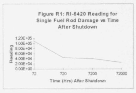
2E4 CPM corresponds to the minimum expected response and is significantly higher than the alarm setpoint of 600 CPM.
