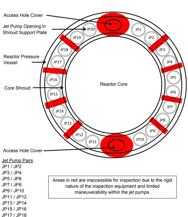
Attachment D – Monticello Shroud Support Plate Underside Illustration (Shroud Support Legs Not Illustrated) Attachment E - Tooling Insertion Paths
