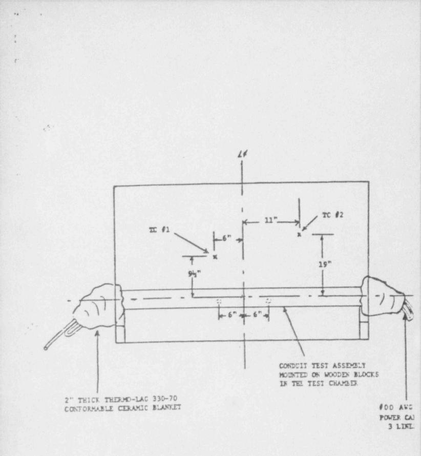
FIGURE 2.1 LOCATION OF TEST ASSEMBLY AND AMBIENT TEMPERATURE THERMOCOUPLES IN TEST CHAMBER
