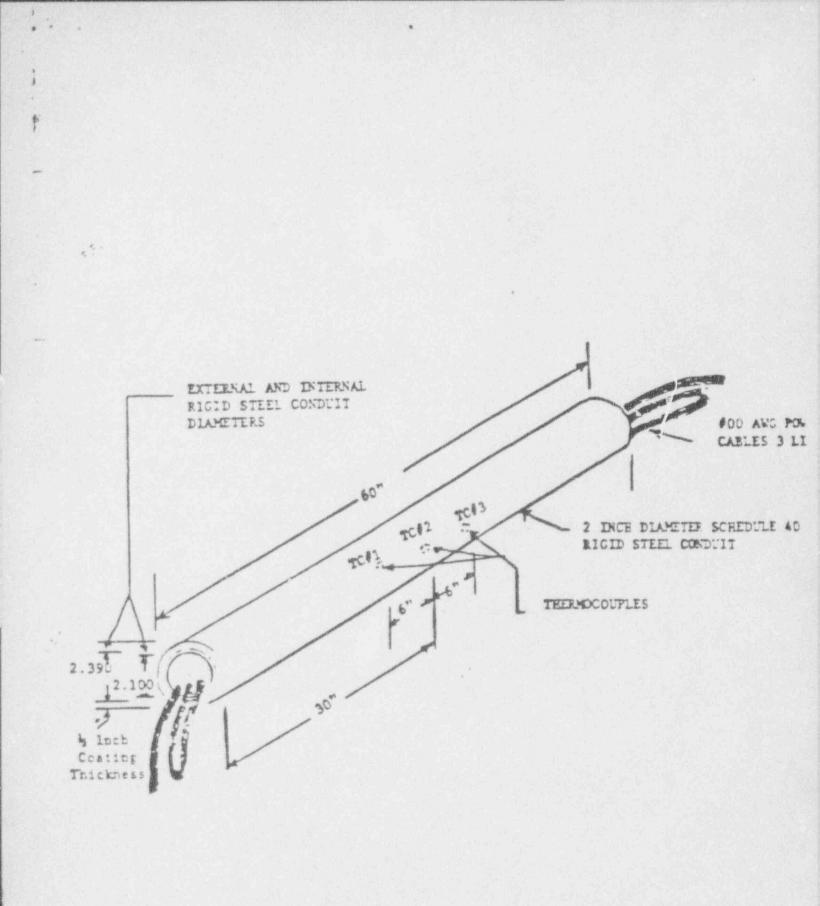
FIGURE 2.3 LOCATION OF THERMOCOUPLES WITHIN THE TEST ASSEMBLY
