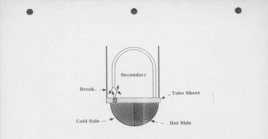
Schematic Description of A Steam Generator Tube Rupture
