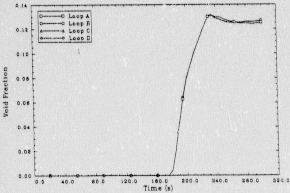
Figure 25. Scenario 3: loop reactor coolant pump vapor void fractions.
