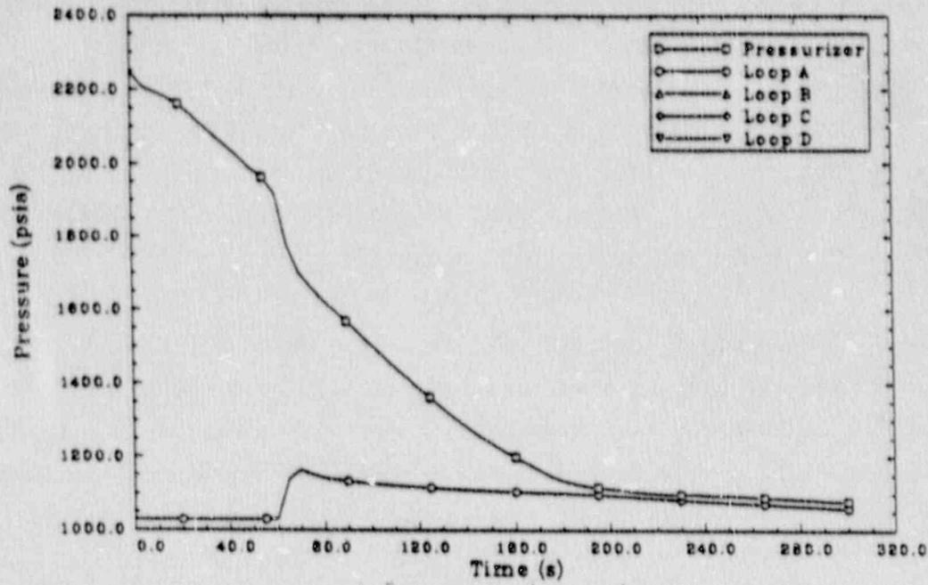
Figure 20. Scenario 3: primary and secondary pressures.
