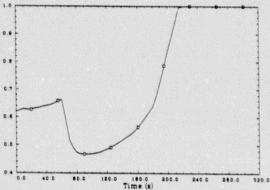
Figure 21. Scenario 3: pressurizer level.
