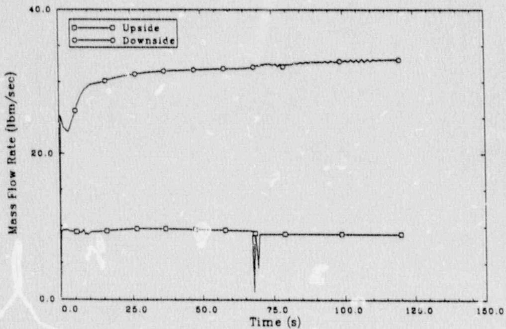
Figure 35. Scenario 4: steam generator tube rupture mass flow rates.
