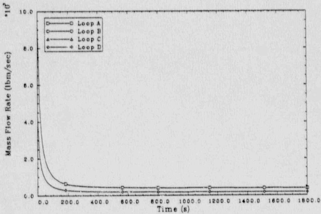
Figure 10. Scenario 1: primary hot leg mass flow rates.
