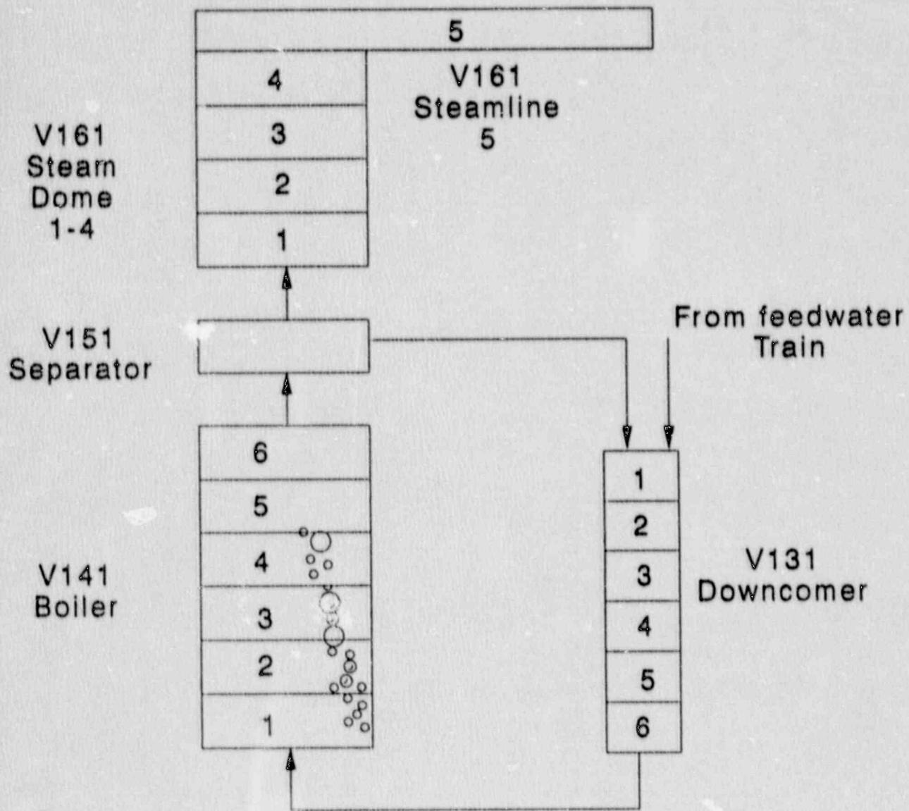
Figure 3. Nodalization of the SNUPPS Model F Steam Generator (Loop A shown).
