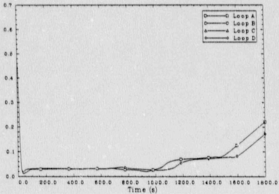
Figure 19. Scenario 2: steam generator narrow range levels.
