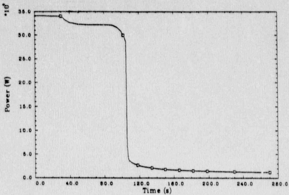
Figure 46. Scenario 5: reactor power.
