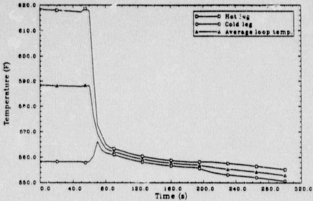
Figure 22. Scenario 3: primary hot, cold and loop average temperatures.
