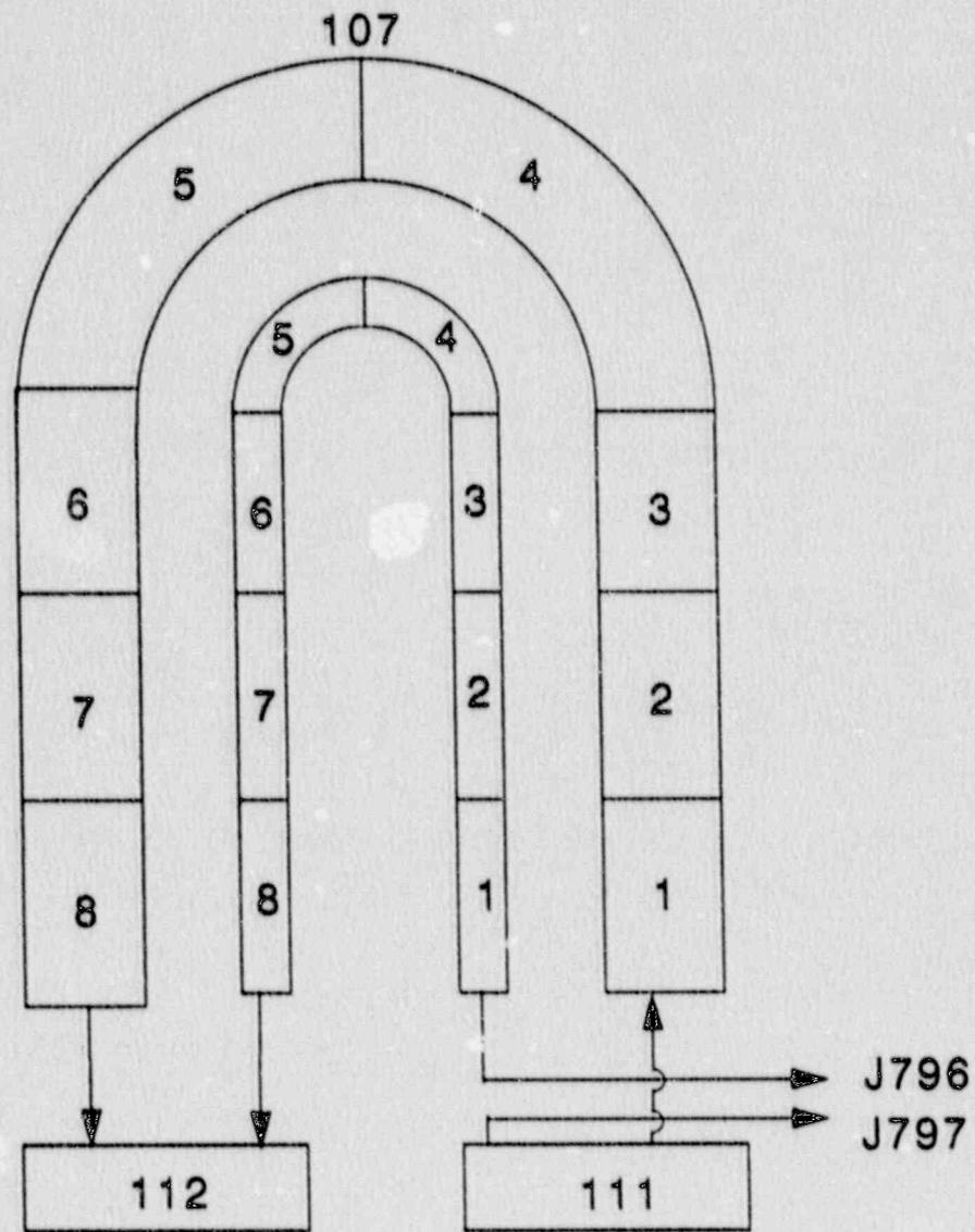
Figure 29. Scenario 4: nodalization changes for loop A steam generator tube rupture.
