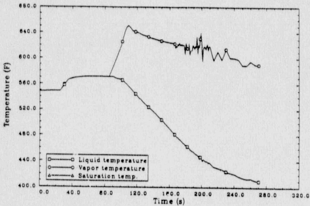
Figure 49. Scenario 5: loop A steam generator boiler region liquid, vapor, and saturation temperatures.
