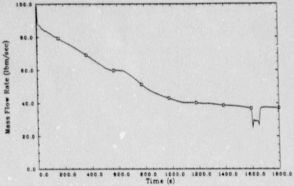
Figure 18. Scenario 2: loop D cold leg break mass flow rate.
