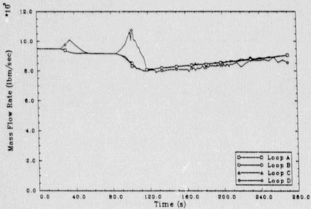
Figure 45. Scenario 5: primary leg mass flow rates.
