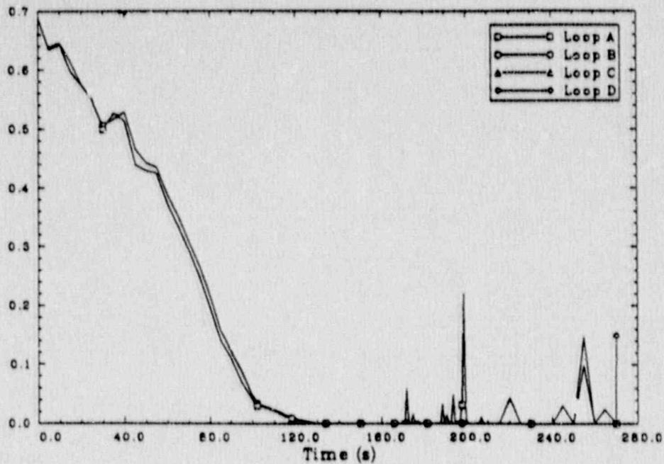
Figure 48. Scenario 5: steam generator wide range levels.
