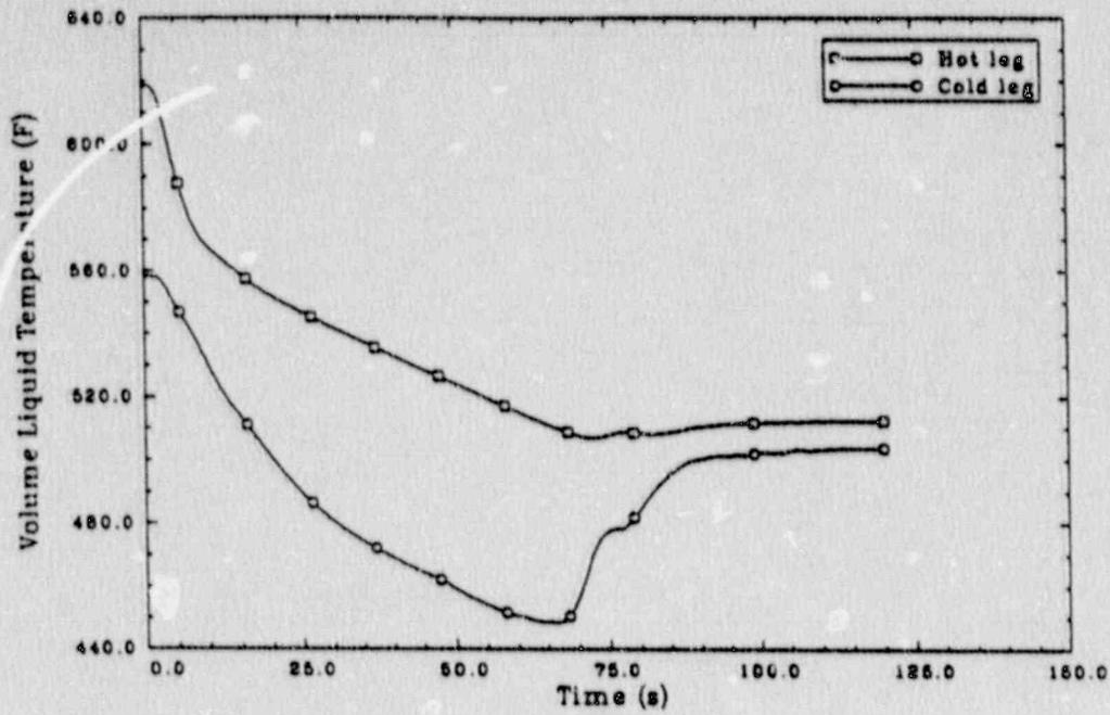
Figure 38. Scenario 4: loop A hot and cold leg temperatures.
