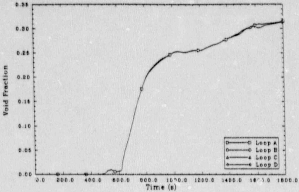
Figure 16. Scenario 2: primary hot leg void fractions.
