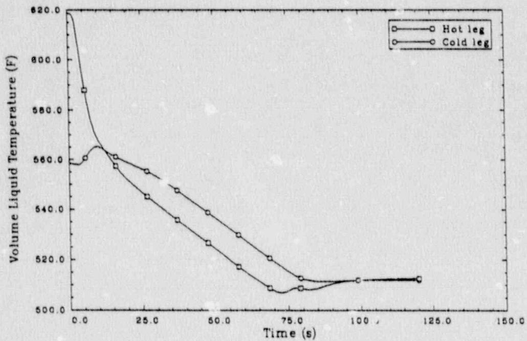
Figure 41. Scenario 4: loop D hot and cold leg temperatures.
