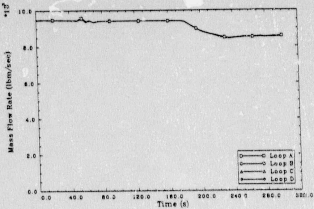
Figure 24. Scenario 3: primary cold leg mass flow rates.
