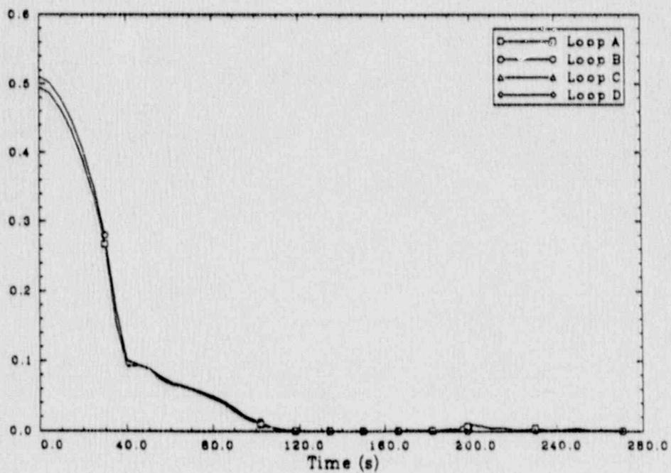
Figure 47. Scenario 5: steam generator narrow range levels.
