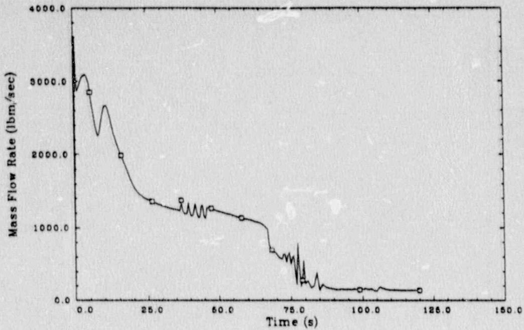
Figure 34. Scenario 4: steam line break mass flow rate.
