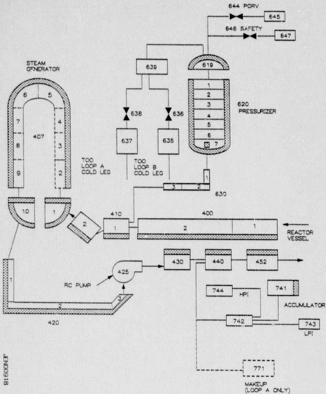
Figure 1. Nodalization of the SNUPPS primary coolant loops (Loop D shown).
