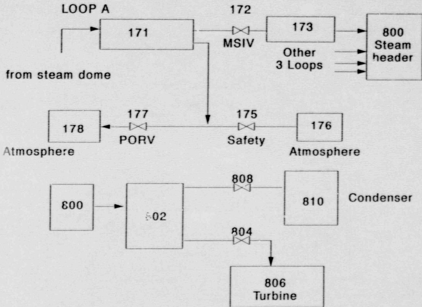
Figure 4. Nodalization of the SNUPPS Steam Line (Loop A shown).
