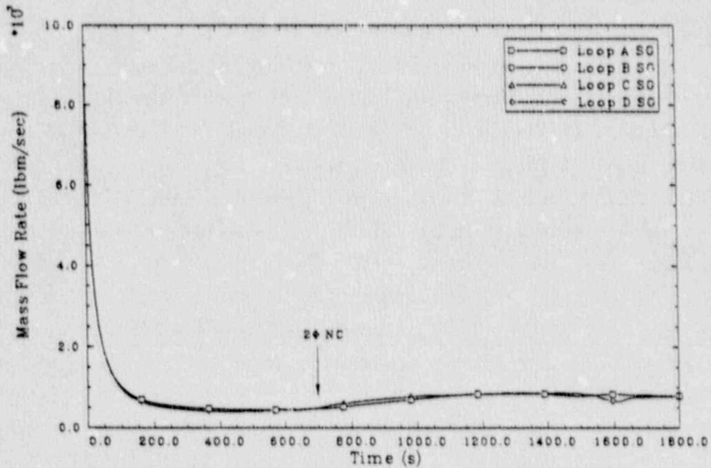
Figure 13. Scenario 2: primary hot leg mass flow rates.
