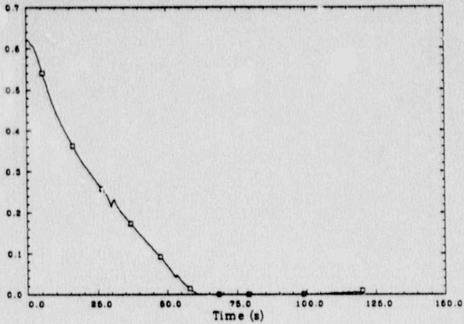
Figure 36. Scenario 4: pressurizer level.
