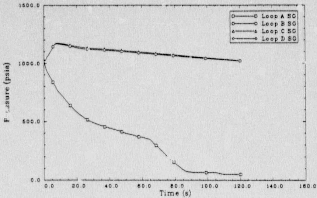
Figure 30. Scenario 4: steam generator pressures.
