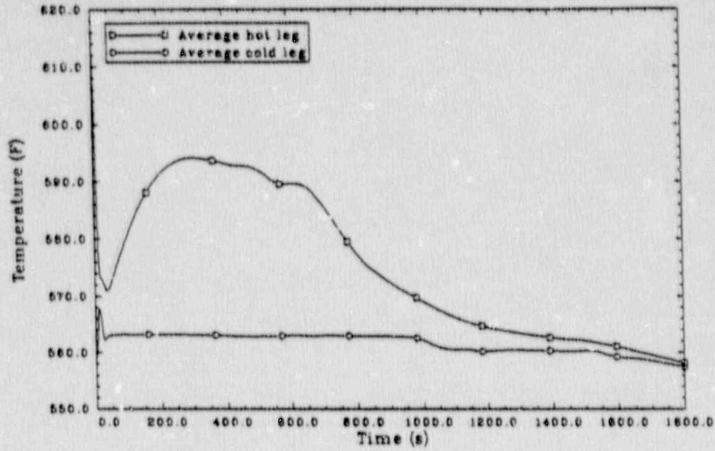
Figure 14. Scenario 2: average primary hot and cold leg temperatures.
