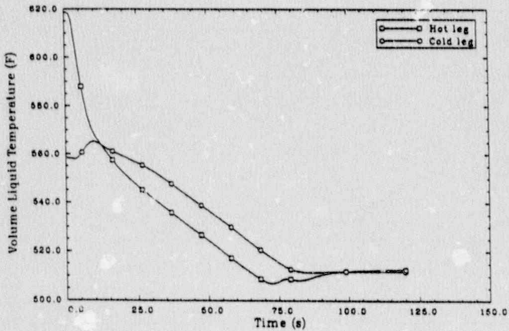
Figure 39. Scenario 4: loop B hot and cold leg temperatures.
