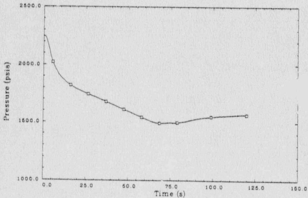
Figure 31. Scenario 4: pressurizer pressure.
