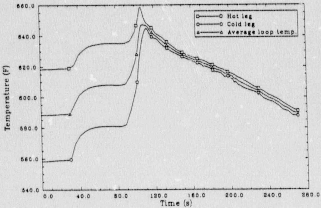
Figure 43. Scenario 5: primary loop hot, cold, and average temperatures.
