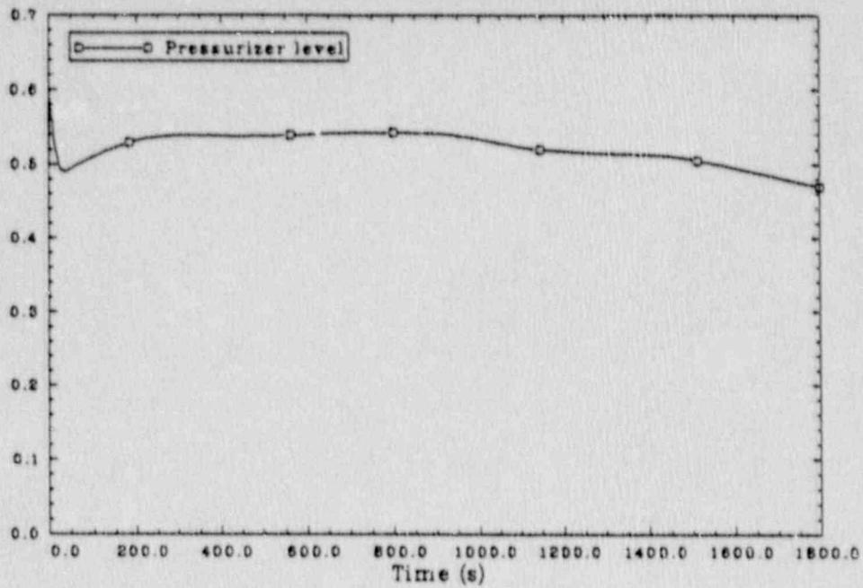
Figure 9. Scenario 1: pressurizer level.
