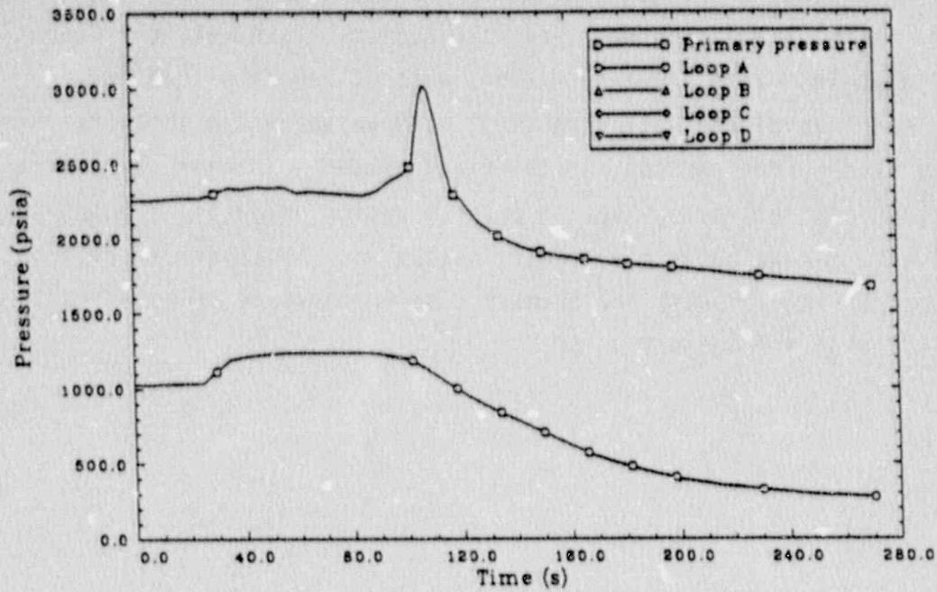
Figure 42. Scenario 5: primary and secondary pressures.
