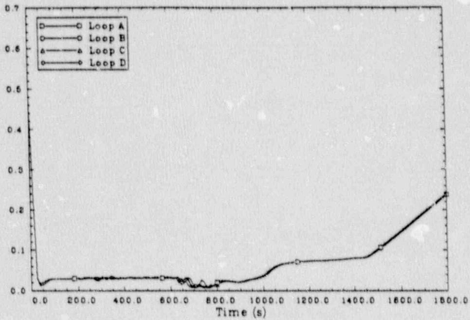
Figure 11. Scenario 1: steam generator narrow range levels.
