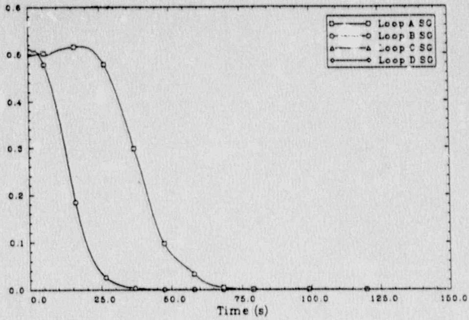
Figure 32. Scenario 4: steam generator narrow range levels.
