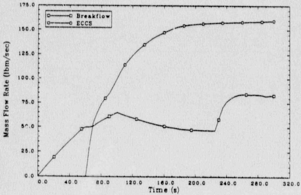
Figure 23. Scenario 3: break and total ECCS mass flow rates.
