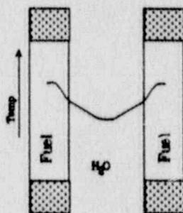
Figure A-3. Temperature variation within a cooling channel.
