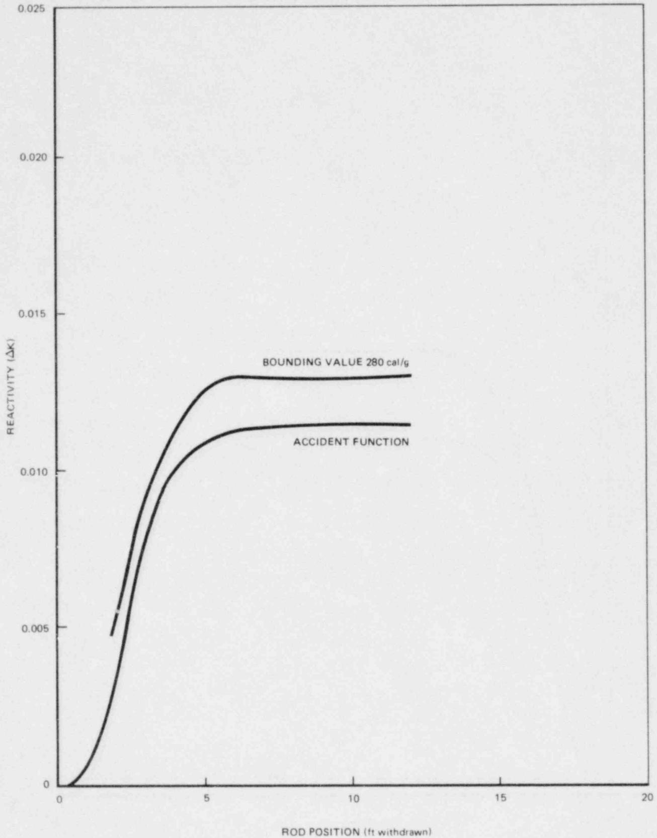
Figure 11. RDA Reactivity Shape Function, Hot Standby
