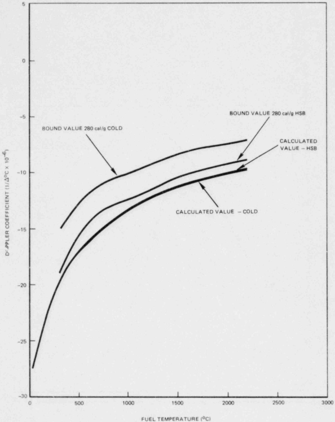
Figure 9. Doppler Reactivity Coefficient Comparison for RDA Y1003J01A34
