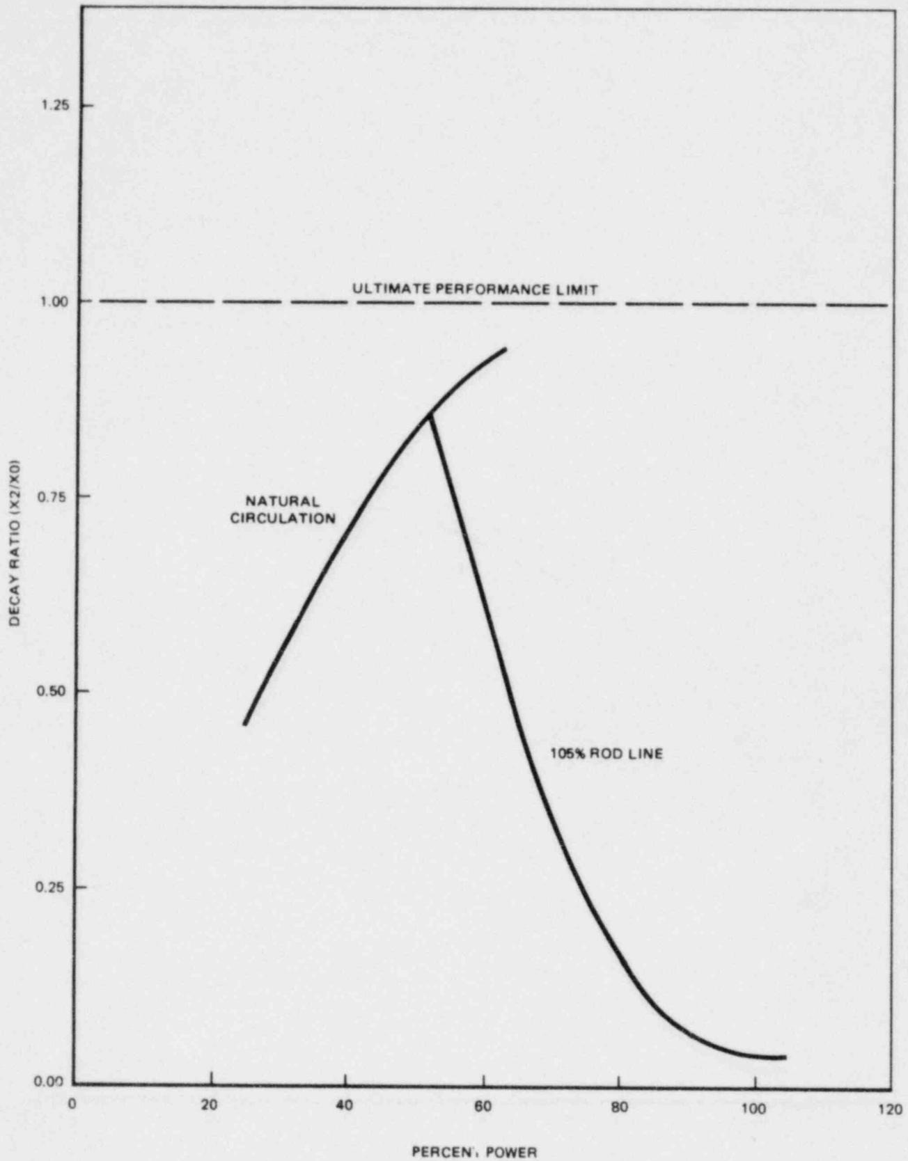
Figure 8. Reactor Core Decay Ratio versus Power
