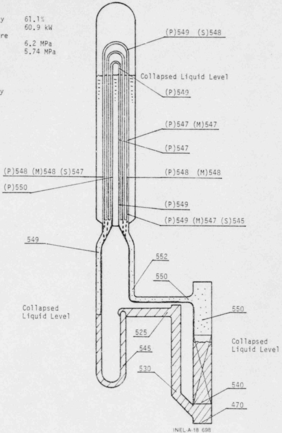
Figure 9. Fluid temperature and mass distribution in the system during reflux natural circulation.
