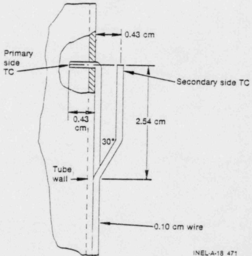
Figure 4. Intact loop steam generator fluid thermocouple installation.
