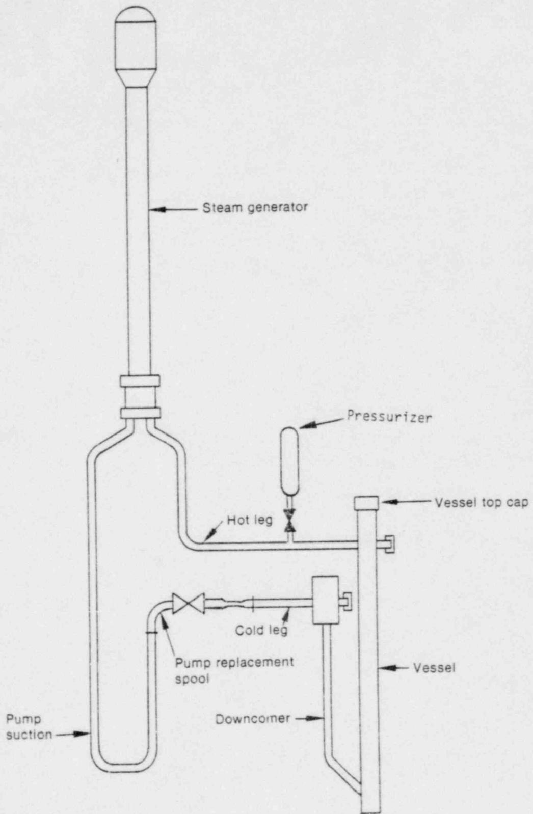
Figure 1. System configuration for Test S-NC-4.
