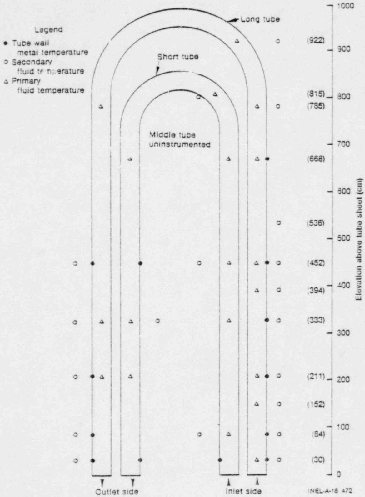
Figure 3. Intact loop steam generator thermocouple locations.
