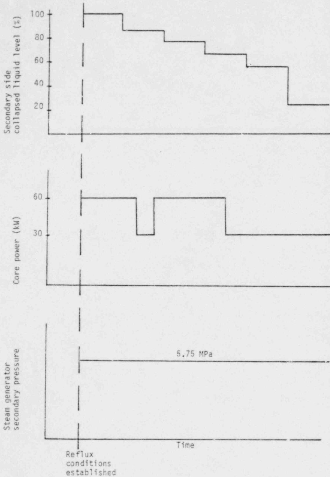
Figure 7. Idealized sequence of events for Test S-NC-4.
