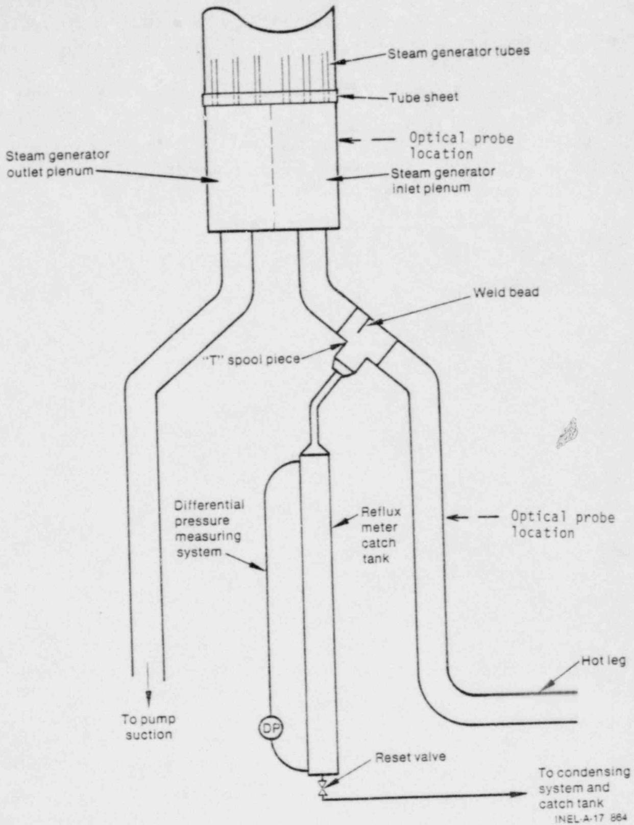
Figure 6. Reflux meter configuration.
