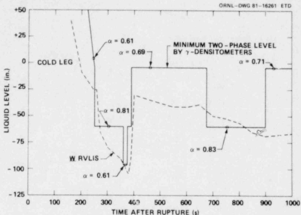
Fig. 8. Coolant levels in Semiscale for Westinghouse vessel dP and densitometers.
