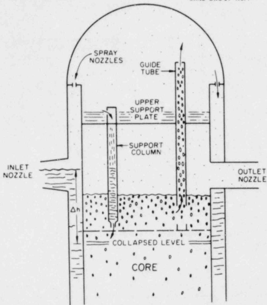
Fig. 9. Semiscale simulation of a PWR.
