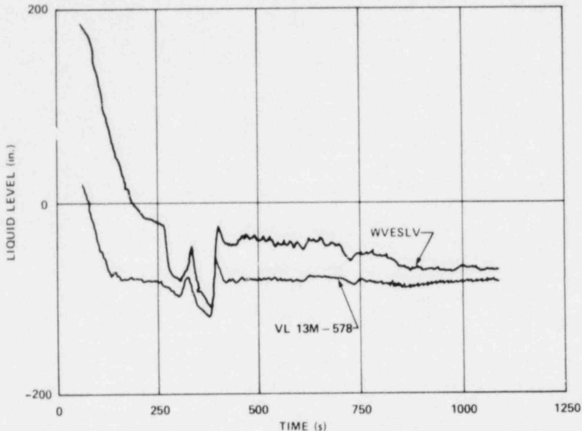
Fig. 3. Westinghouse collapsed liquid level (upper head to lower plenum) compared with Semiscale collapsed liquid level (-13 cm to lower plenum). Source: W. W. Tingle and R. W. Golden, *Installation and Initial Test Data Report: Westinghouse Reactor Vessel Level Indicating System Performance During Semiscale Test S-UT-3*, EGG-SF-5494 (June 1981).
