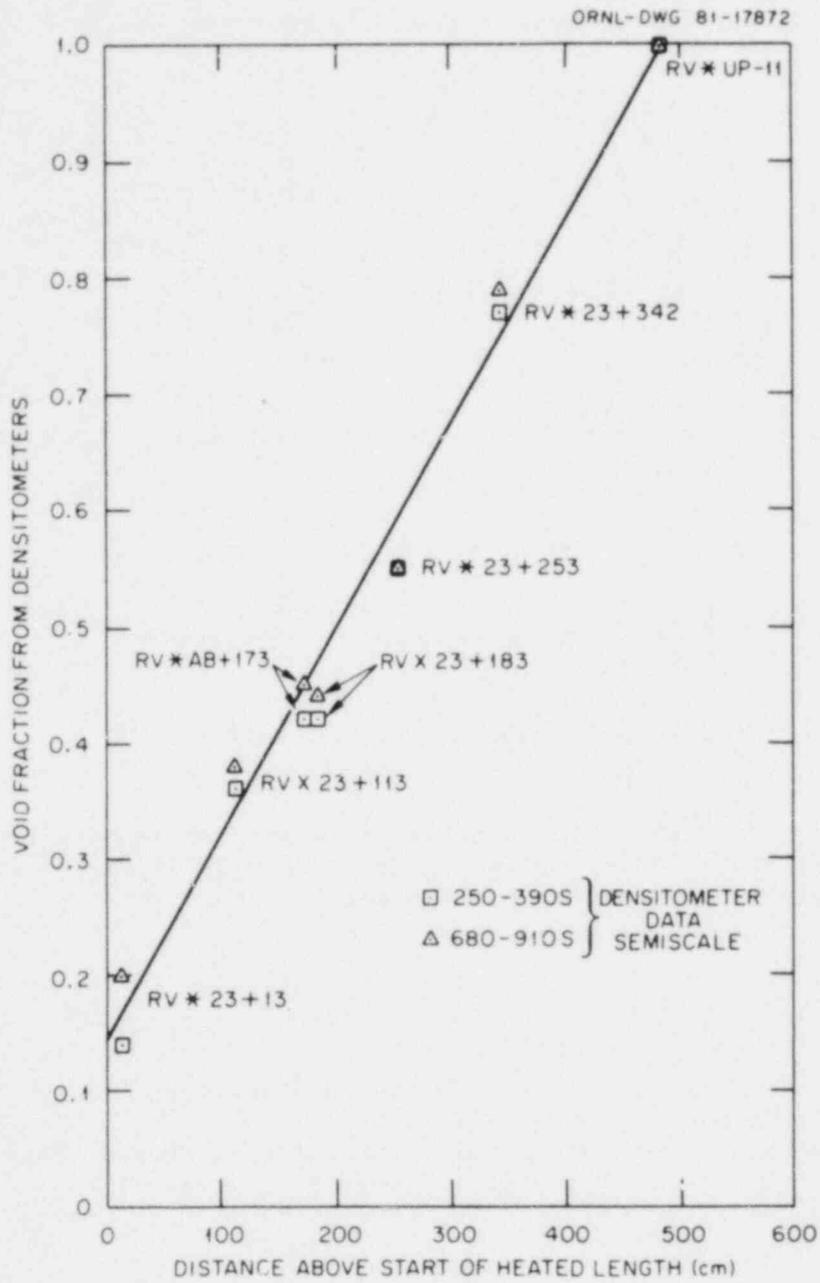
Fig. 5. Plot of void fraction based on densitometers.
