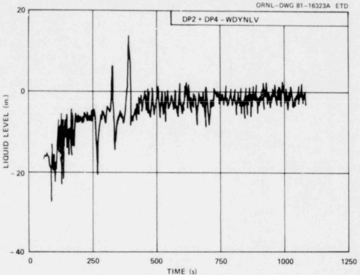
Fig. 6. Plot of difference between Westinghouse dynamic measurements and Semiscale measurements. (For entire vessel - note good agreement.)
