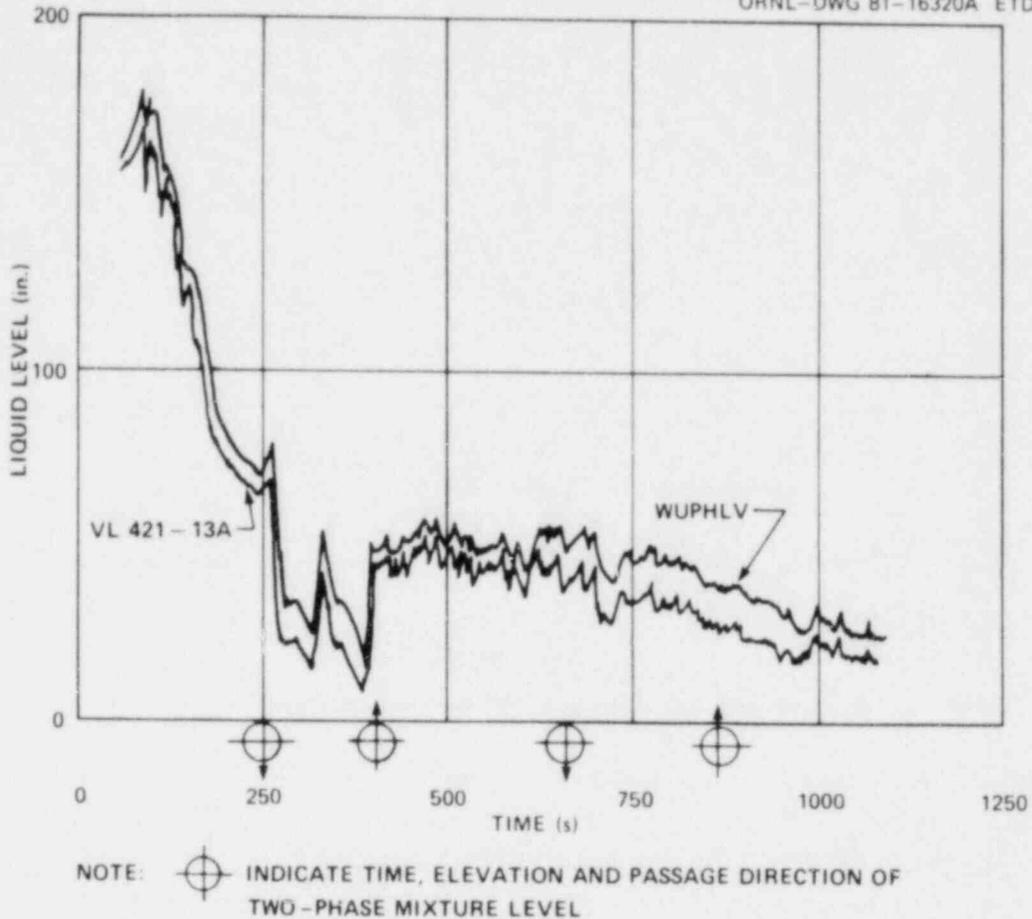
Fig. 2. Westinghouse and Semiscale upper-head and upper-plenum dP measurements. Source: W. W. Tingle and R. W. Golden, *Installation and Initial Test Data Report: Westinghouse Reactor Vessel Level Indicating System Performance During Semiscale Test S-UT-3*, EGG-SEMI-5494 (June 1981).
