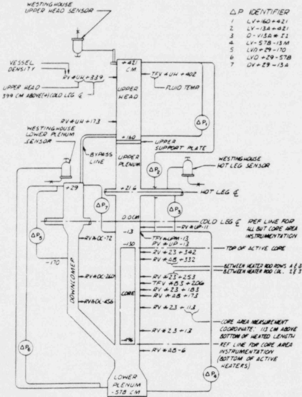
Fig. 1. Instrumentation of significance for the Westinghouse vessel liquid level indicating system test. Source: W. W. Tingle and R. W. Golden, *Installation and Initial Test Data Report: Westinghouse Reactor Vessel Level Indicating System Performance During Semiscale Test S-UT-3*, EGG-SEMI-5494 (June 1981).
