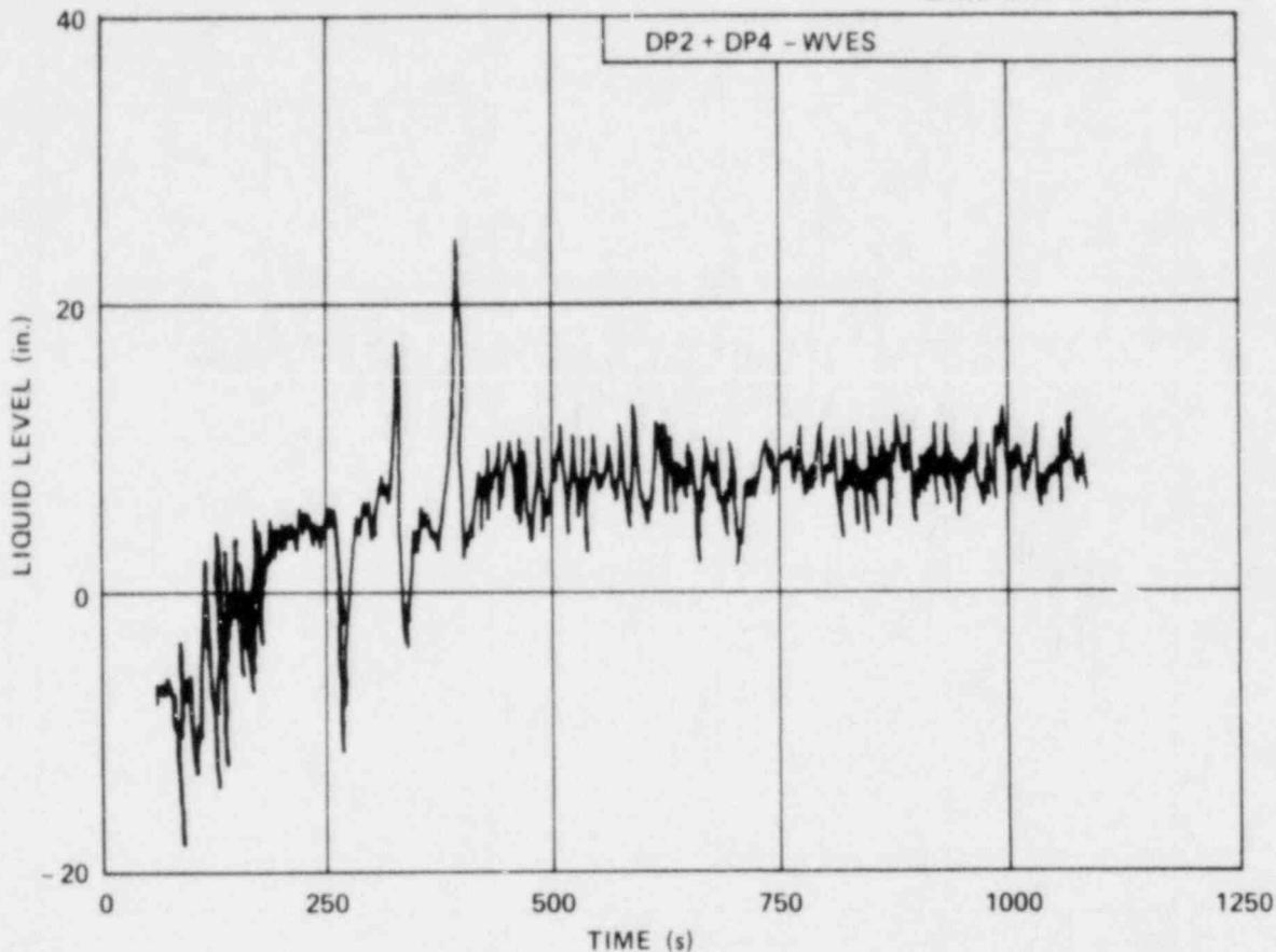
Fig. 7. Plot of difference between Westinghouse level measurements and Semiscale level measurements. (For entire vessel - note good agreement.)
