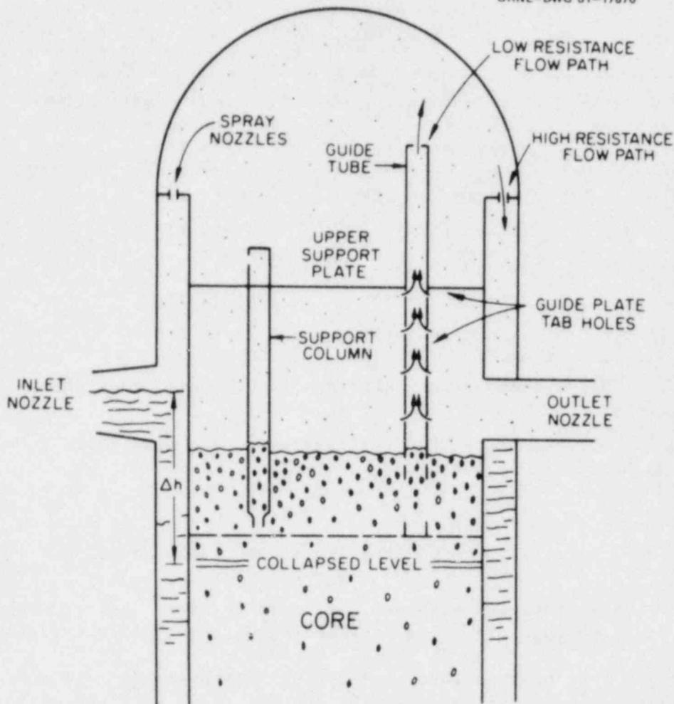
Fig. 10. Westinghouse reactor vessel configuration (PWR).
