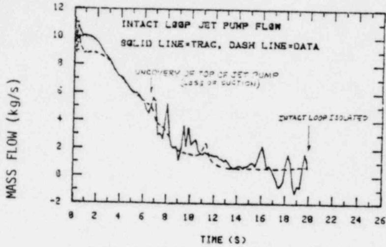
FIG. 3 INTACT LOOP JET PUMP FLOW
