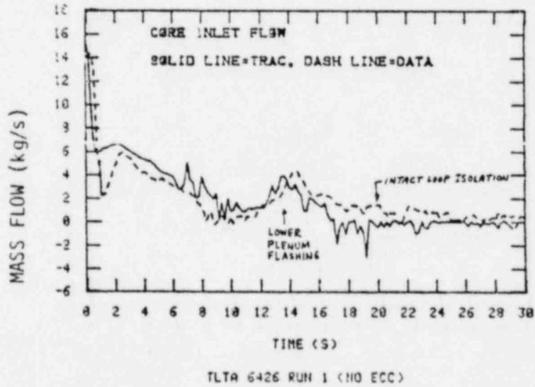
FIG. 2 CORE INLET FLOW
