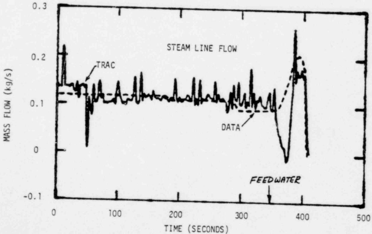
FIG. 19 STEAM LINE MASS FLOW RATE
