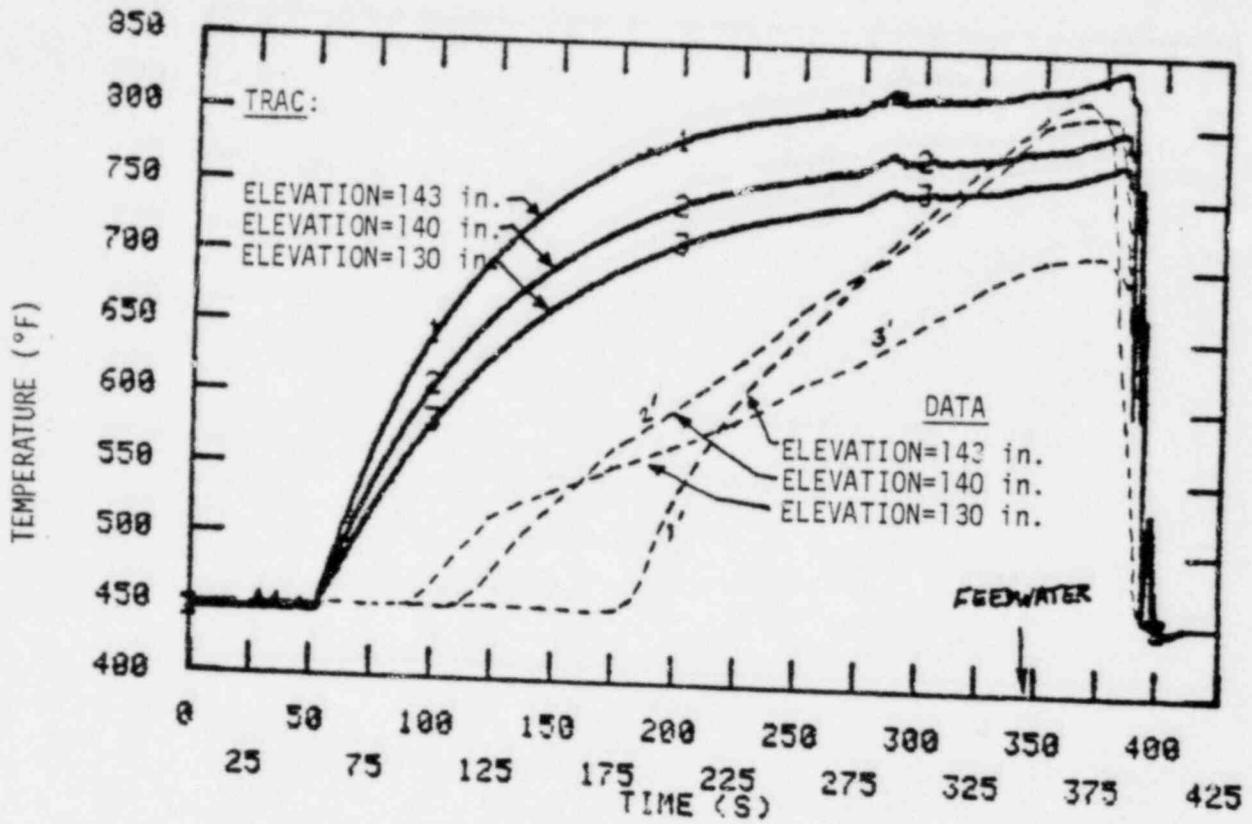
FIG. 18 ROD TEMPERATURES AT BUNDLE UPPER ELEVATIONS
