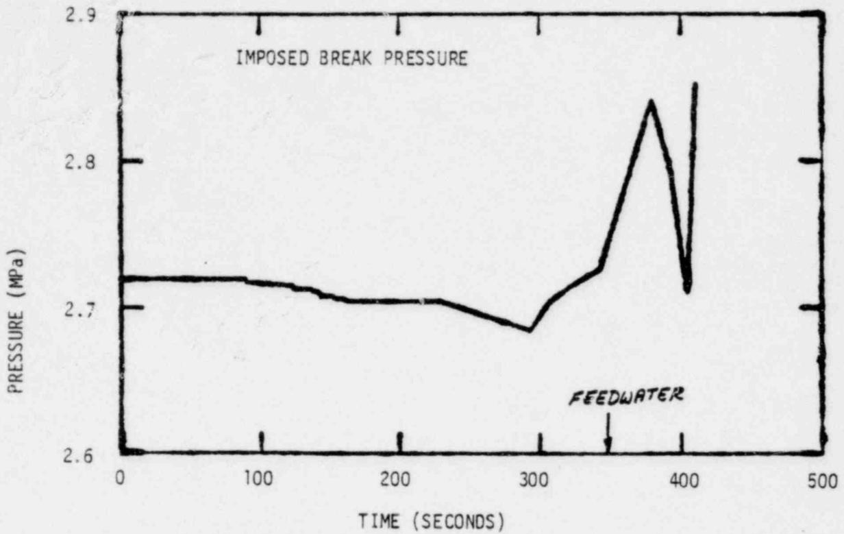
FIG. 16 PRESSURE BOUNDARY CONDITION IMPOSED AT VESSEL TOP
