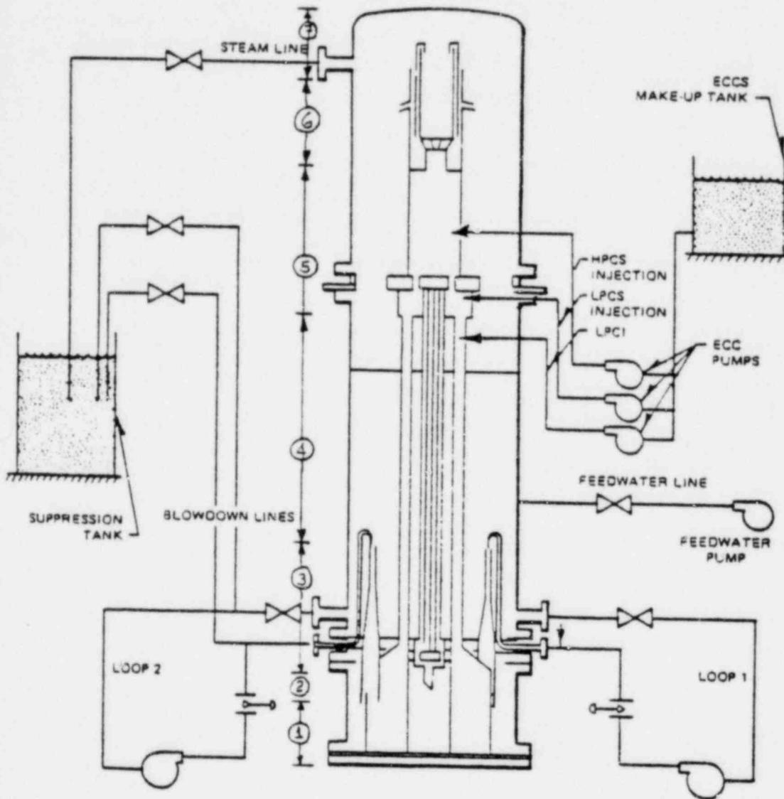
Figure 1. TLTA5 (Two-Loop Test Apparatus Configuration 5) with ECCS showing Minimum Number of Axial Levels for a DBA LOCA Test
