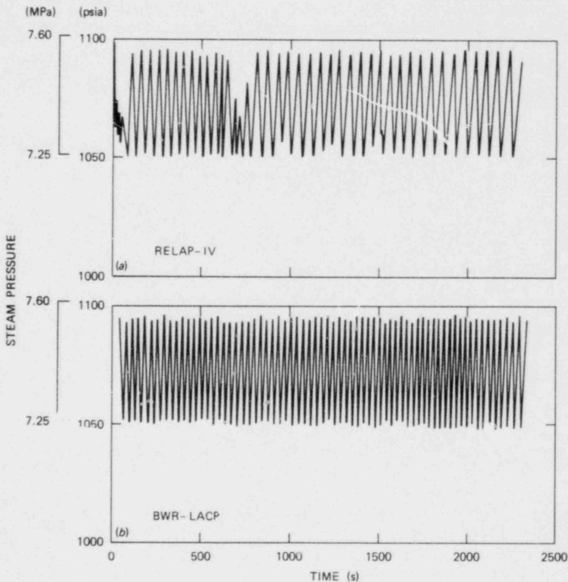
Fig. 4.6 Comparison of RELAP-IV and BWR-LACP results for reactor vessel pressure.
