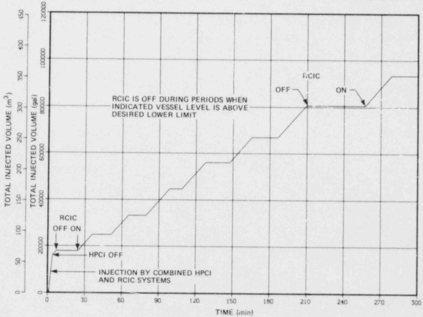
Fig. 7.5 Normal recovery after station blackout - total injected flow.
