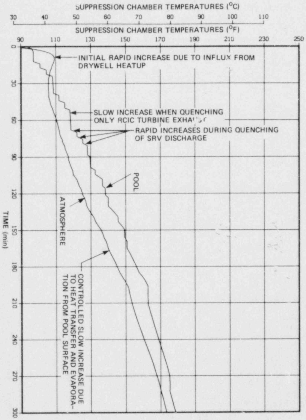
Fig. 7.7 Normal recovery after station blackout - suppression chamber temperatures.
