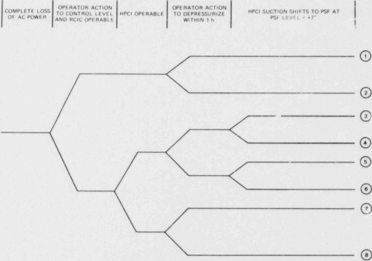
Fig. 8.1 Event tree for initial phase of a station blackout in which DC power remains available.
