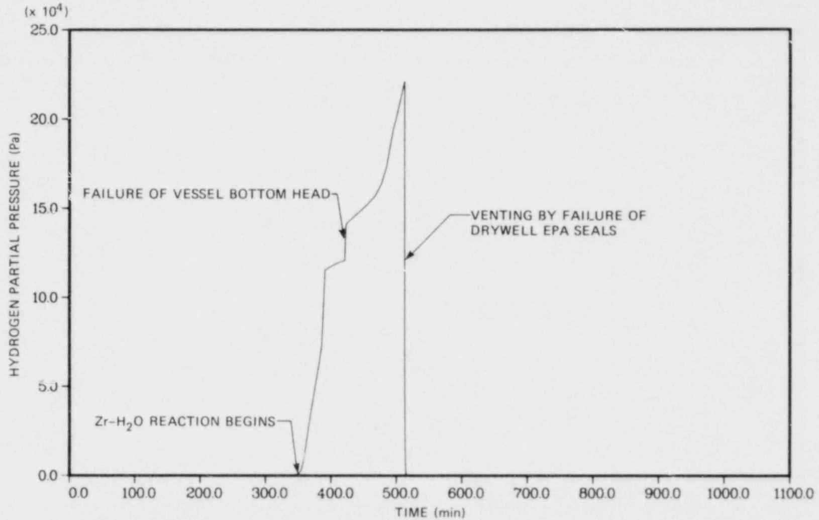
Fig. 9.41 Wetwell hydrogen partial pressure (TB').
