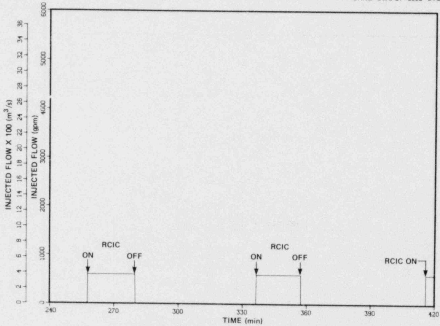
Fig. G.4 Injected flow - four to seven hours after station blackout.
