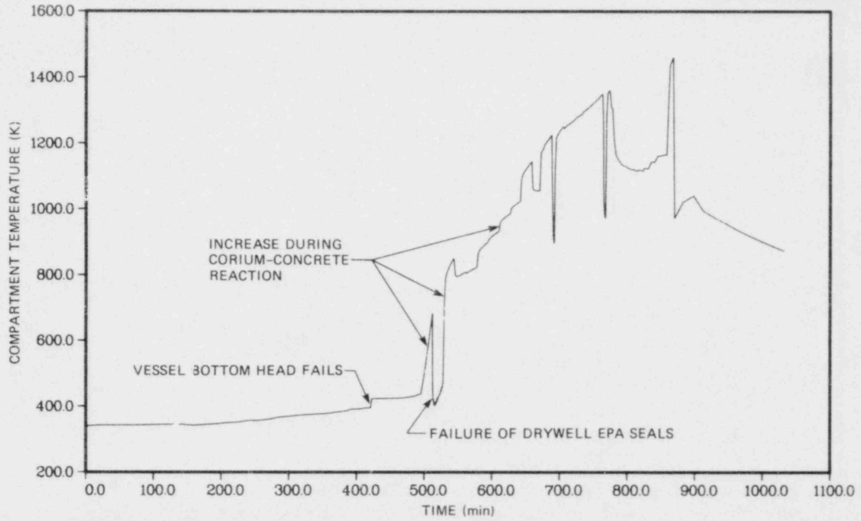
Fig. 9.27 Drywell temperature distribution (TB').
