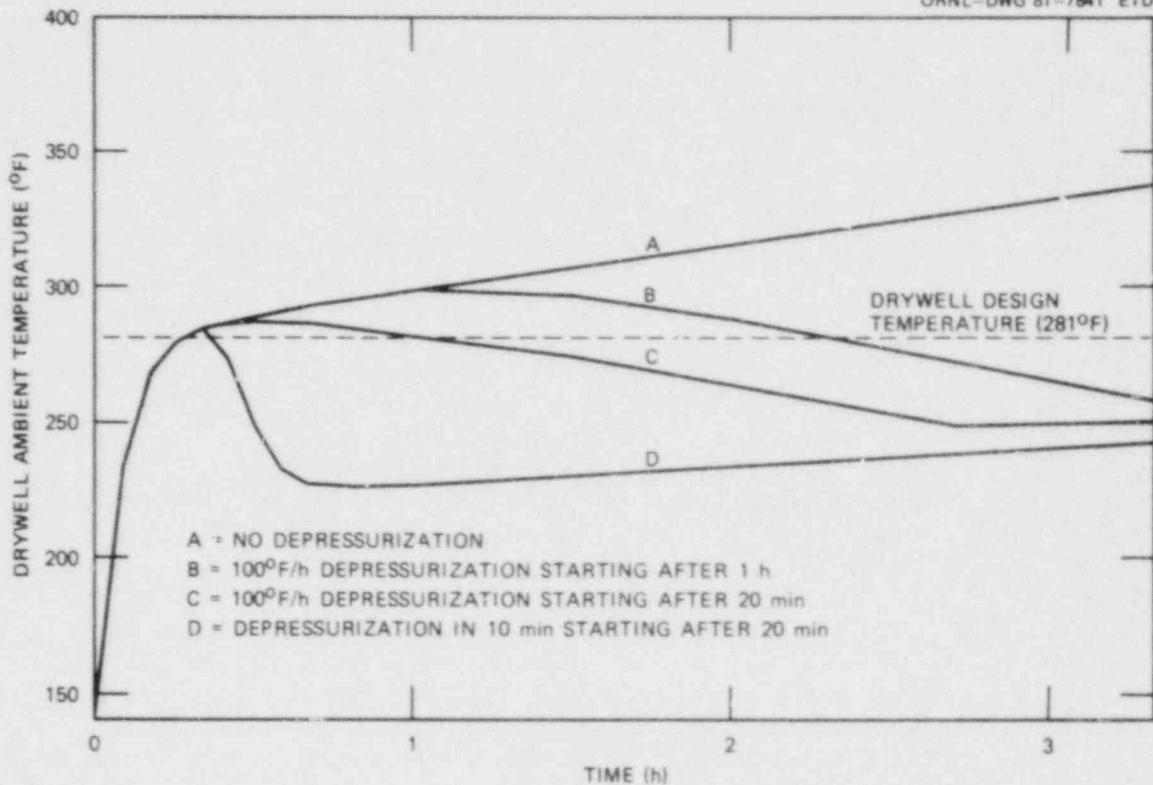
Fig. 3.3 Average drywell temperature during a station blackout.
