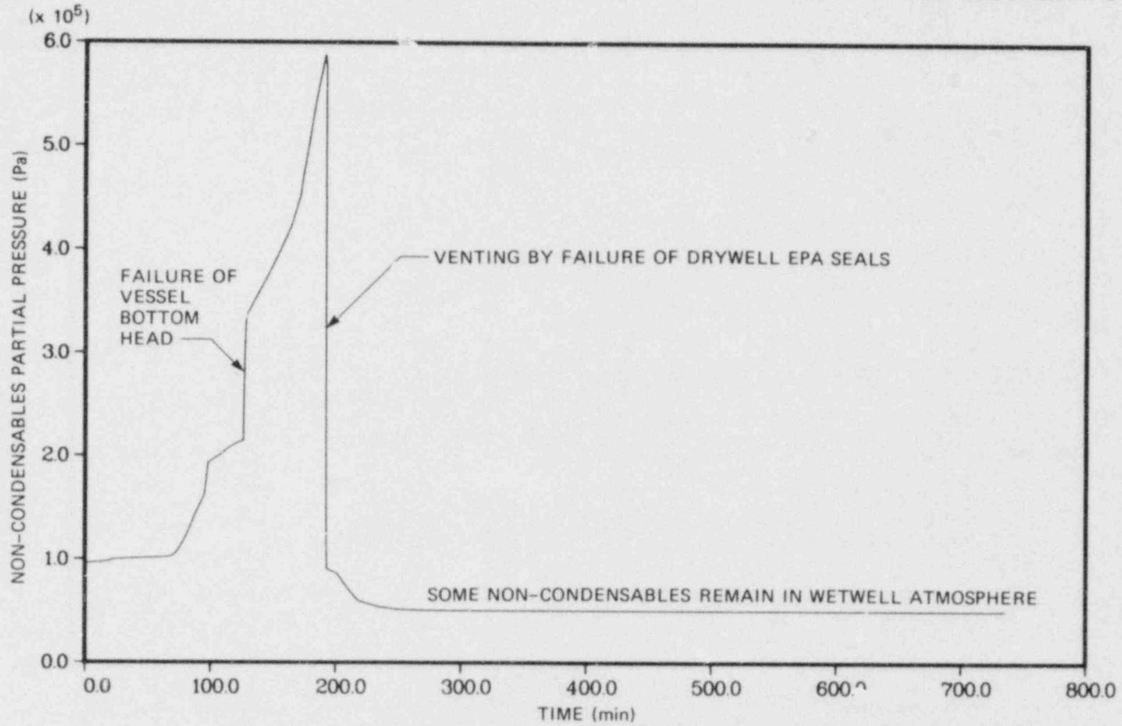
Fig. 9.46 Wetwell non-condensables partial pressure (TUB').
