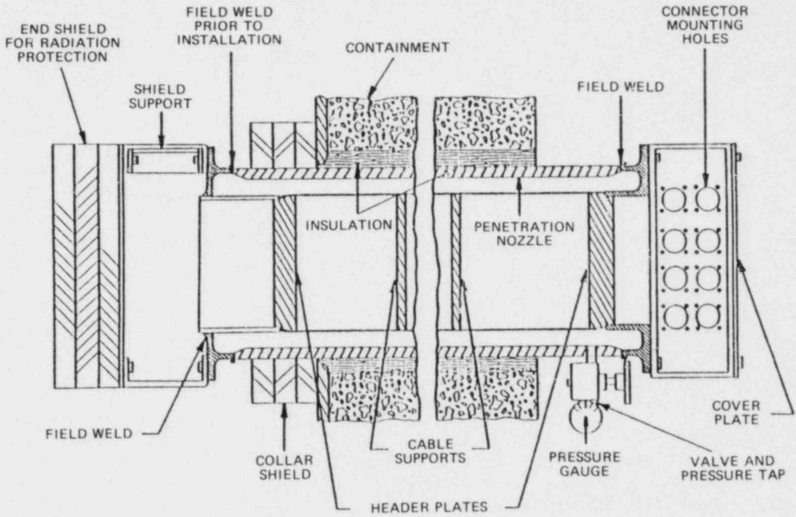
Fig. 9.22 Typical electrical penetration assembly canister.
