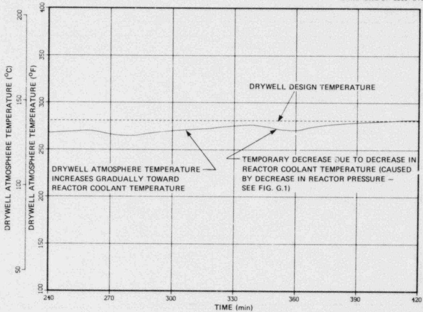
Fig. G.8 Drywell temperatures - four to seven hours after station blackout.
