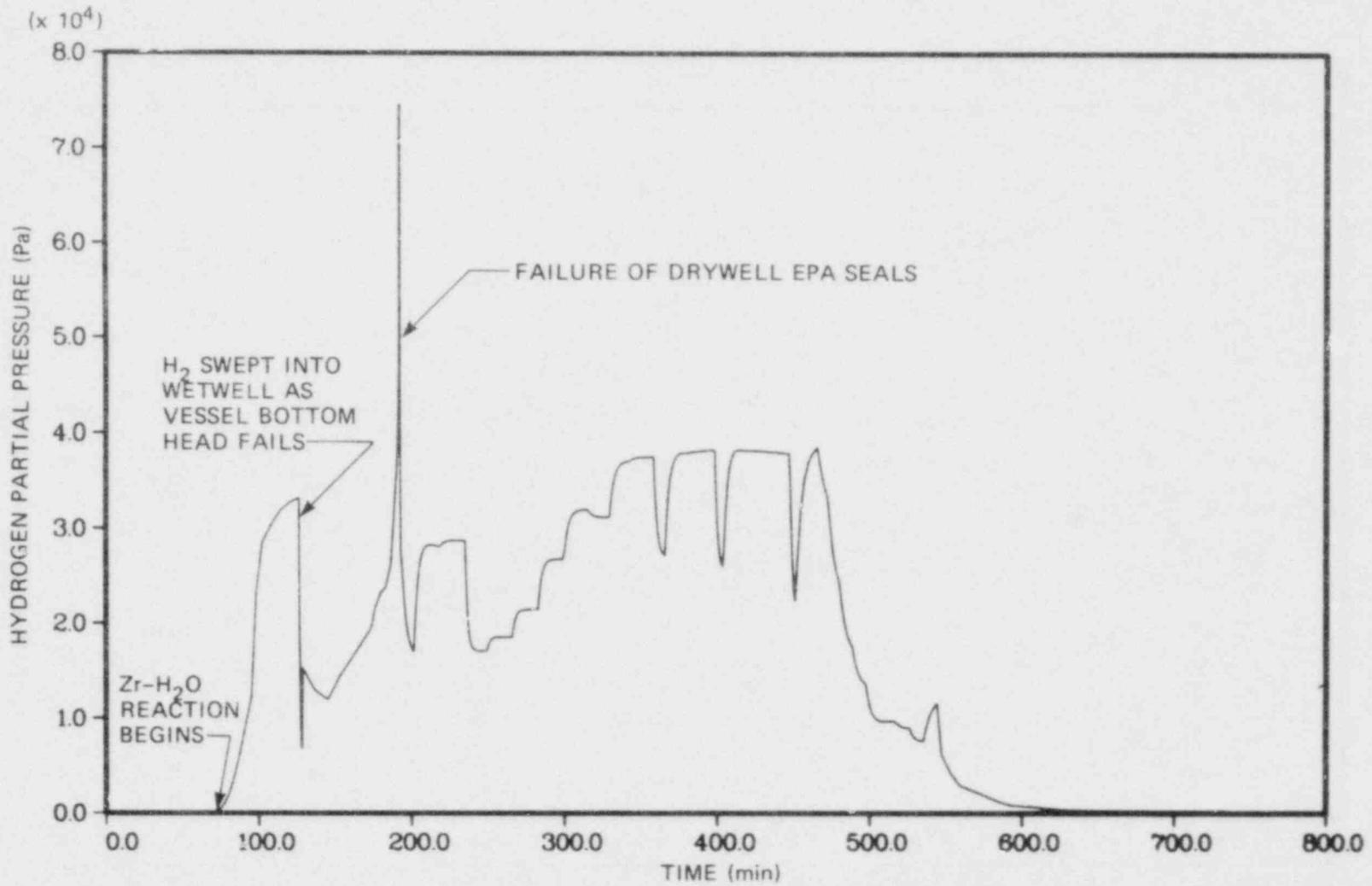
Fig. 9.35 Drywell hydrogen partial pressure (TUB').
