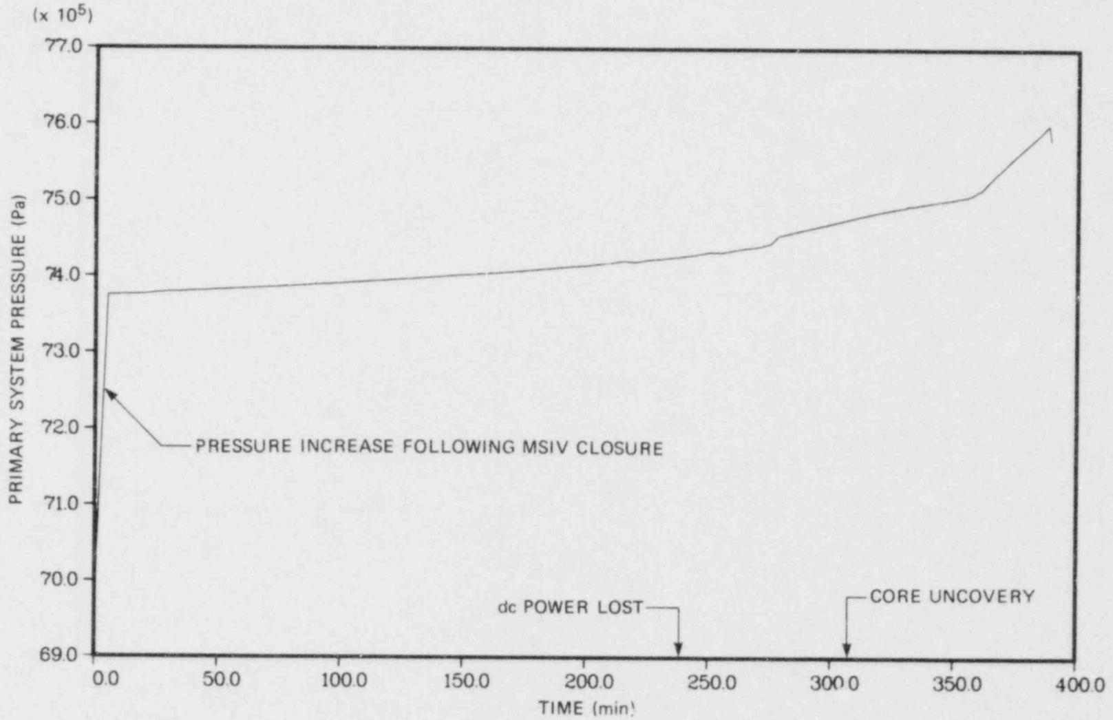
Fig. 9.12 Reactor vessel pressure.
