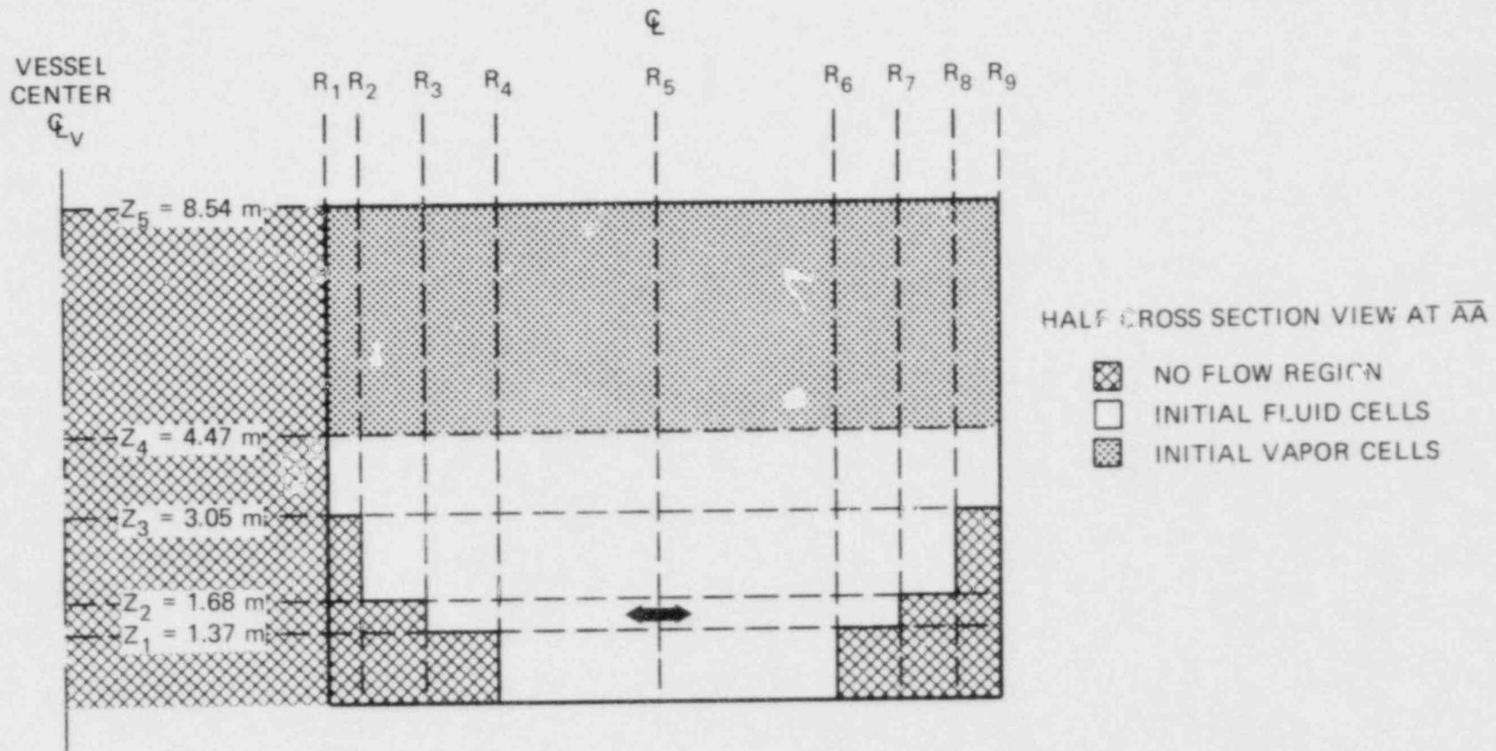
Fig. D.5 Suppression pool model cross section.
