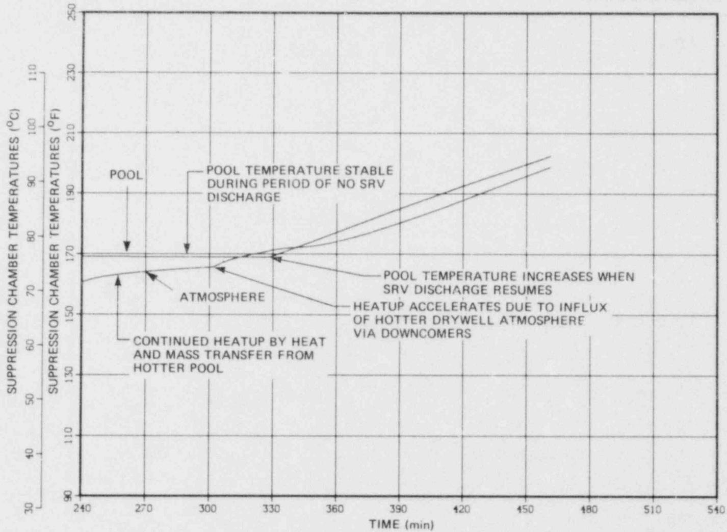
Fig. 7.14 Loss of 250 VDC batteries - suppression chamber temperatures.
