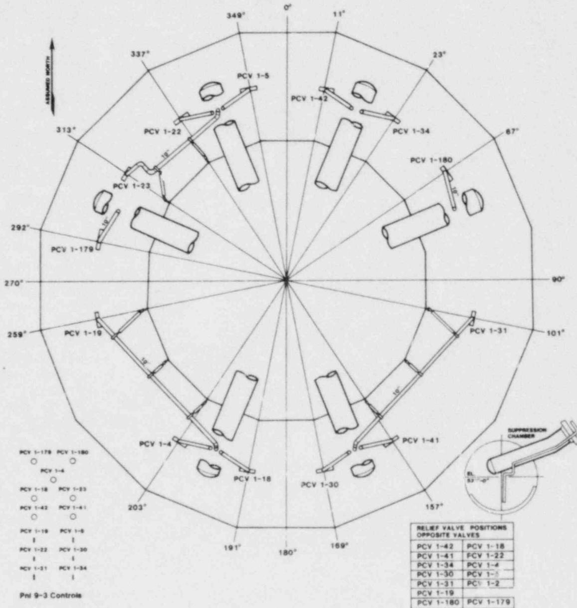
Fig. 3.2 Unit 1 relief valve discharges.
