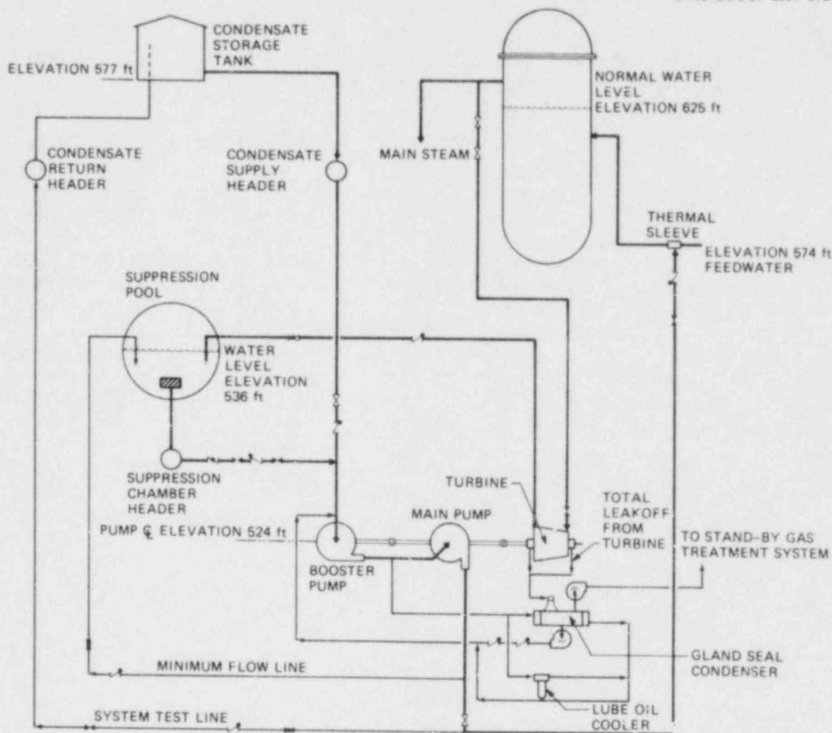
Fig. E.1 High pressure coolant injection system.
