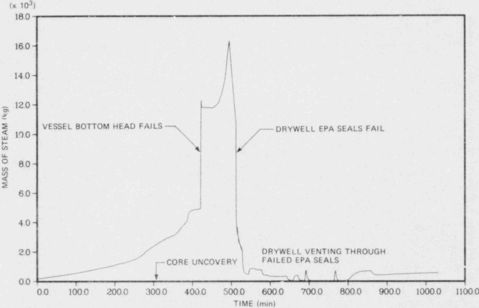
Fig. 9.23 Mass of steam in drywell.
