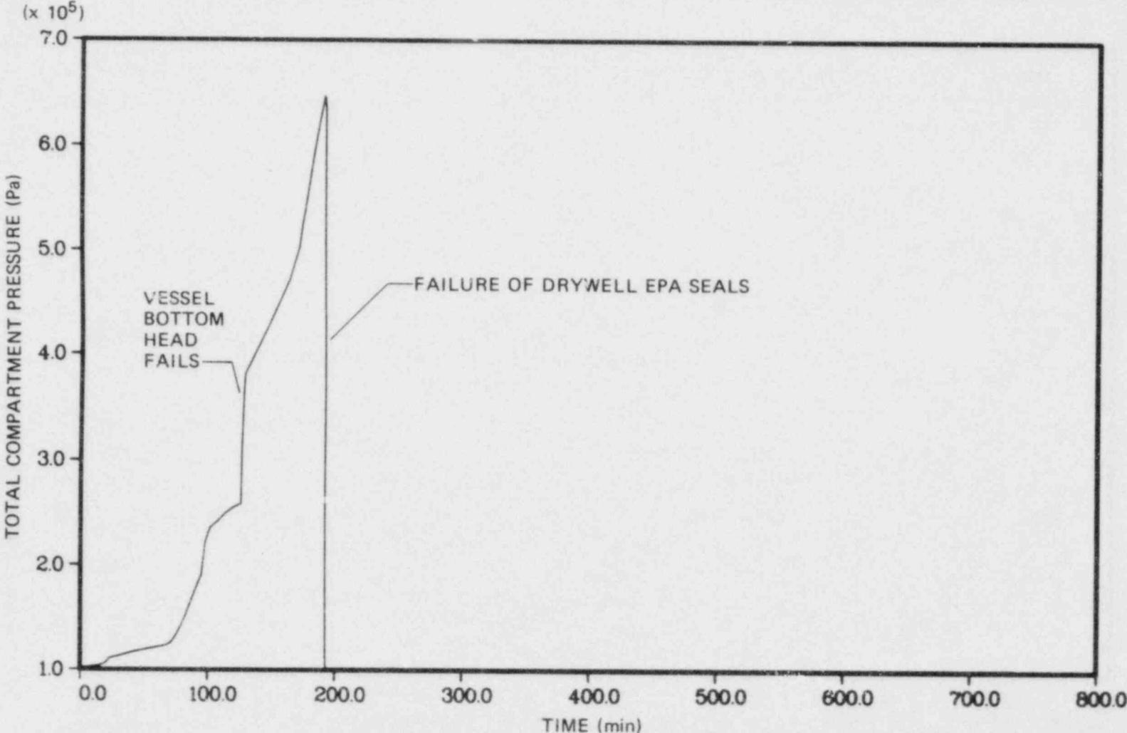
Fig. 9.33 Drywell total pressure (TUB').
