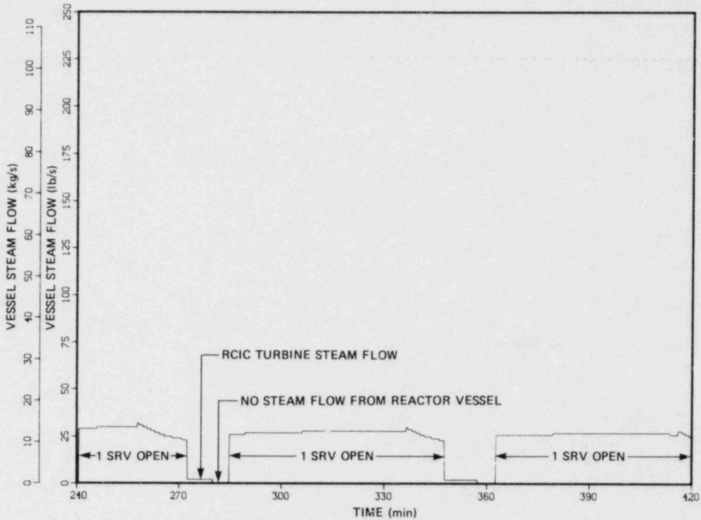
Fig. G.2 Vessel steam flow - four to seven hours after station blackout.
