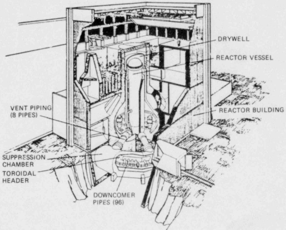
Fig. D.1 BWR reactor building showing primary containment system enclosed.
