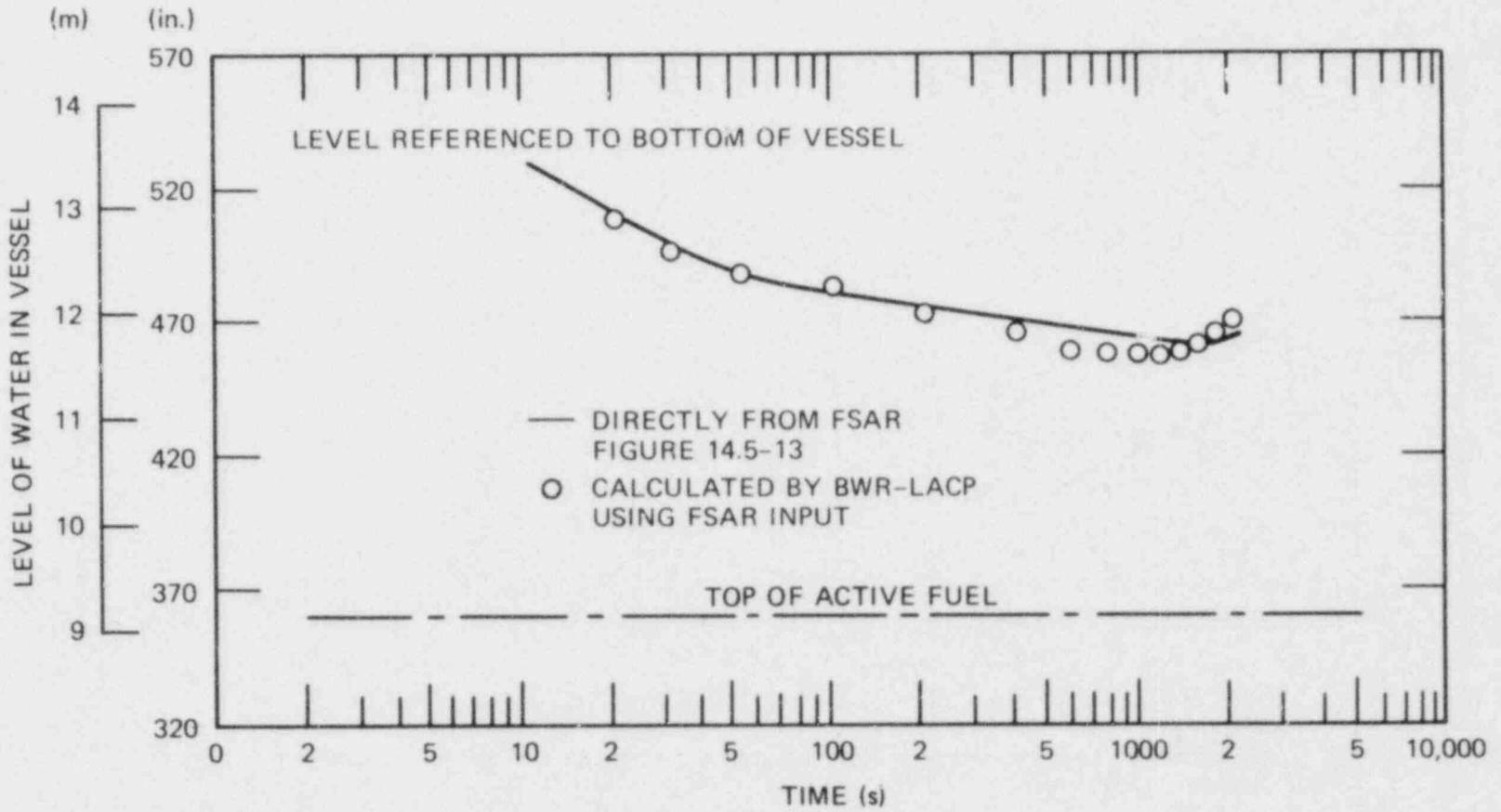
Fig. 4.3 Comparison of FSAR and BWR-LACP results for reactor vessel level.
