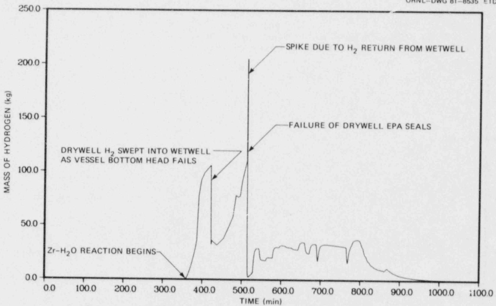
Fig. 9.24 Mass of hydrogen in drywell.
