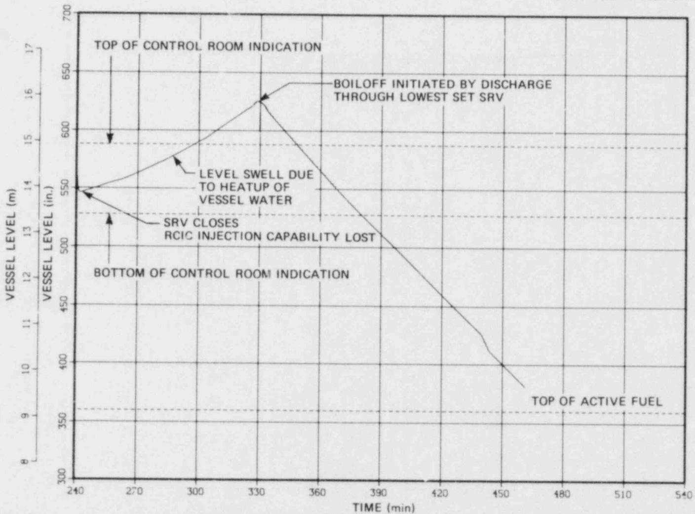
Fig. 7.12 Loss of 250 VDC batteries - vessel level.
