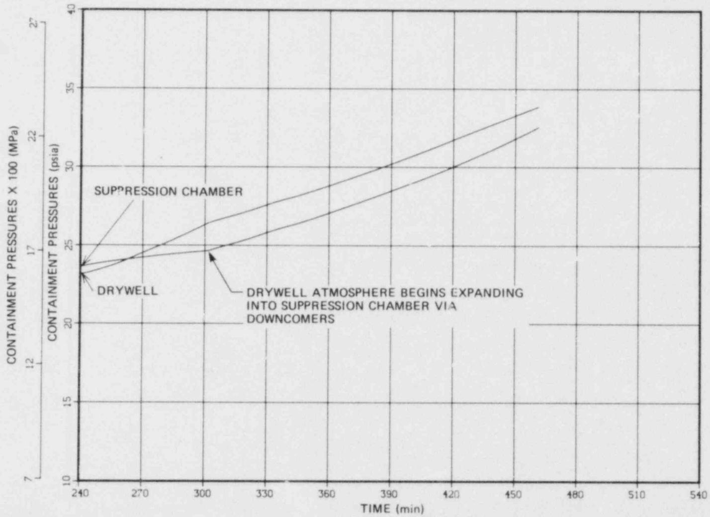
Fig. 7.15 Loss of 250 VDC batteries - containment pressures.
