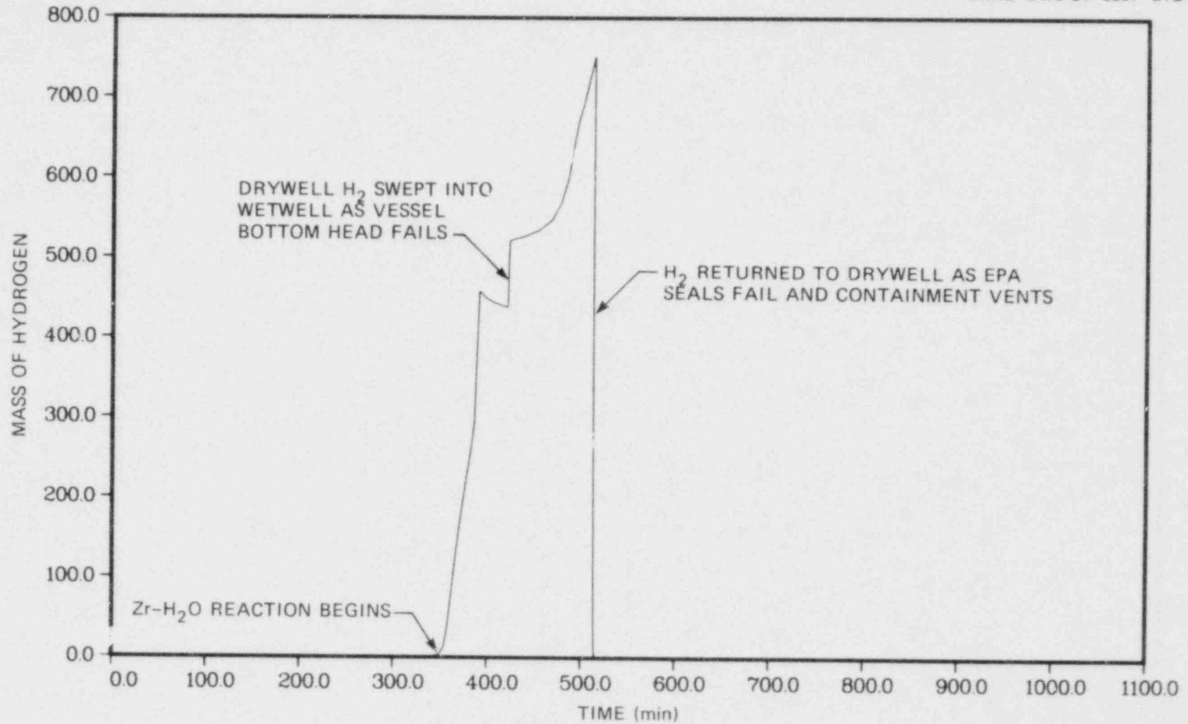
Fig. 9.26 Mass of hydrogen in wetwell.
