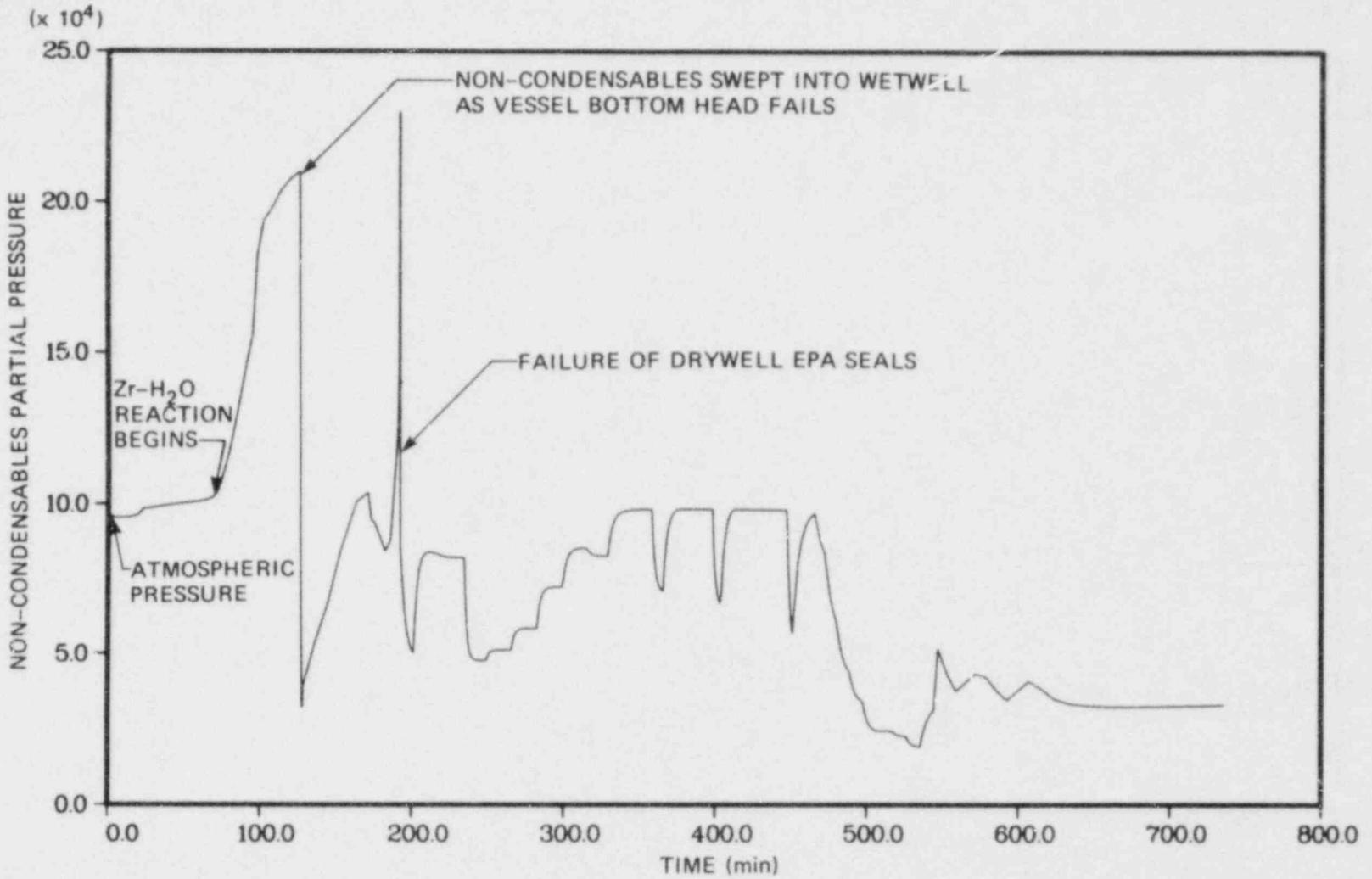
Fig. 9.36 Drywell non-condensables partial pressure (TUB').
