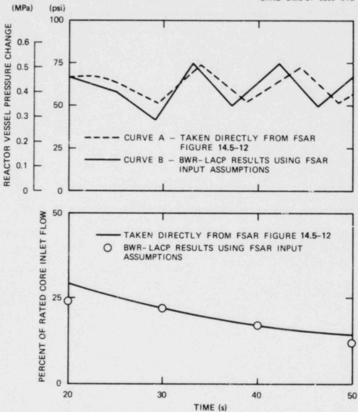
Fig. 4.2 Comparison of FSAR and BWR-LACP results for loss of auxiliary power transients.
