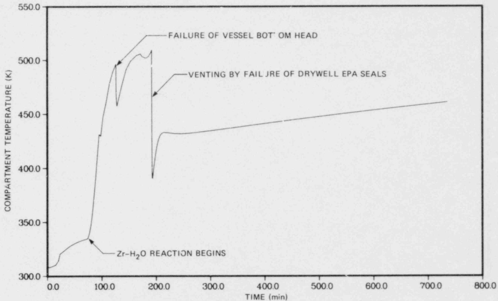
Fig. 9.38 Wetwell temperature distribution (TUB').
