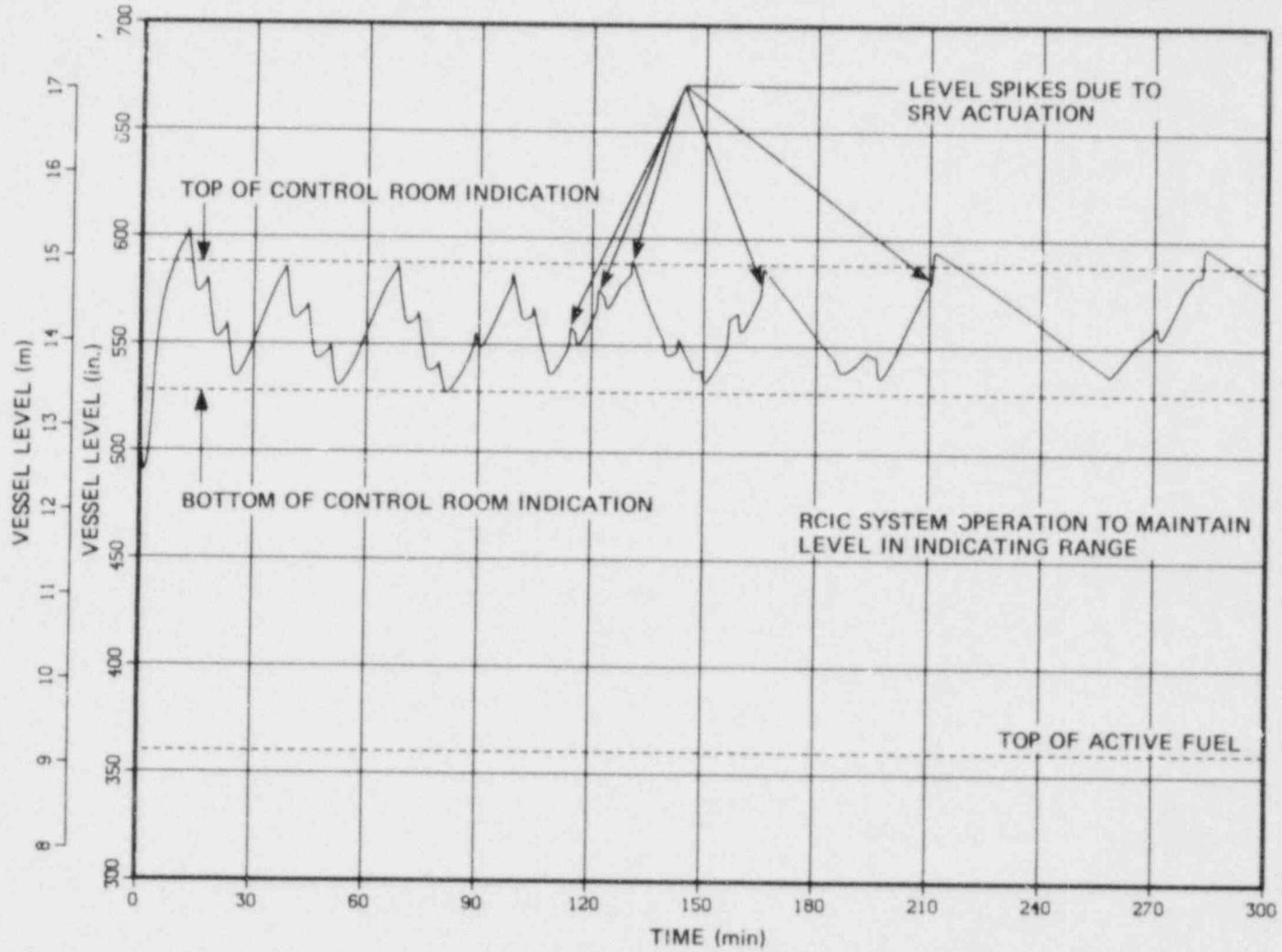
Fig. 7.3 Normal recovery after station blackout - reactor vessel level.
