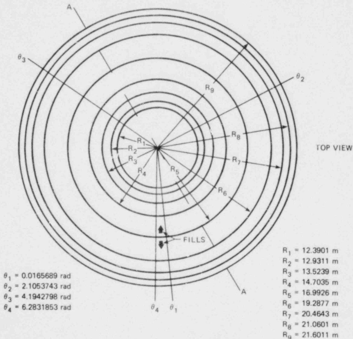
Fig. D.4 Suppression pool model top view.
