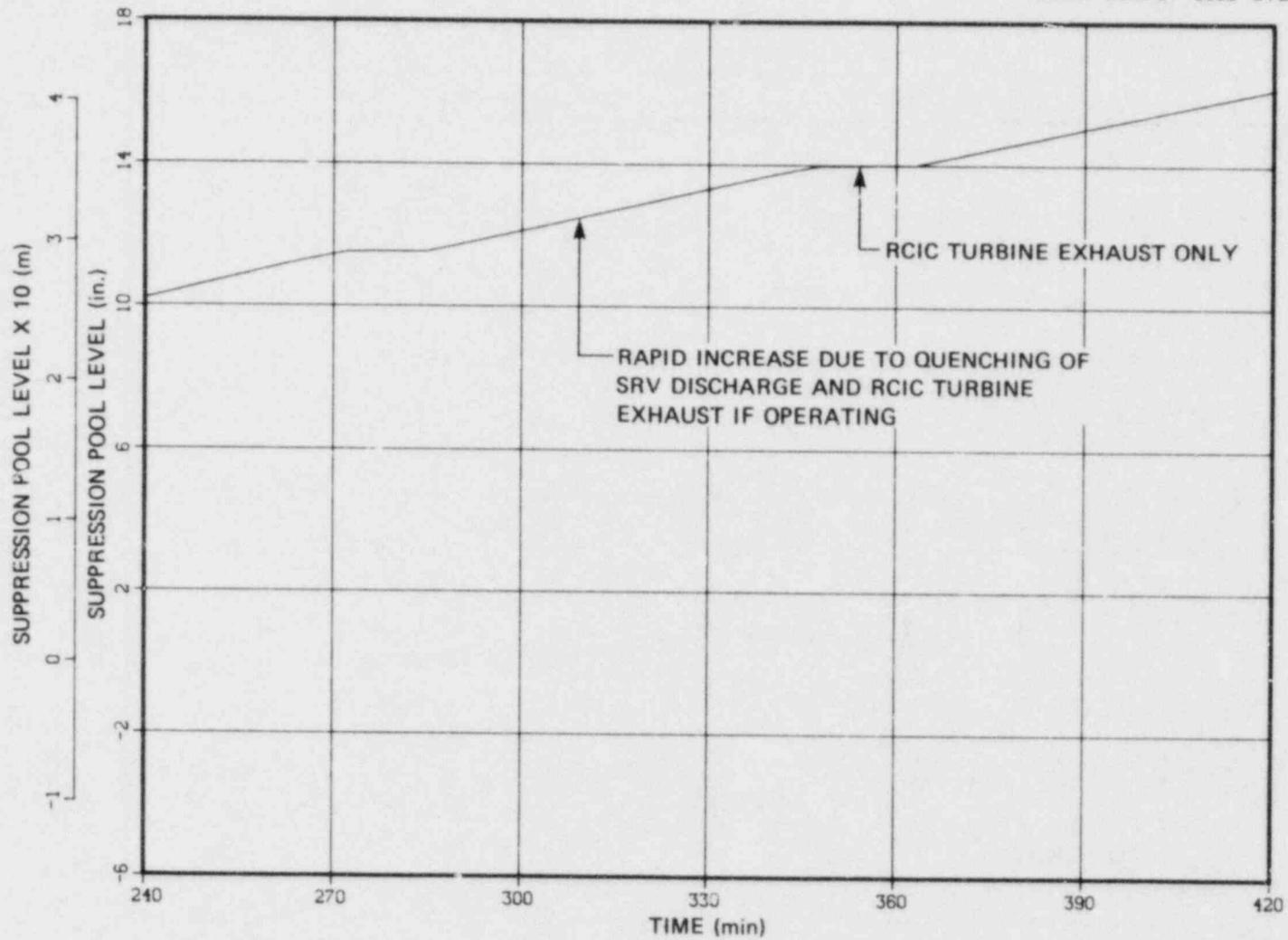
Fig. G.6 Suppression pool level - four to seven hours after station blackout.
