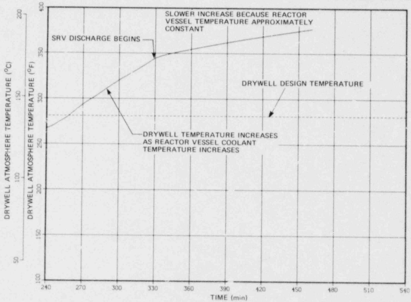
Fig. 7.16 Loss of 250 VDC batteries - drywell atmosphere temperature.
