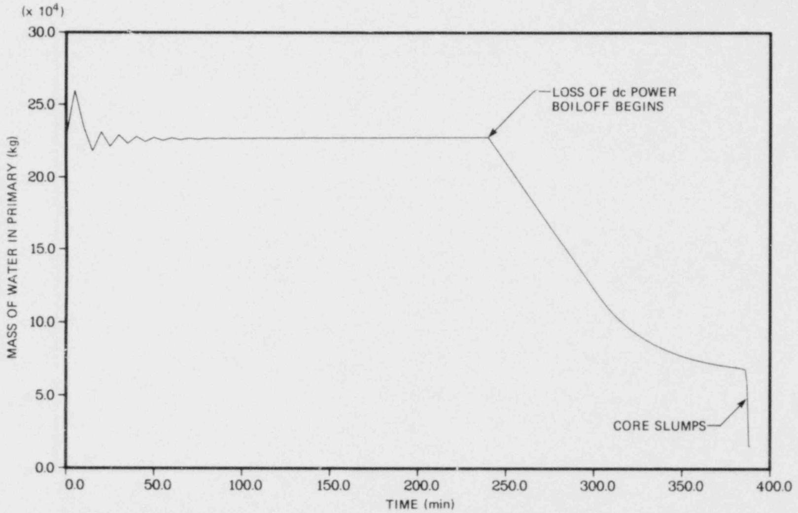
Fig. 9.15 Mass of water in primary system.
