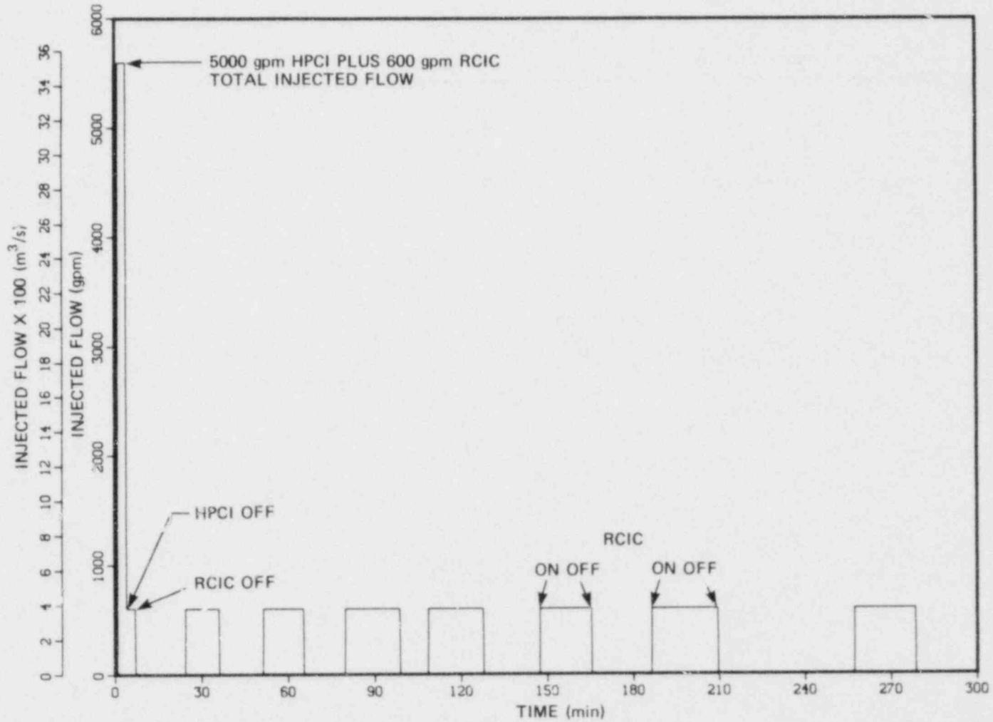
Fig. 7.4 Normal recovery after station blackout - injection flow.
