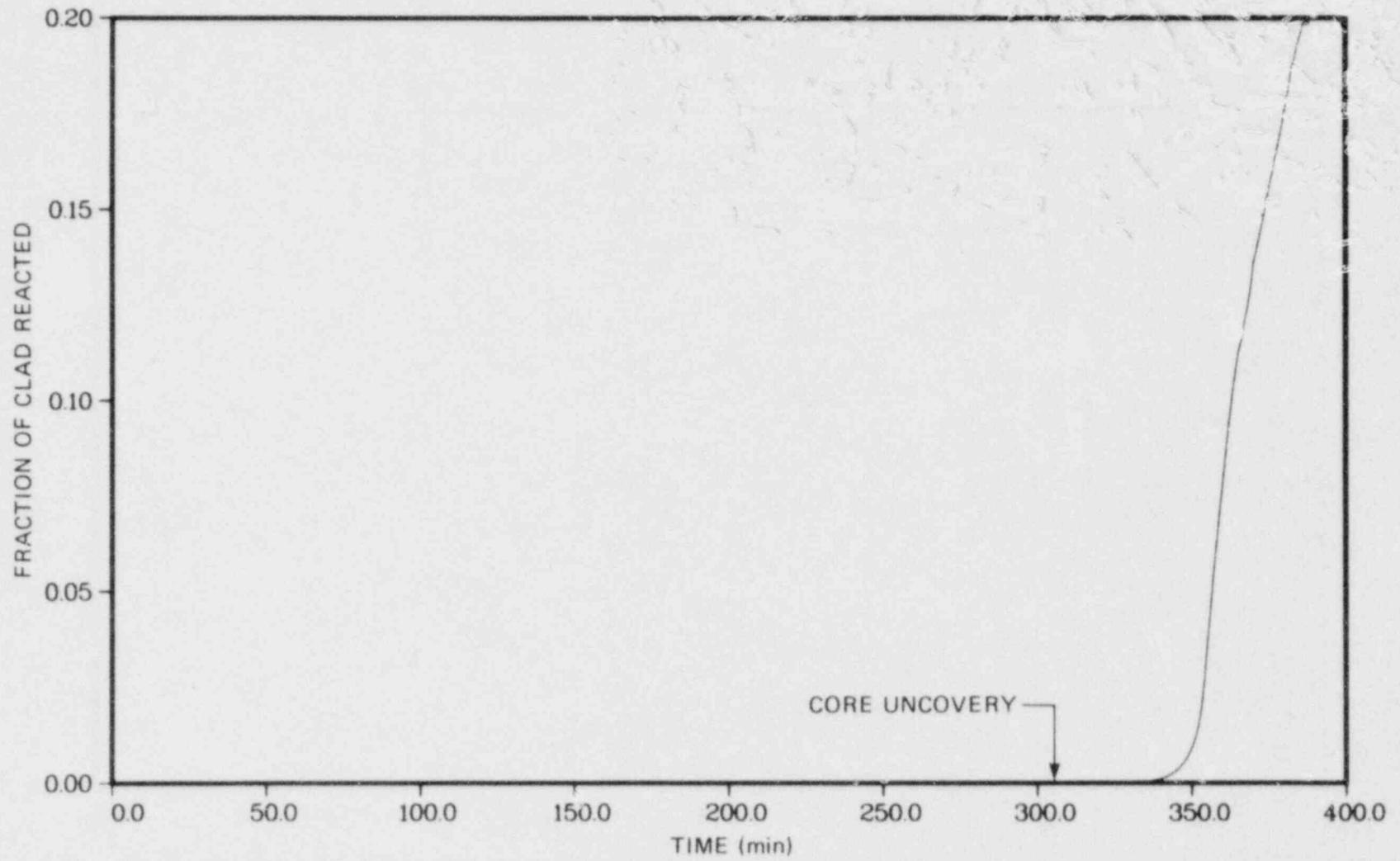
Fig. 9.18 Fraction of clad reacted.
