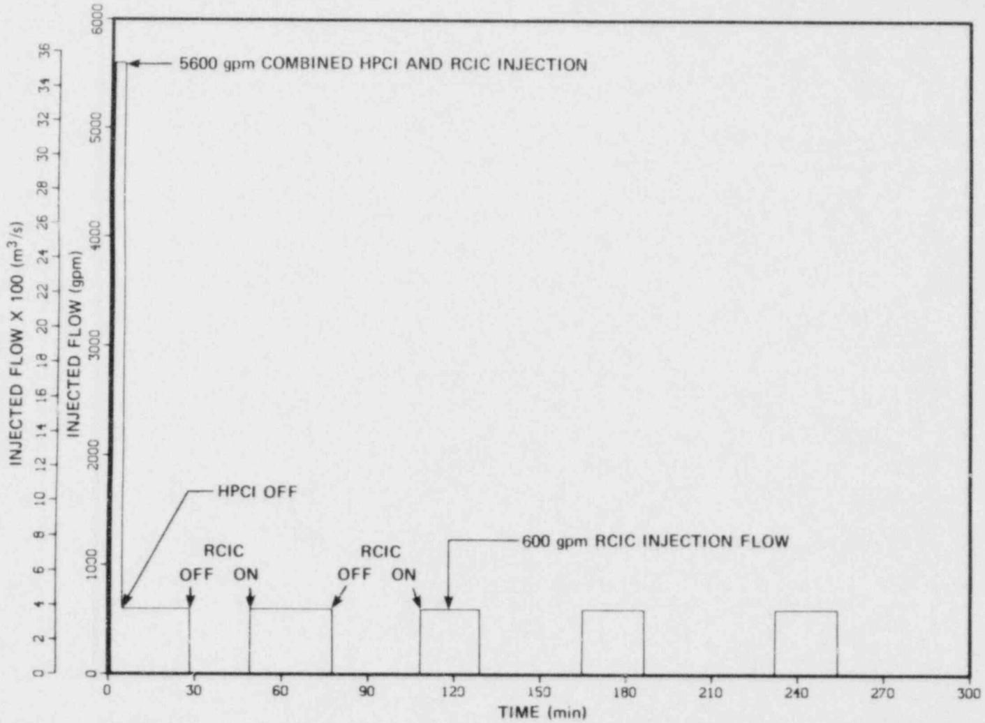
Fig. 8.3 Reactor vessel water injection with a stuck-open relief valve during a station blackout.
