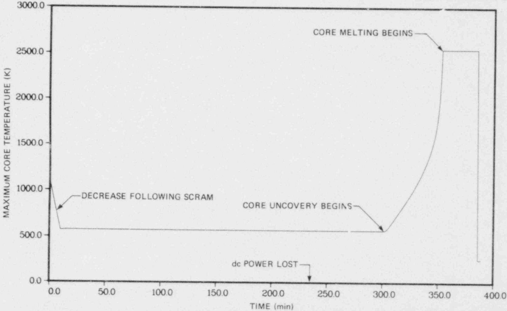
Fig. 9.4 Maximum core temperature (MARCH/MOD 1.4B).
