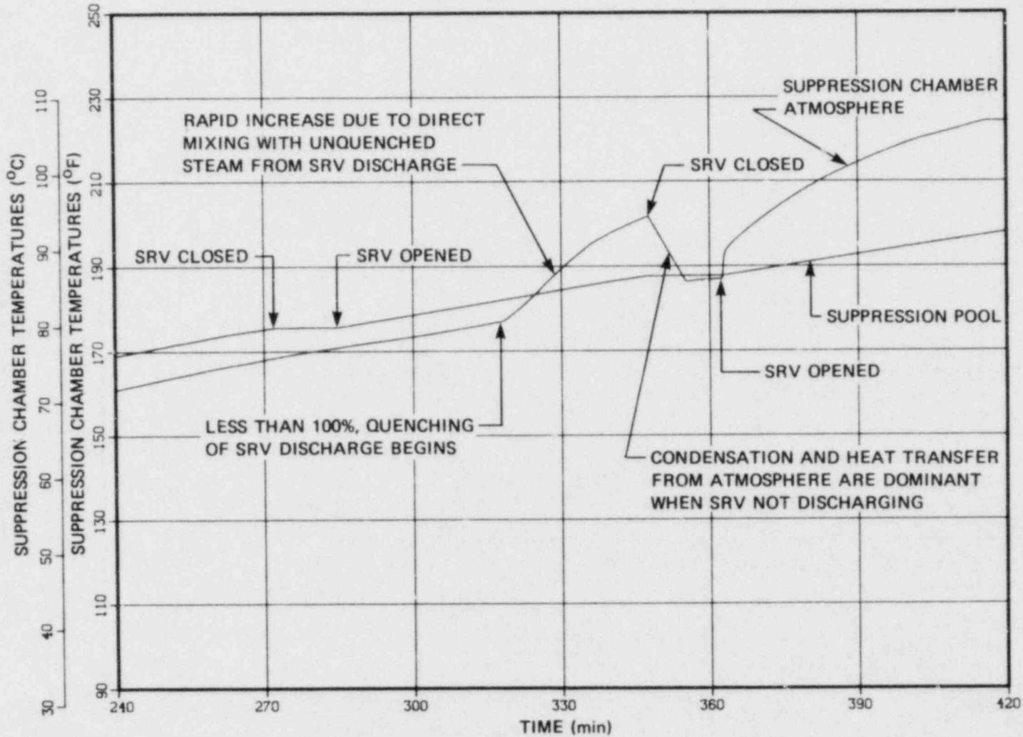
Fig. G.7 Suppression chamber temperatures - four to seven hours after station blackout.
