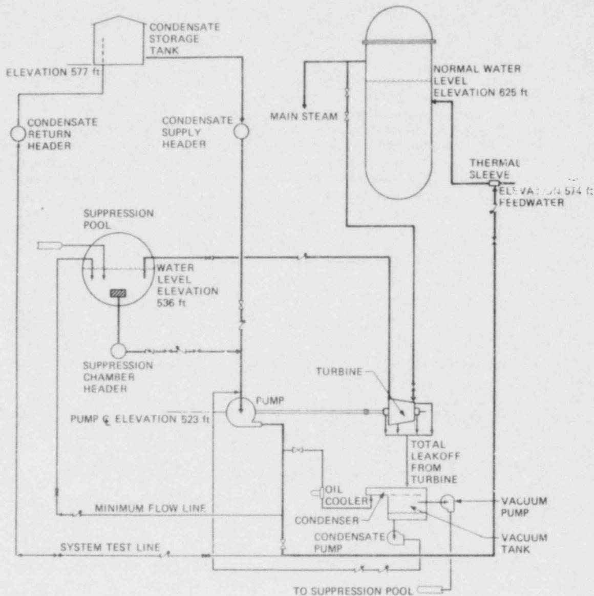
Fig. F.1 Reactor core isolation cooling system.
