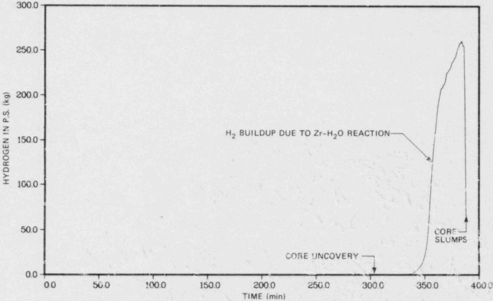
Fig. 9.17 Hydrogen mass in primary system.
