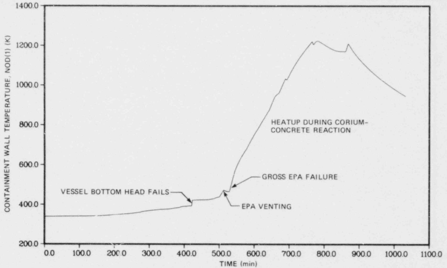
Fig. 9.8 Containment wall temperature (MARCH/MOD 1.4B).
