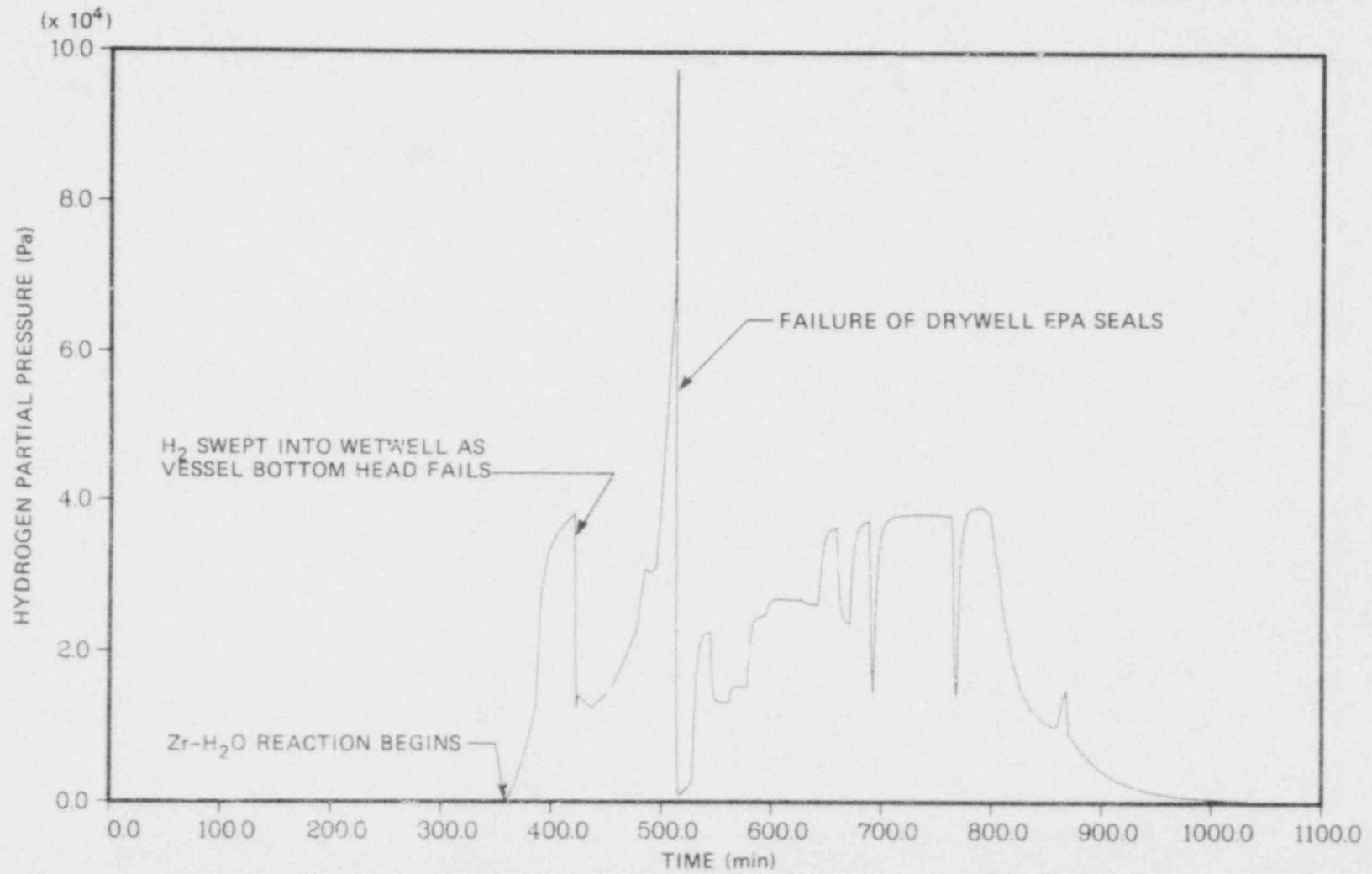
Fig. 9.31 Drywell hydrogen partial pressure (TB').
