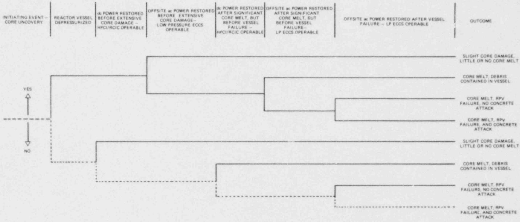
Fig. 9.2 Core damage event tree.
