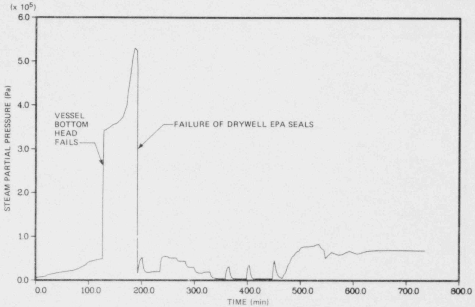
Fig. 9.34 Drywell steam partial pressure (TUB').
