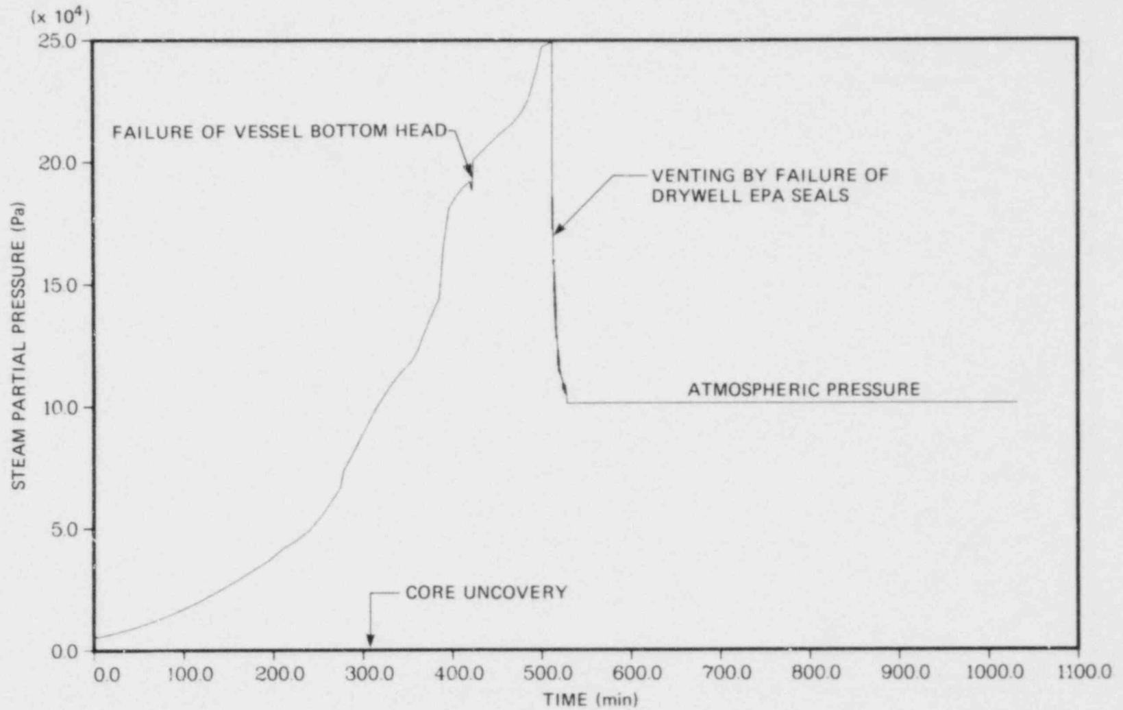
Fig. 9.40 Wetwell steam partial pressure (TB').
