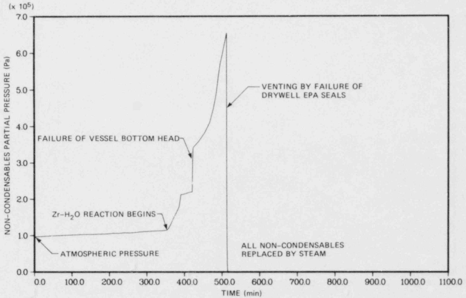
Fig. 9.42 Wetwell non-condensables partial pressure (TB').
