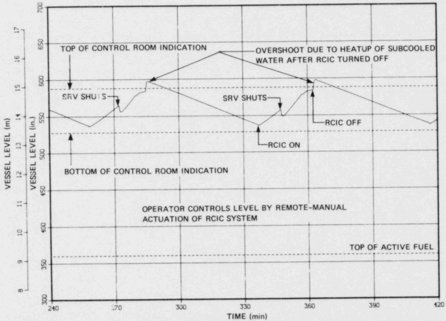
Fig. G.3 Vessel level - four to seven hours after station blackout.
