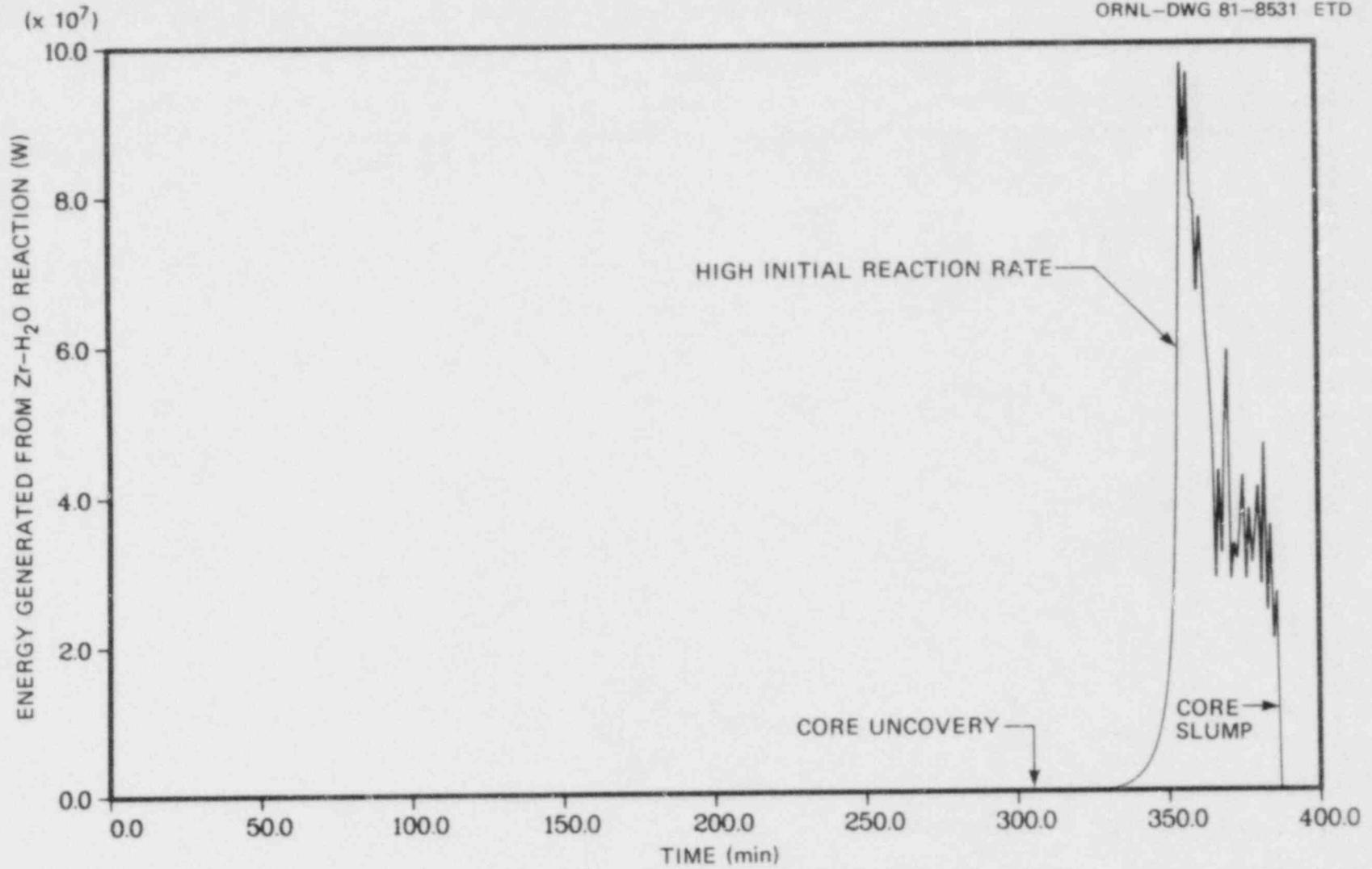
Fig. 9.20 Energy generated from Zr-H<sub>2</sub>O reaction.
