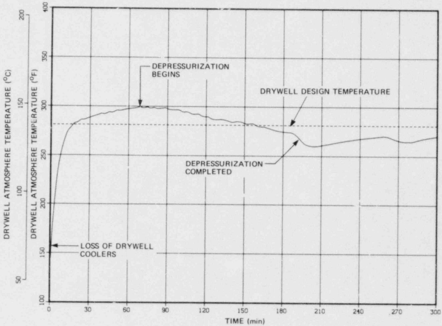
Fig. 7.8 Normal recovery after station blackout - drywell temperatures.
