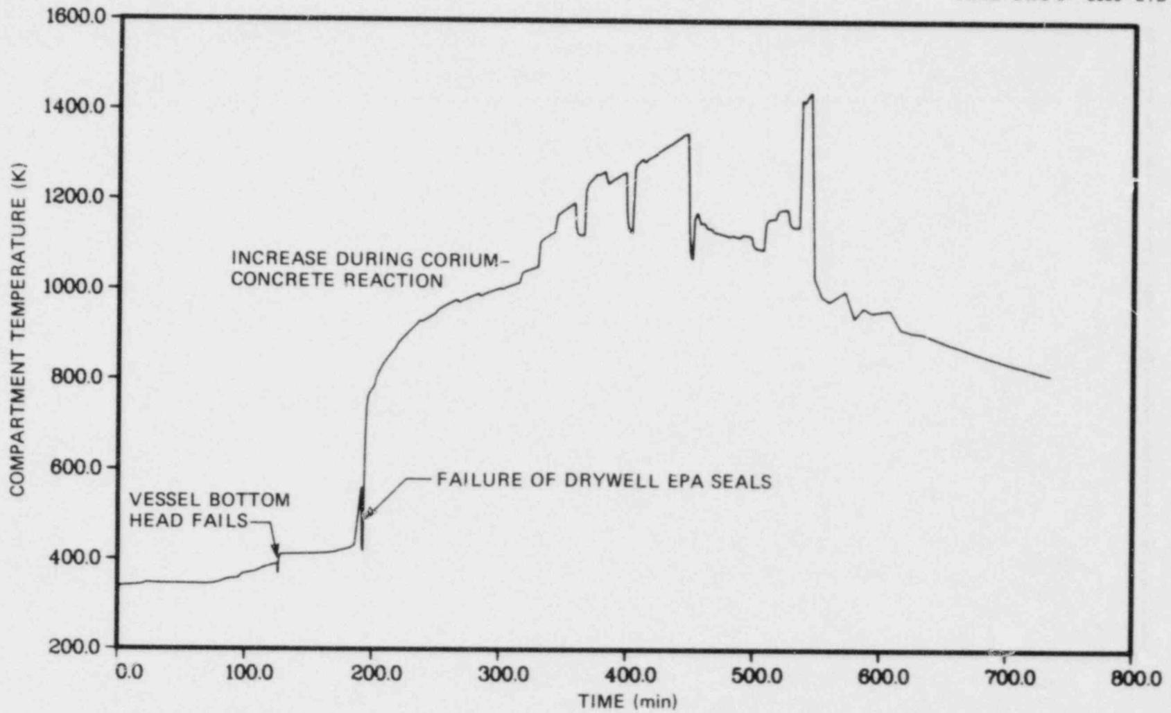
Fig. 9.28 Drywell temperature distribution (TUB').
