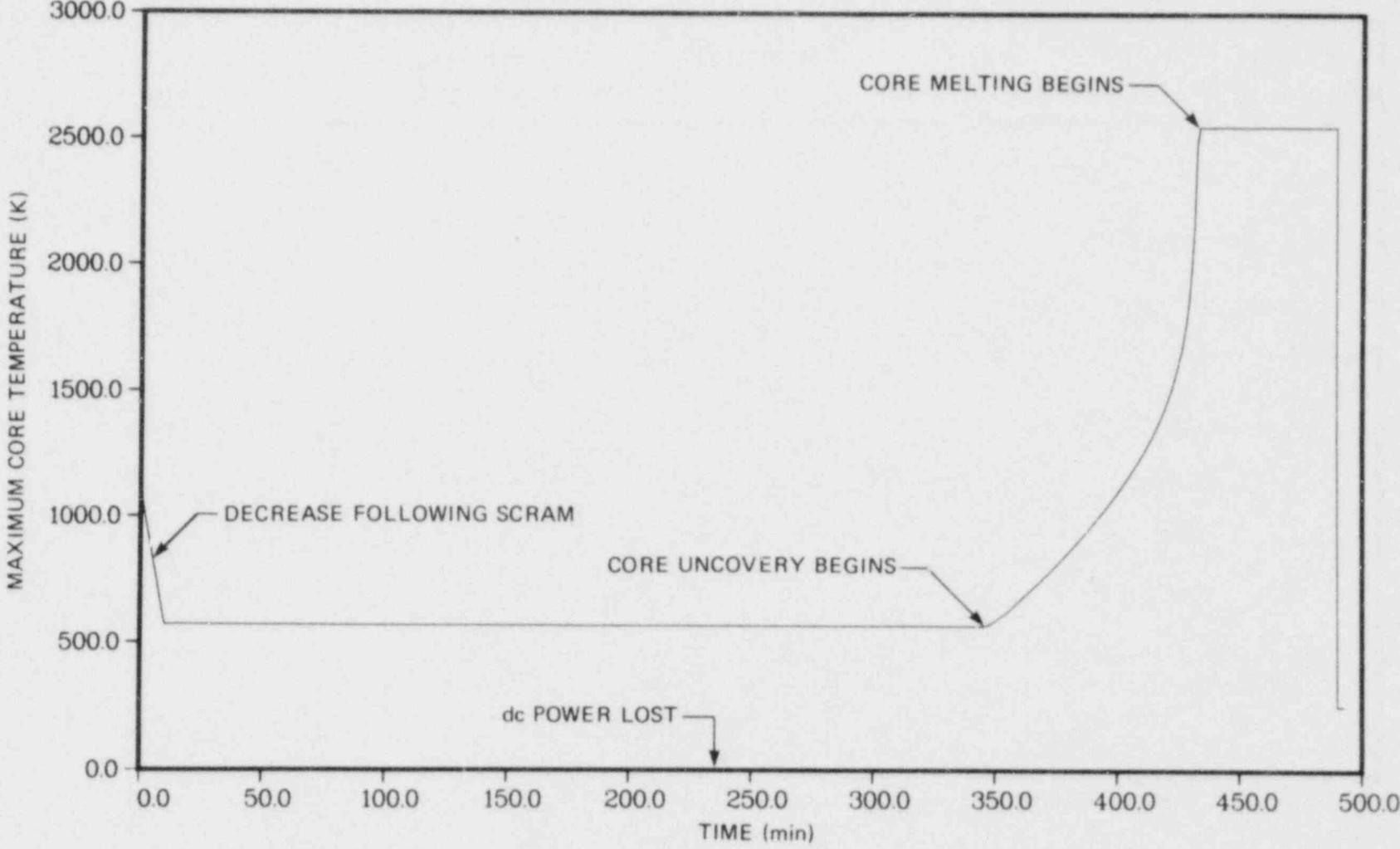
Fig. 9.5 Maximum core temperature (MARCH/MOD 1.4).
