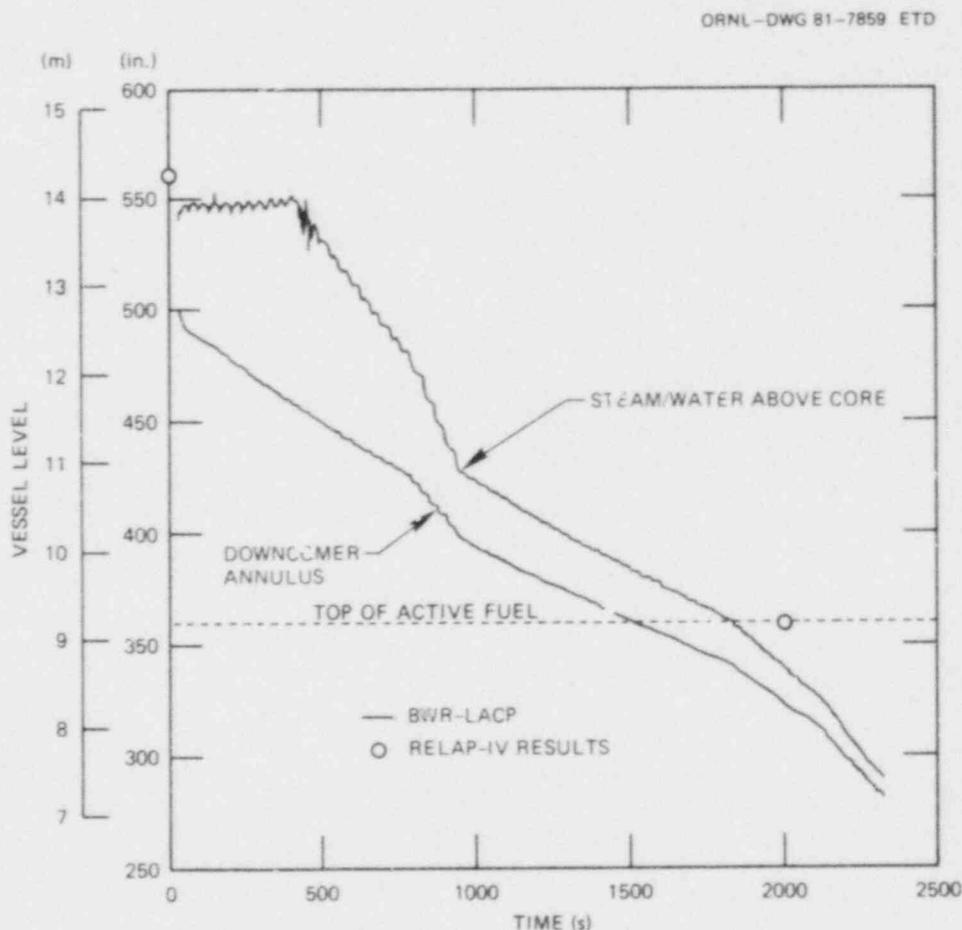
Fig. 4.5 Comparison of RELAP-IV and BWR-LACP results for reactor vessel level.
