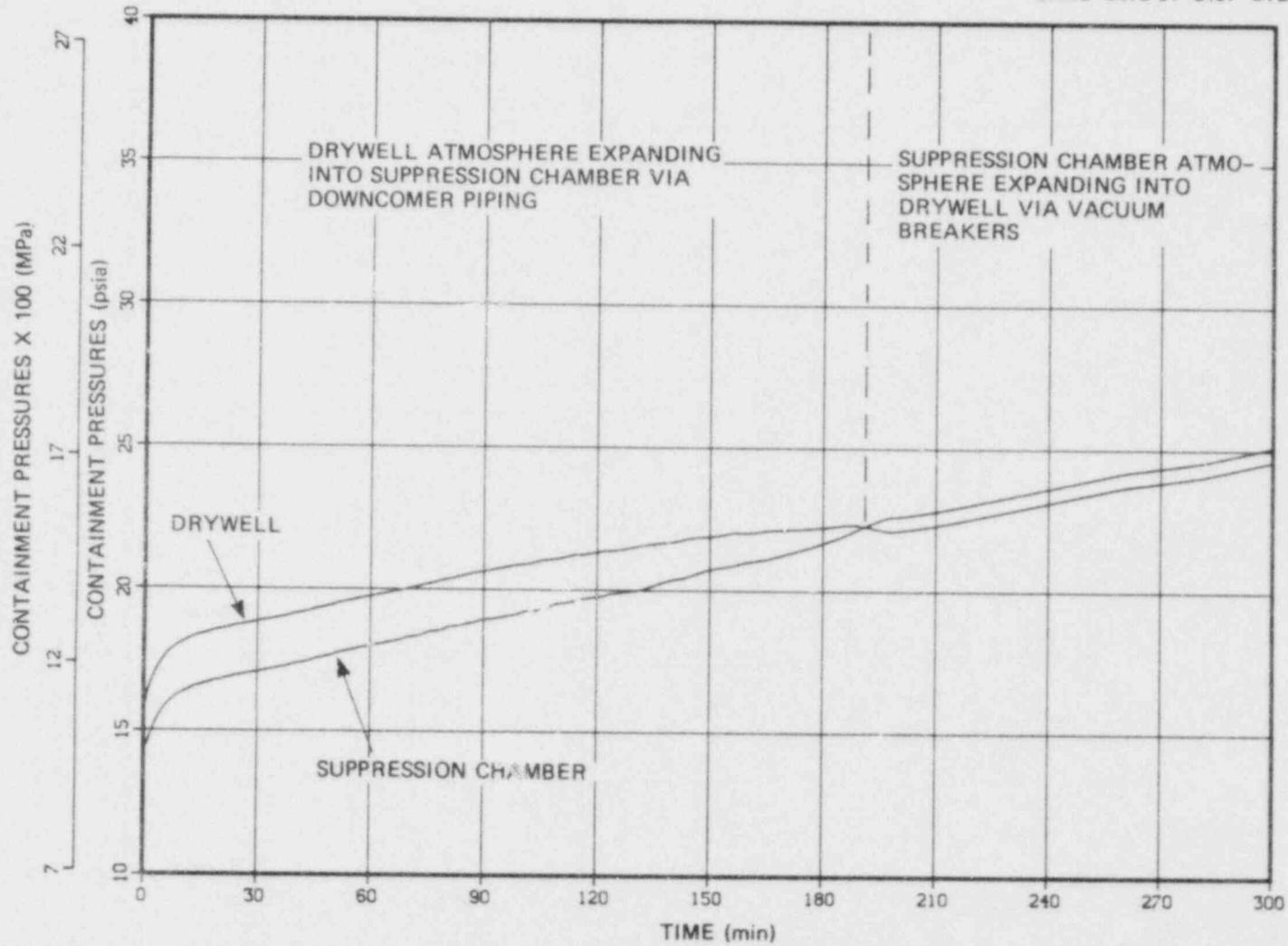
Fig. 7.9 Normal recovery after station blackout - containment pressures.
