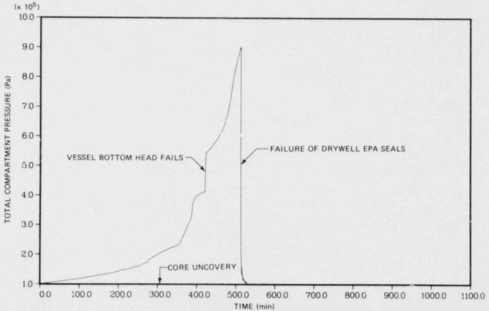
Fig. 9.29 Drywell total pressure (TB').
