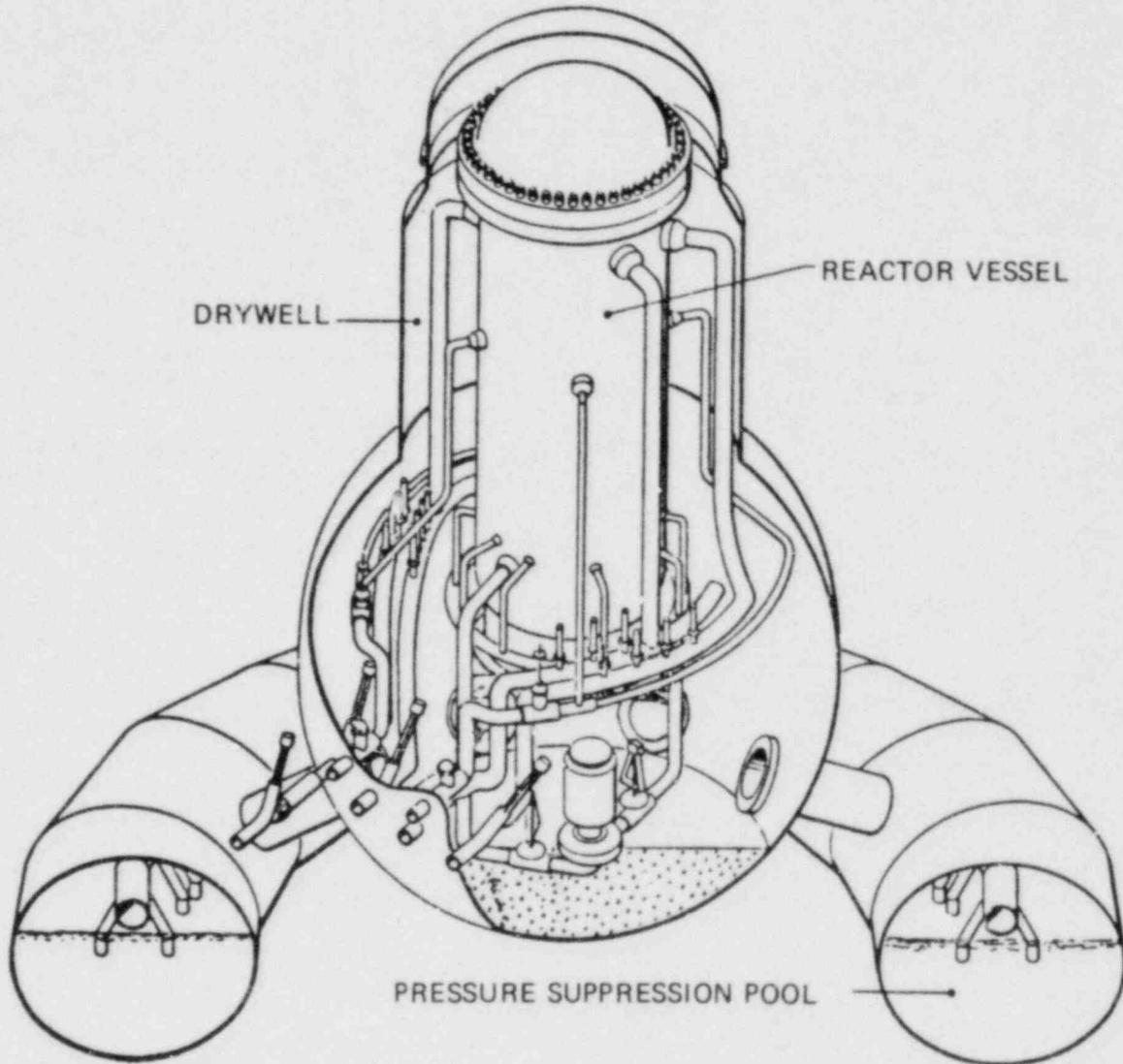
Fig. 3.1 Arrangement of drywell and torus.
