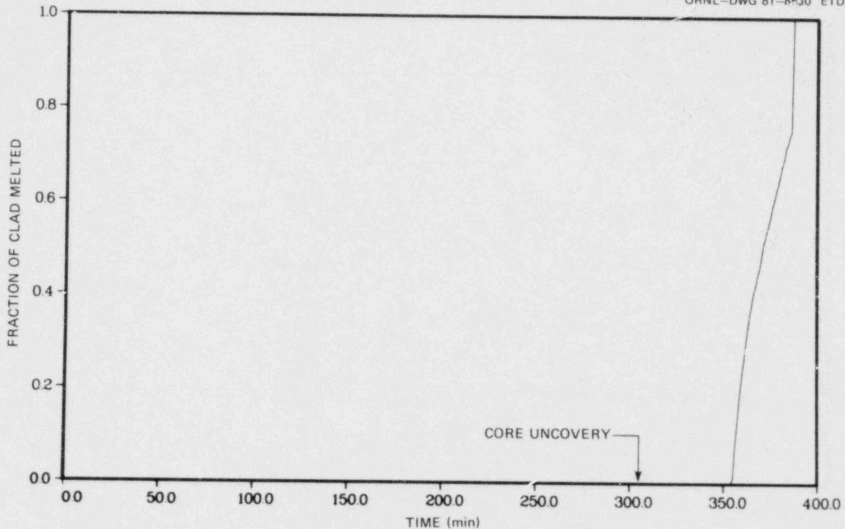
Fig. 9.19 Fraction of core melted.
