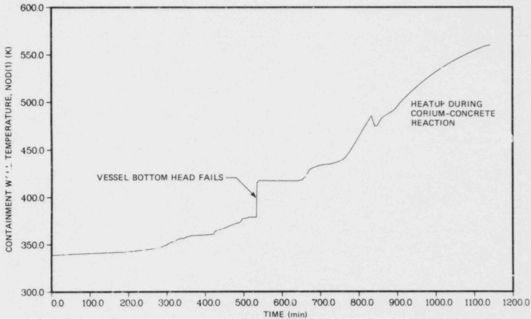
Fig. 9.9 Containment wall temperature (MARCH/MOD 1.4).
