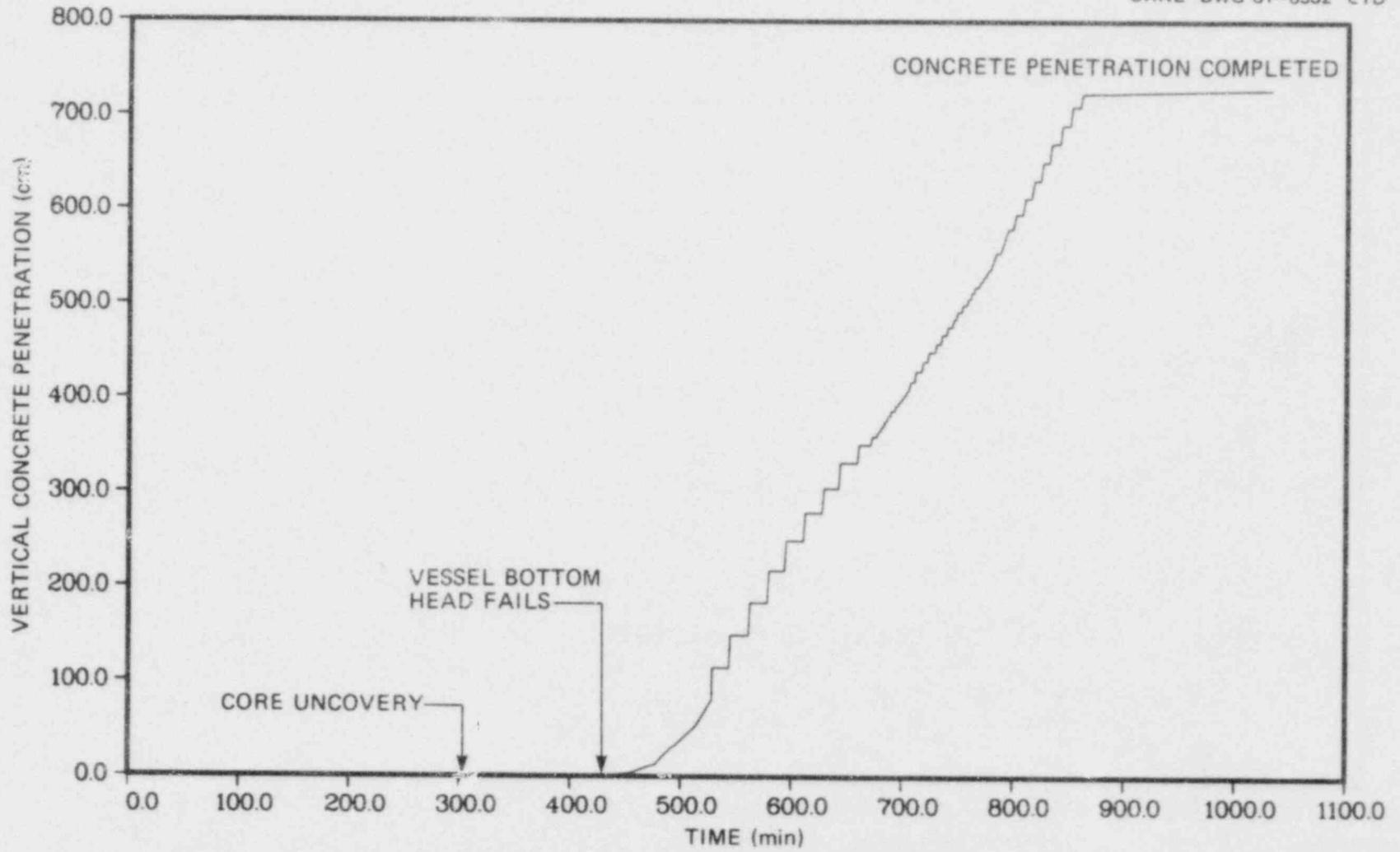
Fig. 9.21 Vertical concrete penetration.
