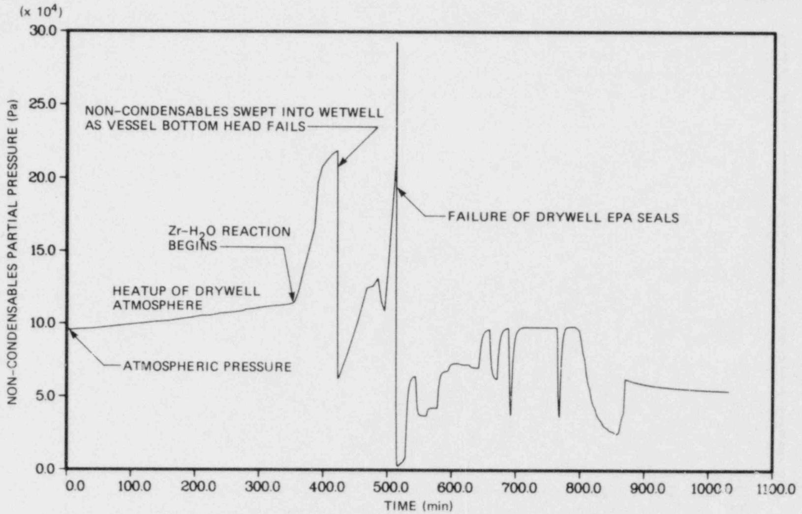
Fig. 9.32 Drywell non-condensables partial pressure (TB').
