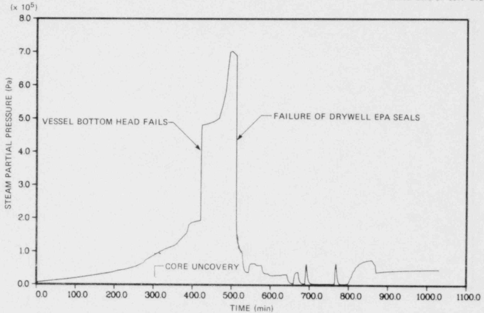
Fig. 9.30 Drywell steam partial pressure (TB').
