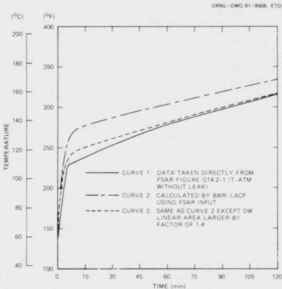
Fig. 4.4 Drywell atmosphere temperature: comparison of FSAR and ORNL BWR-LACP results.
