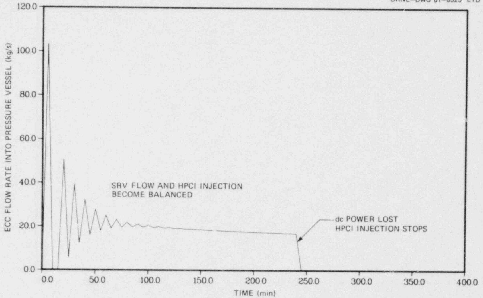
Fig. 9.14 HPCI flow rate into pressure vessel.
