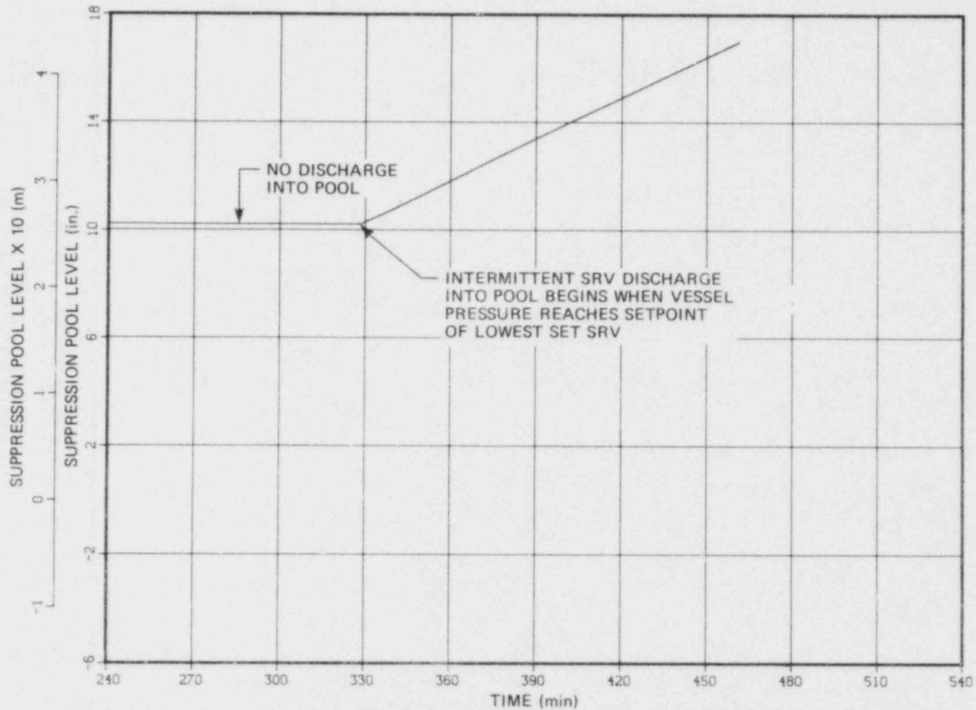
Fig. 7.13 Loss of 250 VDC batteries - suppression pool level.
