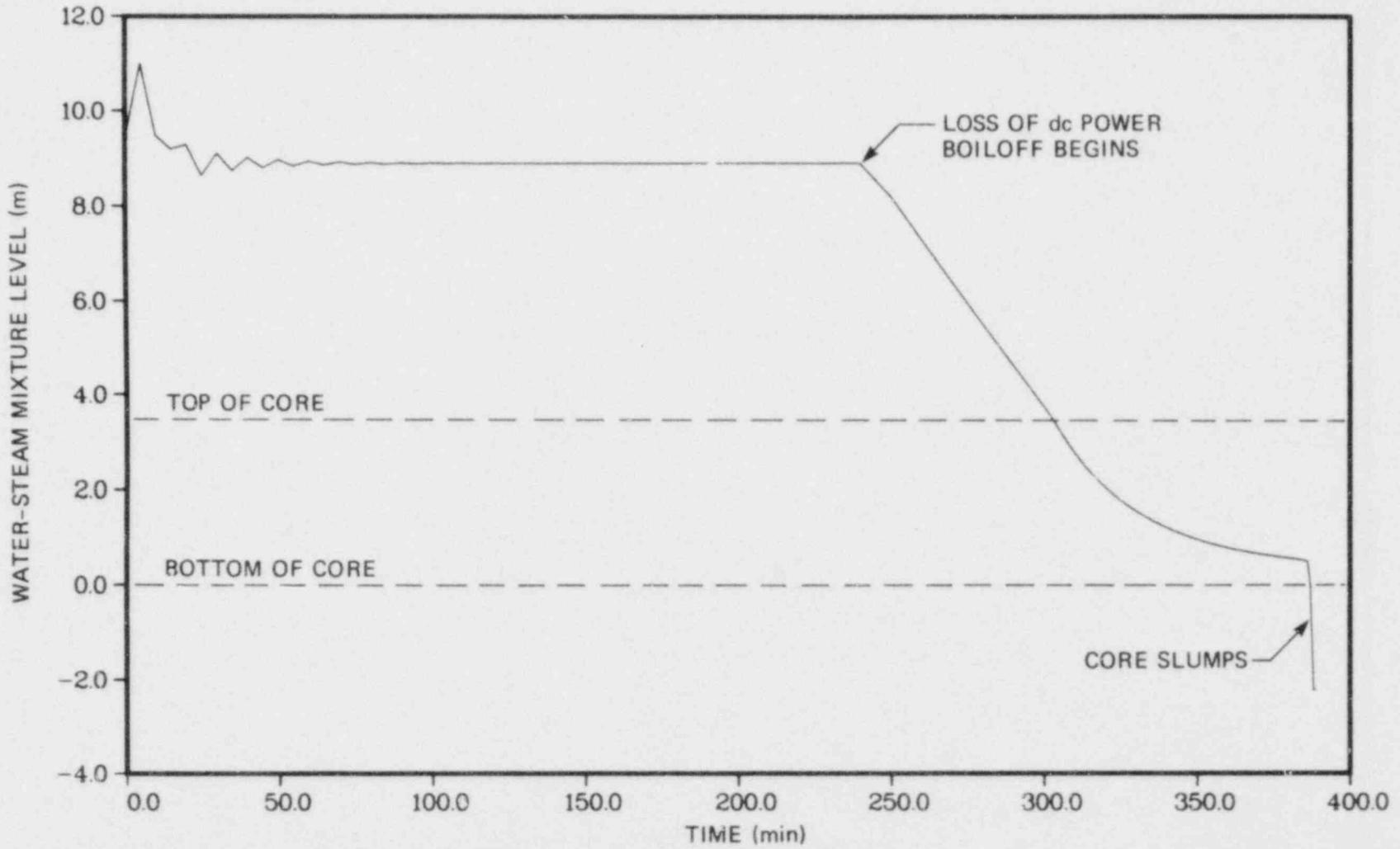
Fig. 9.6 Water-steam mixture level (MARCH/MOD 1.4B).
