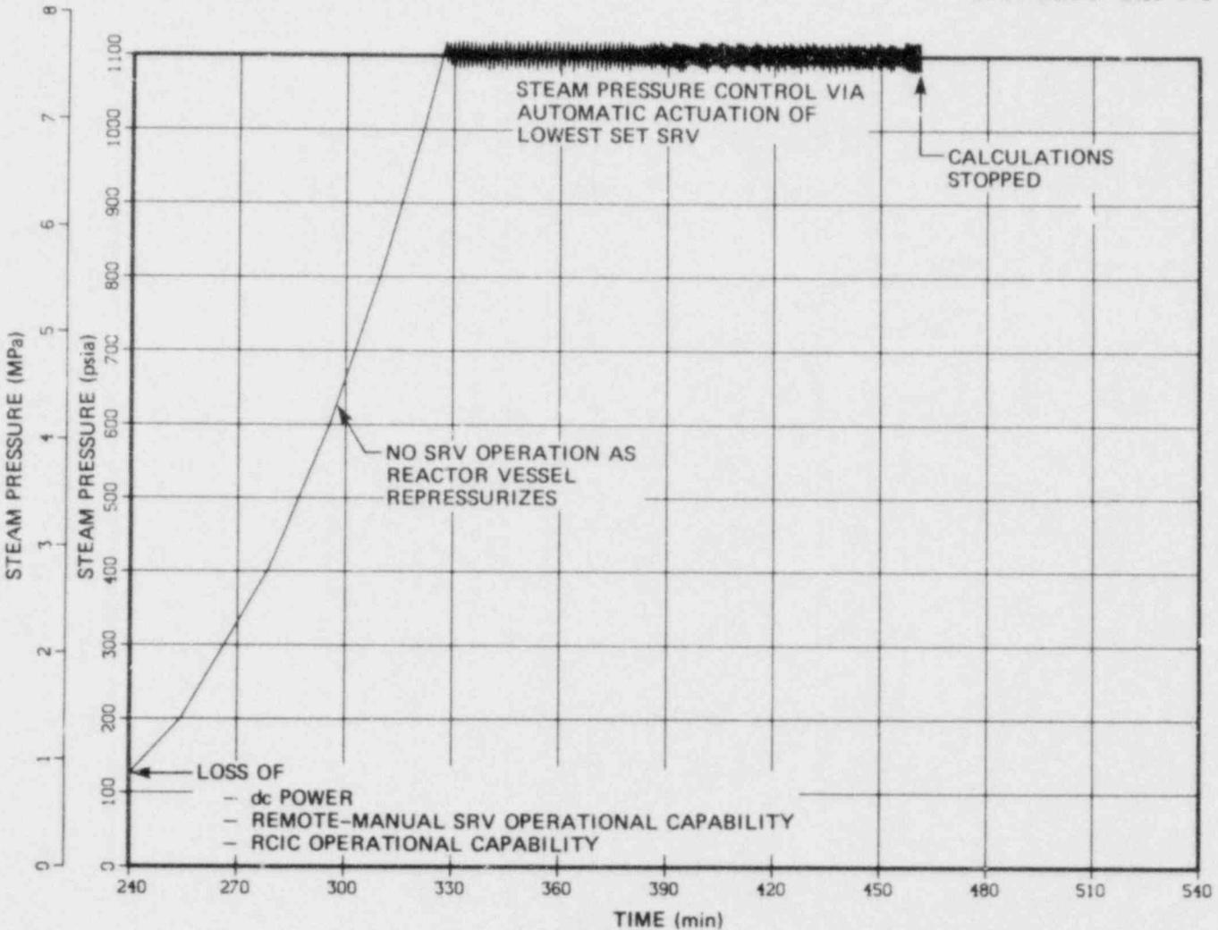
Fig. 7.10 Loss of 250 VDC batteries - reactor vessel pressure.
