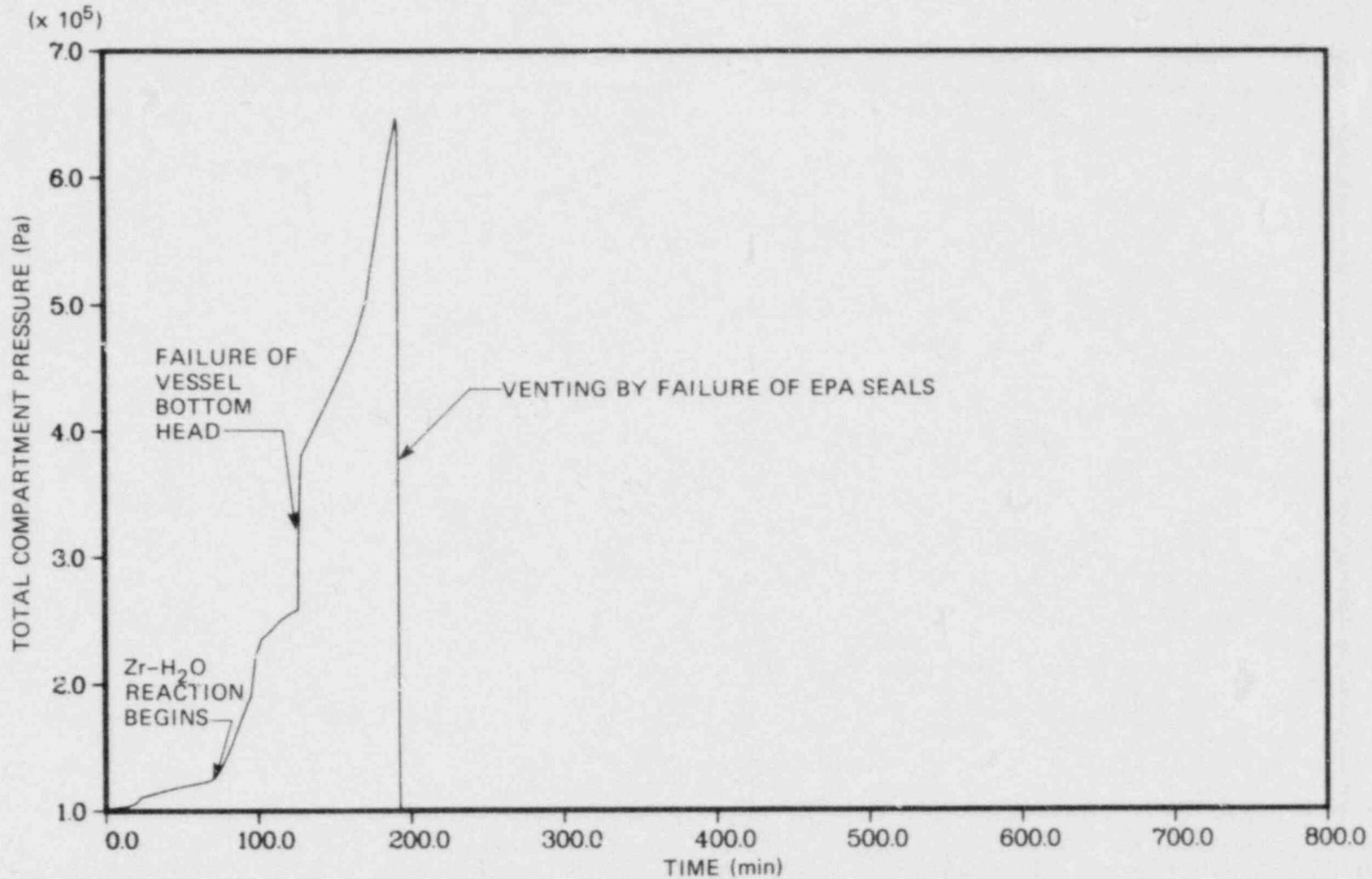
Fig. 9.43 Wetwell total pressure (TUB').
