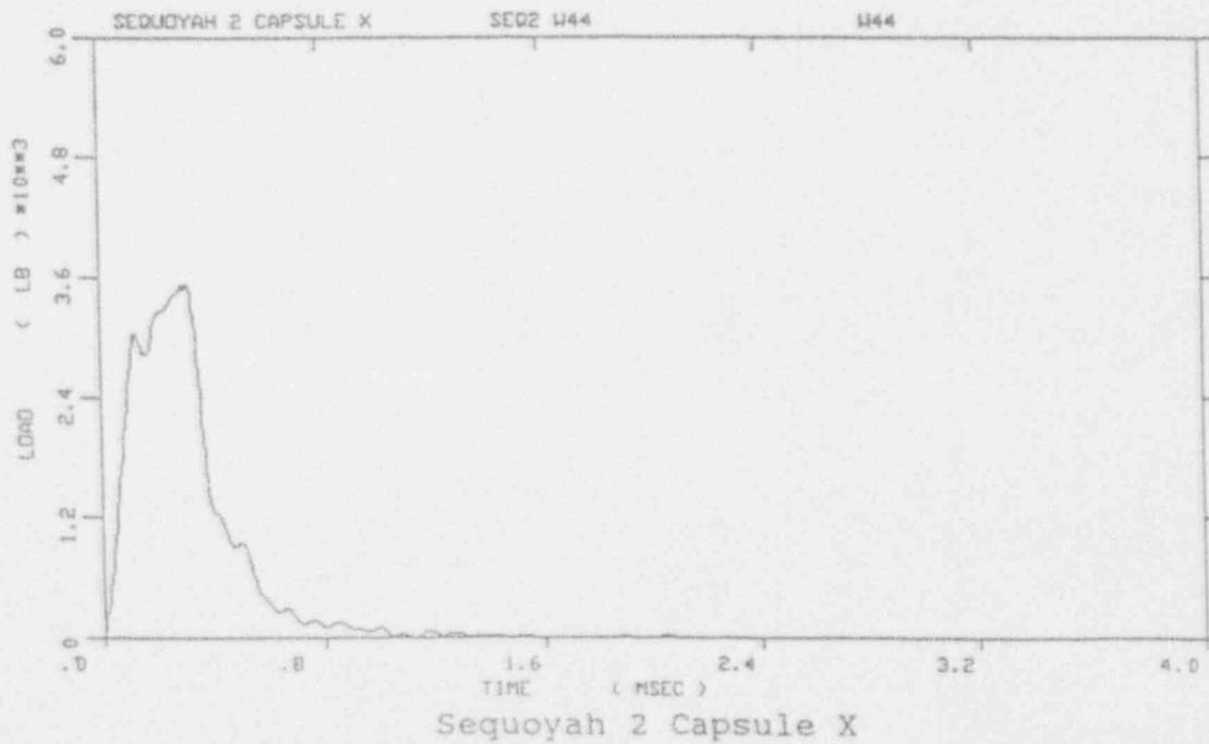
Figure A-15. Load-time records for Specimens W37 and W44
