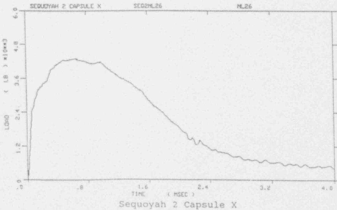
Figure A-5. Load-time records for Specimens NL27 and NL26
