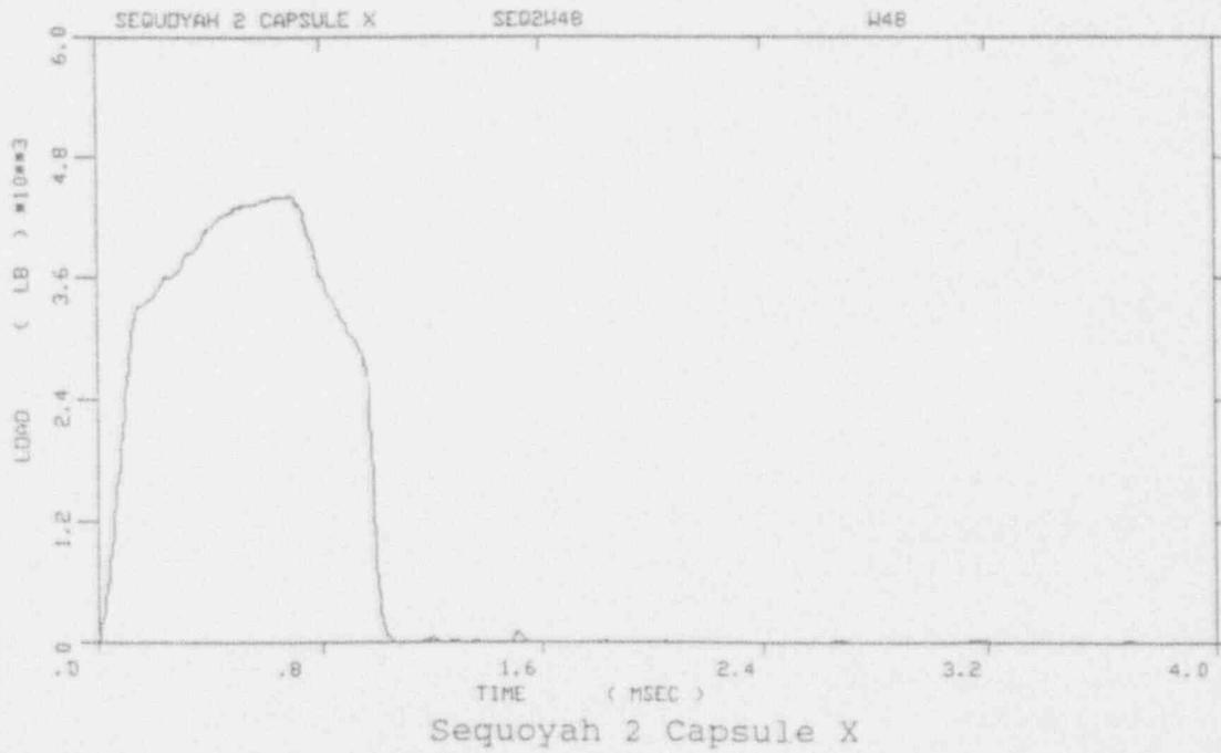
Figure A-14. Load-time records for Specimens W39 and W48
