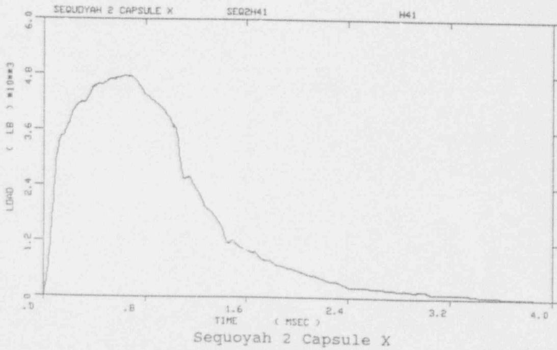
Figure A-21. Load-time records for Specimens H48 and H41
