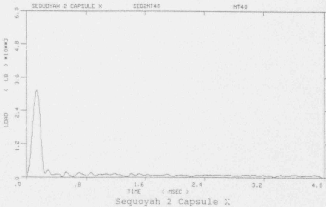
Figure A-6. Load-time records for Specimens NT42 and NT40
