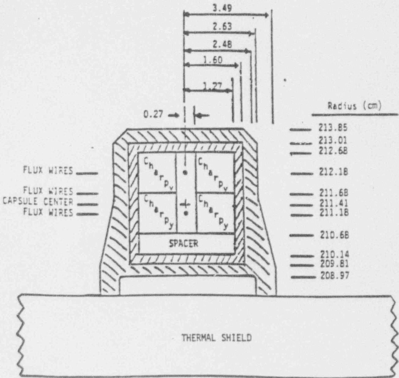
Figure 6-1. Plan View of a Reactor Vessel Surveillance Capsule
