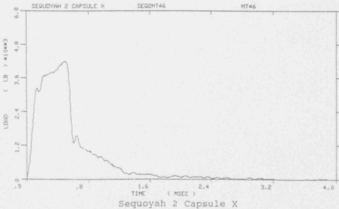
Figure A-8. Load-time records for Specimens NT39 and NT46
