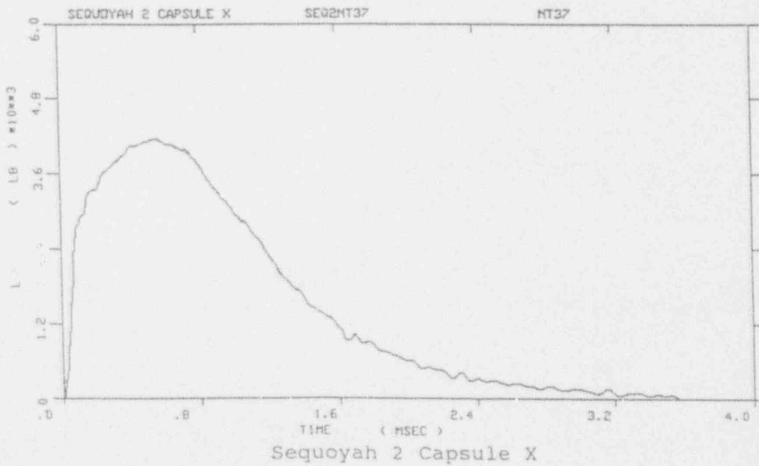
Figure A-11. Load-time records for Specimens NT48 and NT37
