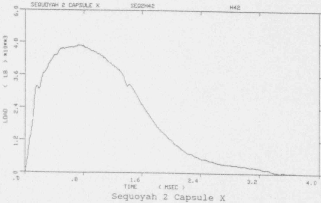
Figure A-23. Load-time records for Specimens H44 and H42
