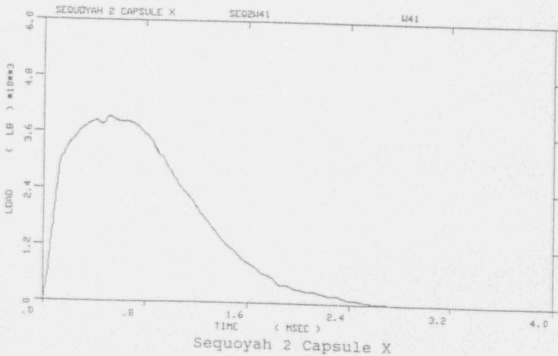
Figure A-17. Load-time records for Specimens W46 and W41
