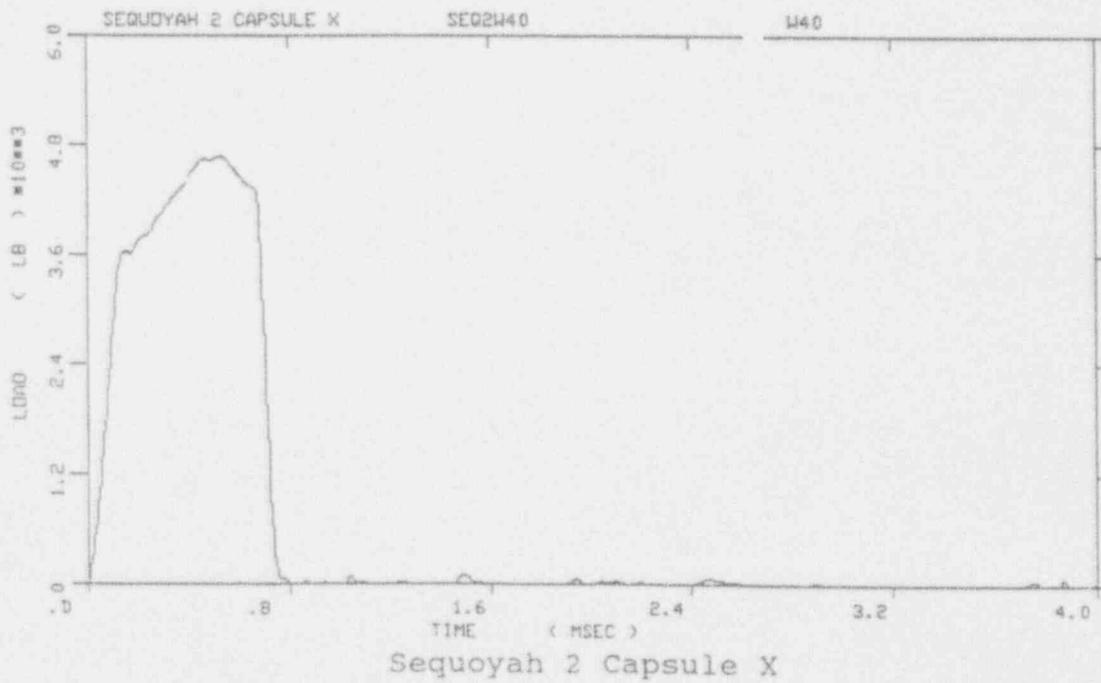
Figure A-13. Load-time records for Specimens W47 and W40
