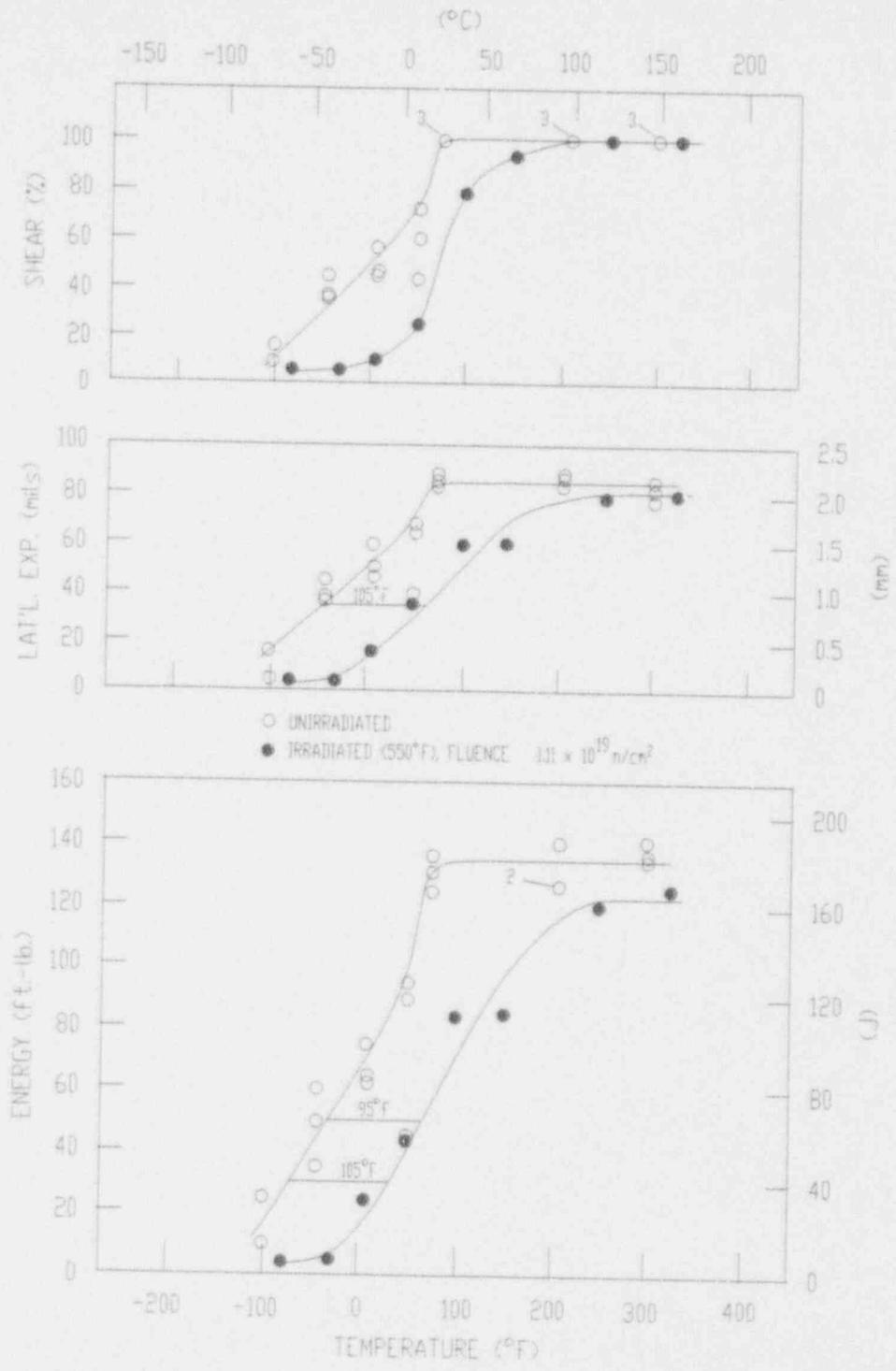
Figure 5-2. Charpy V-Notch Impact Properties for Sequoyah Unit 2 Reactor Vessel Intermediate Shell Forging 05 (Tangential Orientation)
