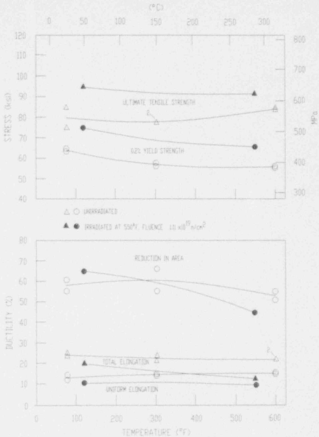
Figure 5-9. Tensile Properties for Sequoyah Unit 2 Reactor Vessel Intermediate Shell Forging 05 (Axial Orientation)
