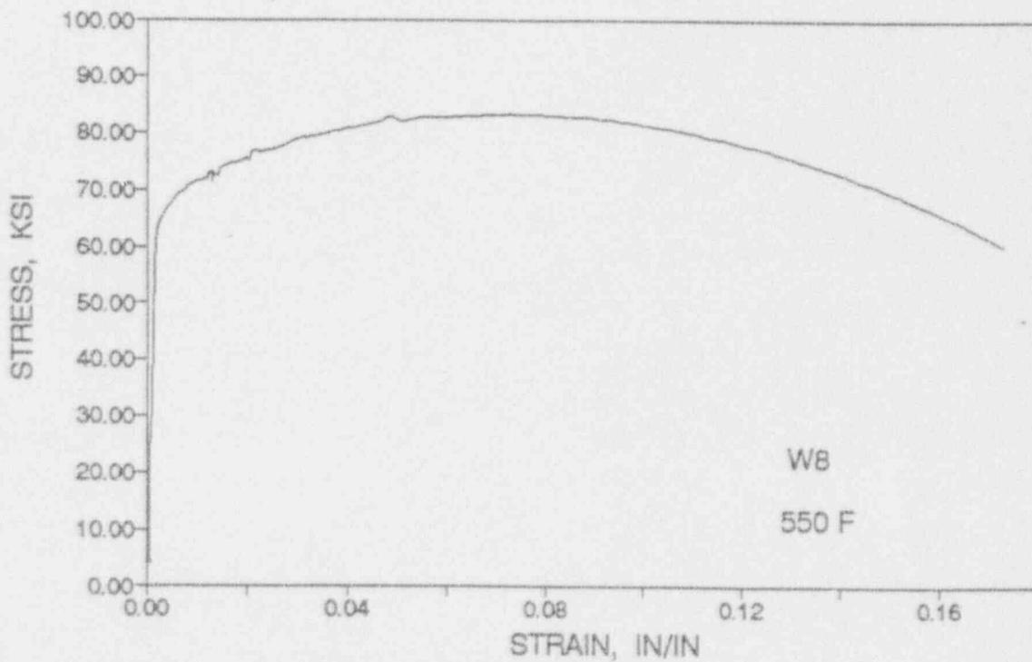
Figure 5-14. Engineering Stress-Strain Curve for Weld Metal Tensile Specimens W7 and W8
