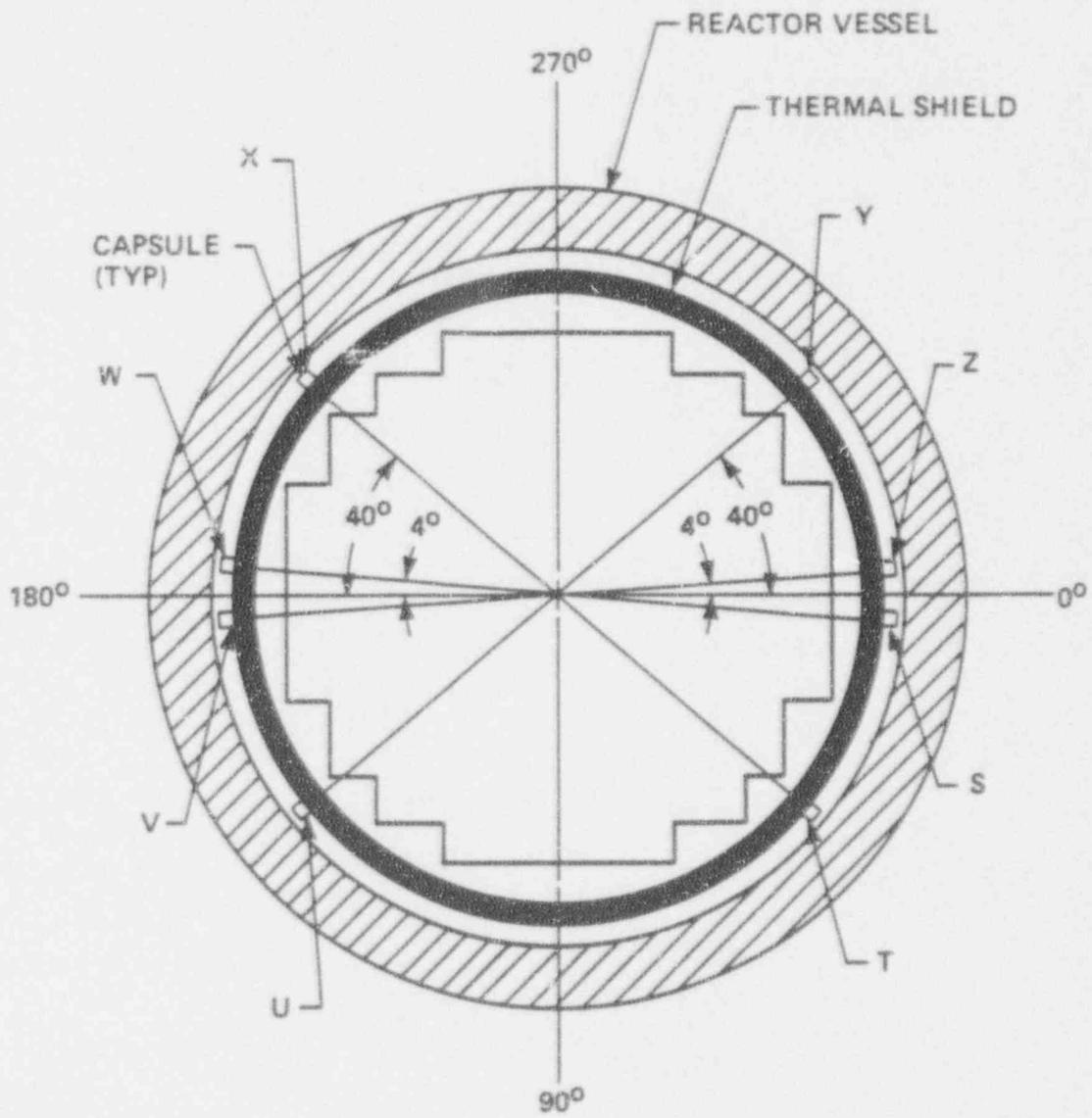
Figure 4-1. Arrangement of Surveillance Capsules in the Sequoyah Unit 2 Reactor Vessel
