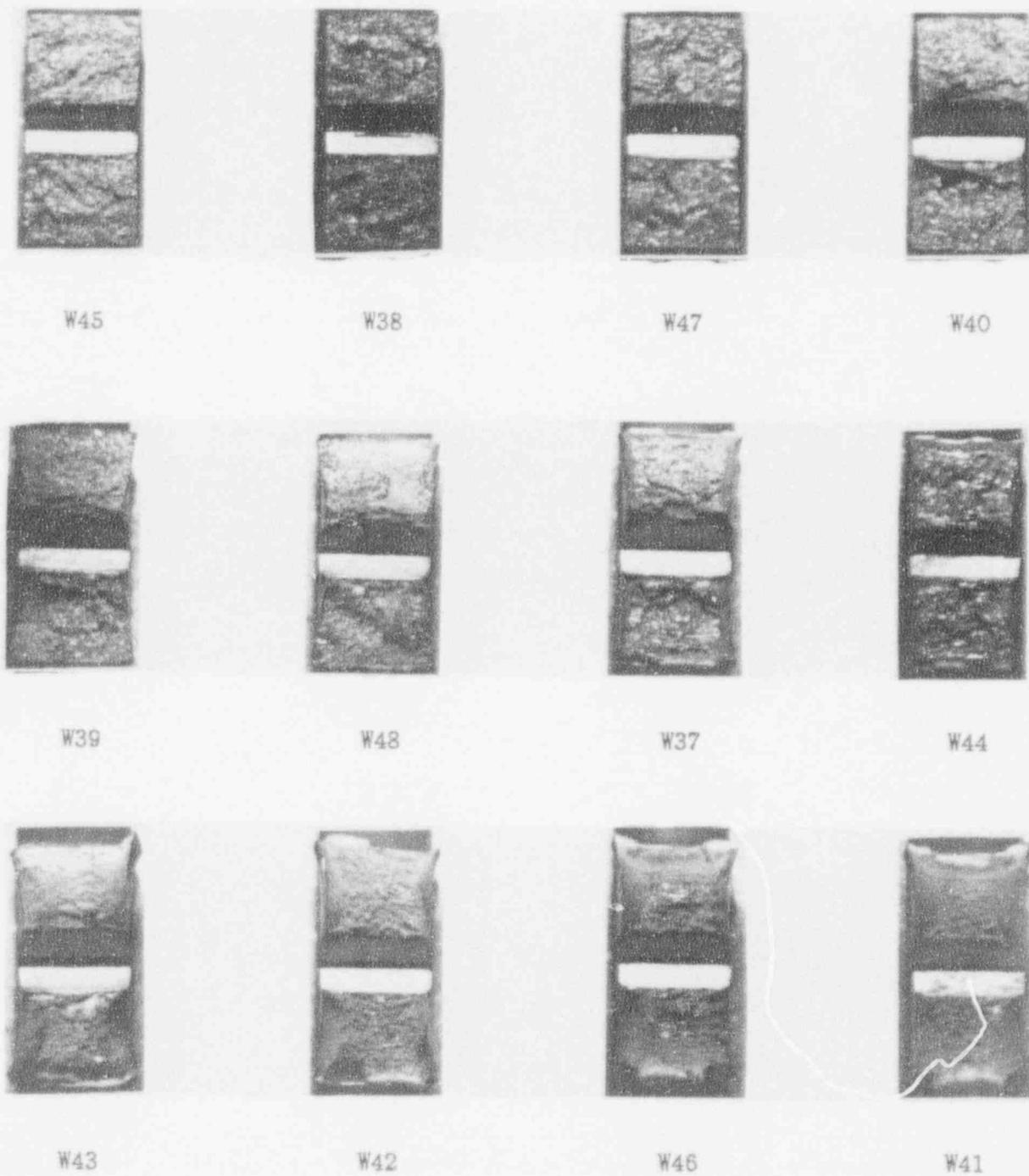
Figure 5-7. Charpy Impact Specimen Fracture Surfaces for Sequoyah Unit 2 Reactor Vessel Surveillance Weld Metal
