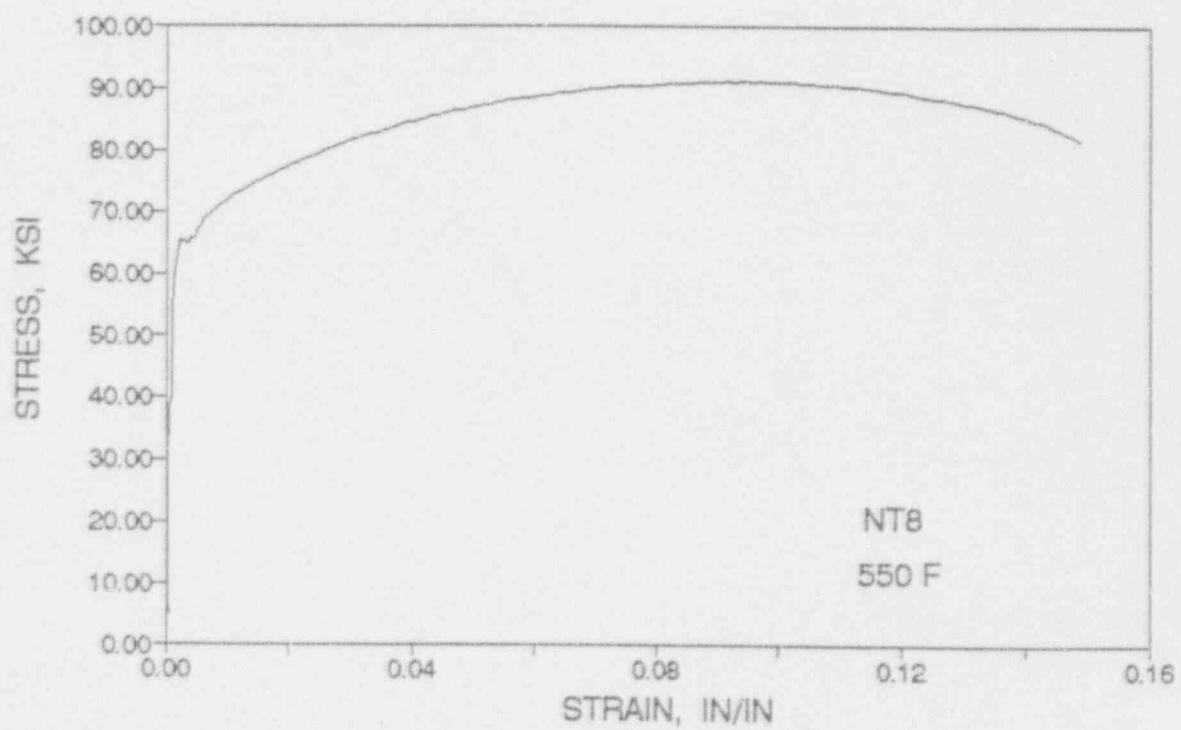
Figure 5-13. Engineering Stress-Strain Curves for Forging 05 Tensile Specimens NT7 and NT8
