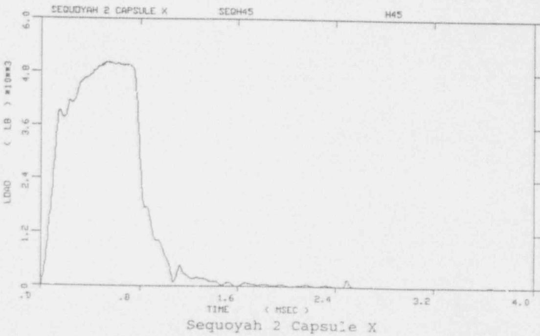
Figure A-20. Load-time records for Spec. H47 and H45
