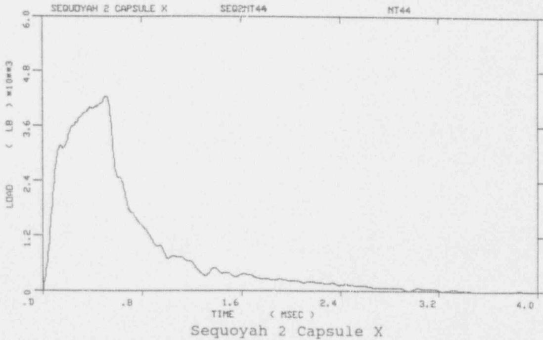
Figure A-9. Load-time records for Specimens NT41 and NT44
