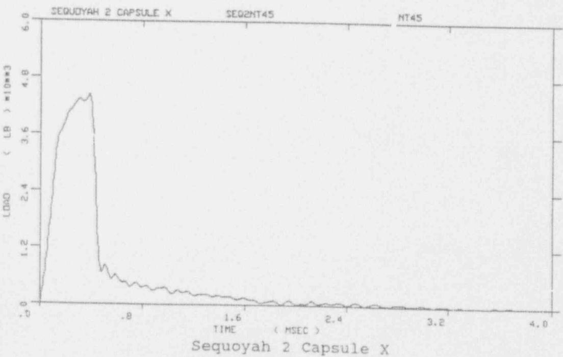
Figure A-7. Load-time records for Specimens NT38 and NT45
