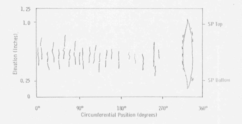
Figure 1 Sketch of the crack distribution found at the second support plate crevice region of Tube R14-C80. Included is the location of the burst test fracture face opening. The OD origin intergranular corrosion was confined to the crevice region, including that found on the burst fracture face.
