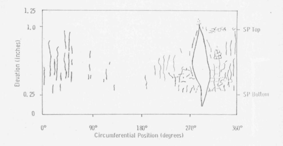
Figure 2 Sketch of the crack distribution found at the first support plate crevice region of Tube R19-C41. Included is the location of the burst test fracture face opening. All deep OD origin intergranular corrosion was confined to the crevice region, including that found on the burst fracture face. Some minor intergranular corrosion was observed up to 0.2 inch above the crevice top.
