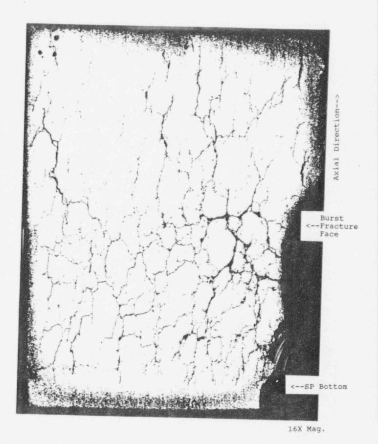
Figure 3 Radial metallography of the SP1 region of Tube R19-C41 showing intergranular cellular corrosion (ICC).
