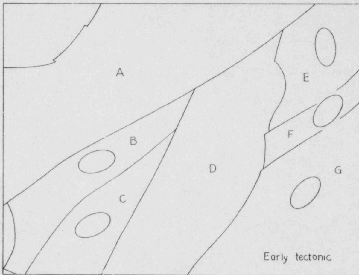
Figure 4b. Map of the Cape Ann area, showing the horizontal projection of the greatest and least principal stress, calculated from joint data, during early regional tectonic events. Letters refer to fault bounded blocks shown on Figure 2.
