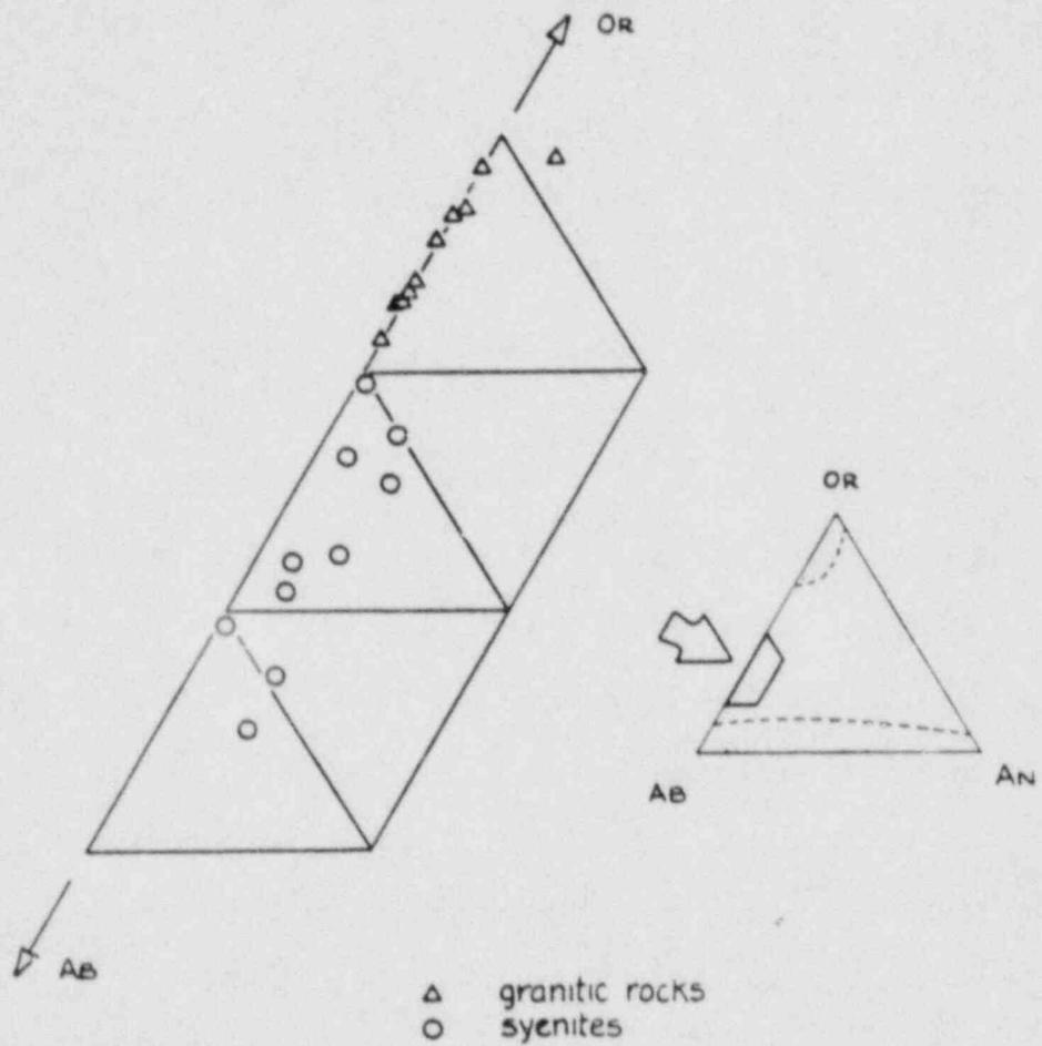
Figure 7. Ternary diagram showing the original composition of homogenized feldspar in salic rocks of the Cape Ann Plutonic Series between orthoclase (OR), anorthite (AN) and albite (AB), end members (from Toulmin, 1964).
