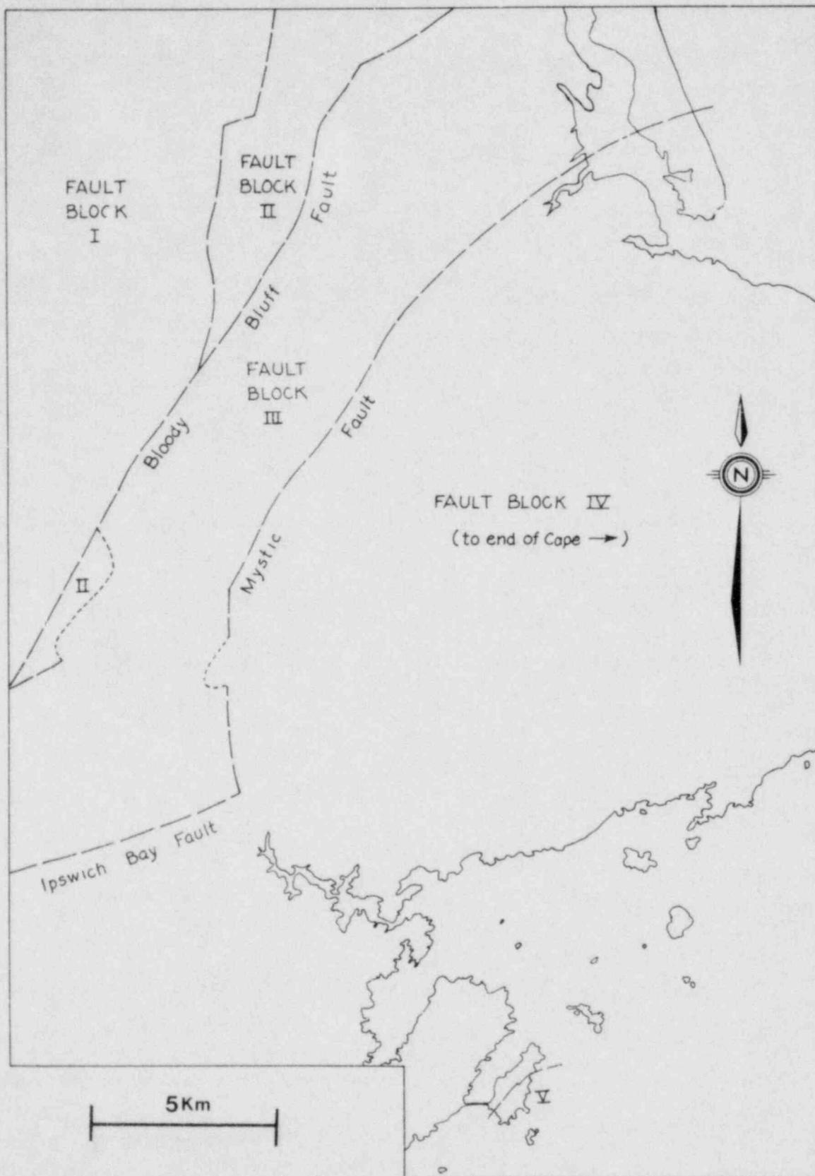
Figure 1. Map of the Cape Ann area, showing faults bounding blocks of the principal lithologic assemblages.
