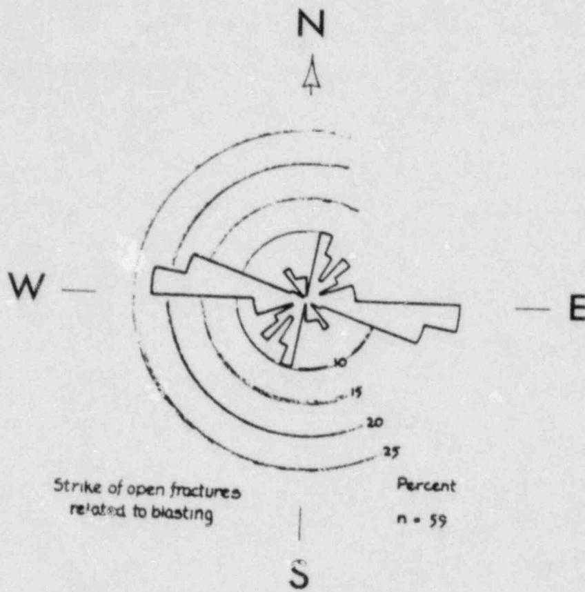
Figure 5. Diagram showing the orientation of relief cracks associated with highway and quarry blasting on Cape Ann.
