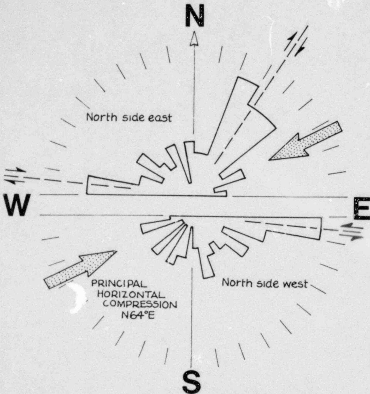
Figure A-3. Diagram showing the orientation and direction of apparent movement on stepped joints and derived direction of principal horizontal compression on Cape Ann.
