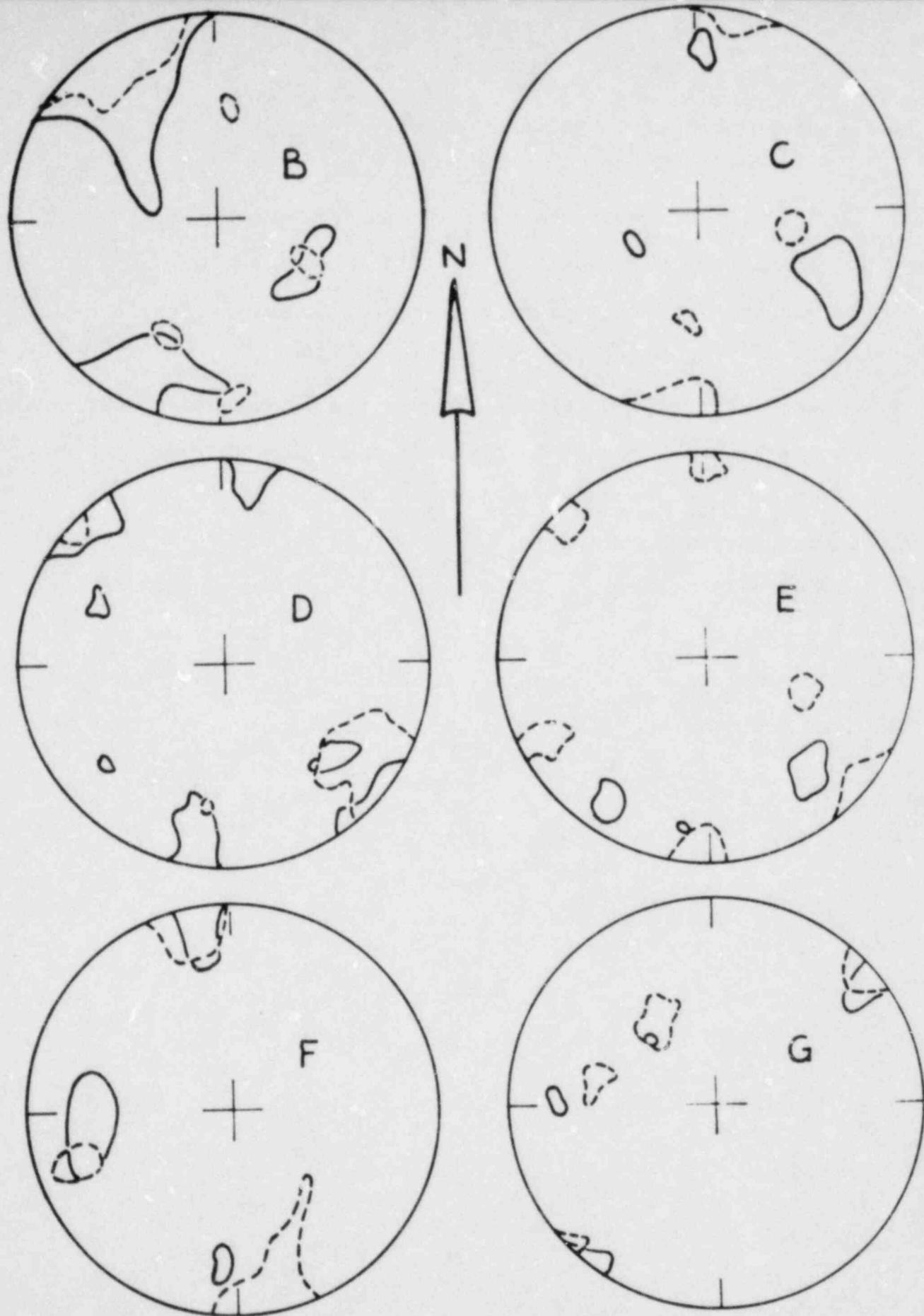
Figure A-1. Diagrams showing contoured polar projections to the lower hemisphere of an equal-area net of consolidation and tectonic joint data. Joints ascribed to consolidation shown as solid contours, joints ascribed to tectonism as dashed contours (Figs. 4a and 4b). Letters refer to fault bounded blocks shown on Figure 2. 80
