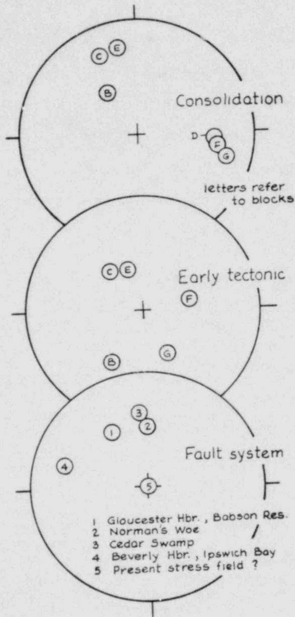
Figure 6. Diagram showing polar projections of the intermediate stress to the lower hemisphere of an equal area net for jointing related to consolidation, early tectonic and fault effects. (Figs. 4a, 4b, and 4c).
