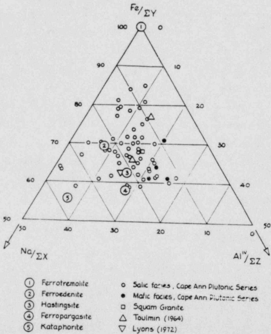
Figure 8. Ternary diagram showing the hornblende composition in the Cape Ann Plutonic Series between iron (Fe/ΣY), aluminum (Al<sup>IV</sup>/ΣZ) and sodium (Na/ΣX) end member.
