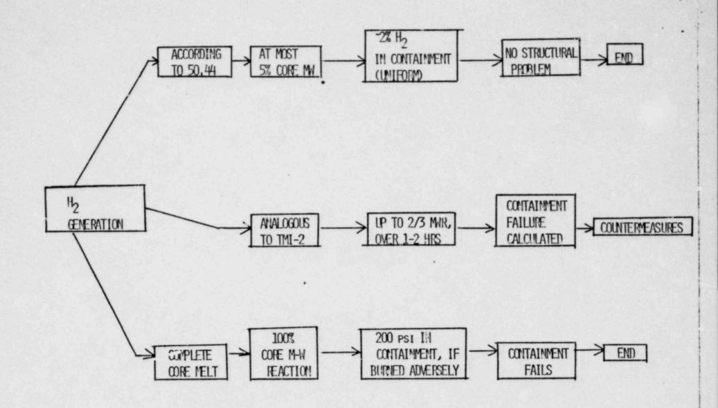
ADIABATIC CONTAINMENT HYDROGEN COMBUSTION CALCULATION
