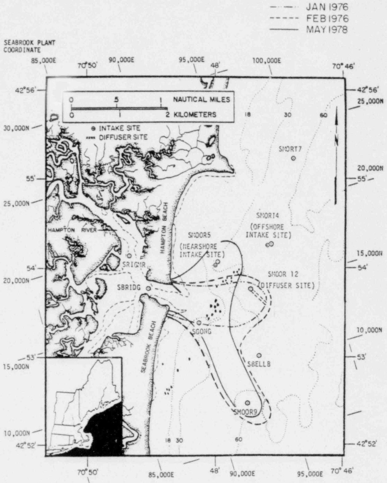
Figure 4.1-1. Schematic of the Observed Ebb Tidal Plumes in January and February, 1976 and May 1978. Seabrook Annual Hydrographic Report, 1978.
