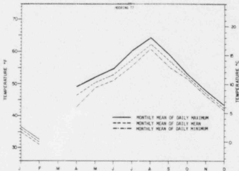
Figure 3.2-2. Summary plots of the monthly means of daily maxima, daily mean and daily minima of temperature at Mooring T-7 during 1978. Seabrook Annual Hydrographic Report, 1978.
