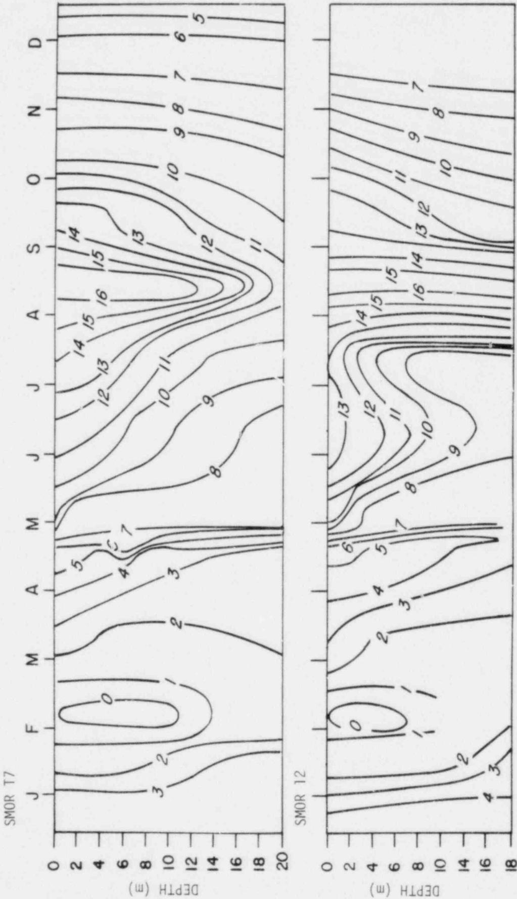
Figure 3.2-7. Vertical distribution of temperature at SMOR 7 and SMOR 12 during 1978. Contour interval is 1C. Seabrook Annual Hydrographic Report, 1978.
