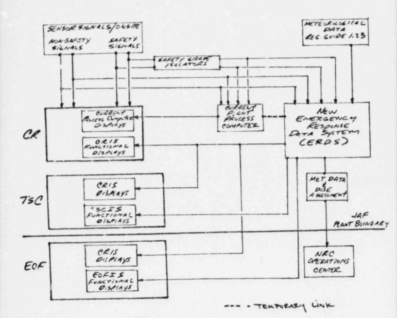
C.R. - MAIN CONTROL ROOM TSC - TECHNICAL SUPPORT CENTER EOF - EMERGENCY OPERATIONS FACILITY The ERDS functions of each system are:
