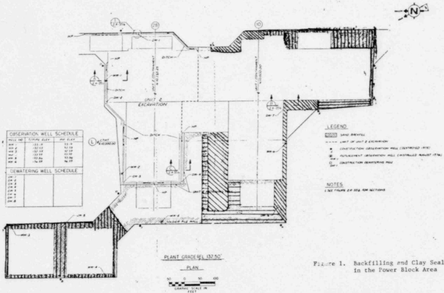
Figure 1. Backfilling and Clay Sealing in the Power Block Area
