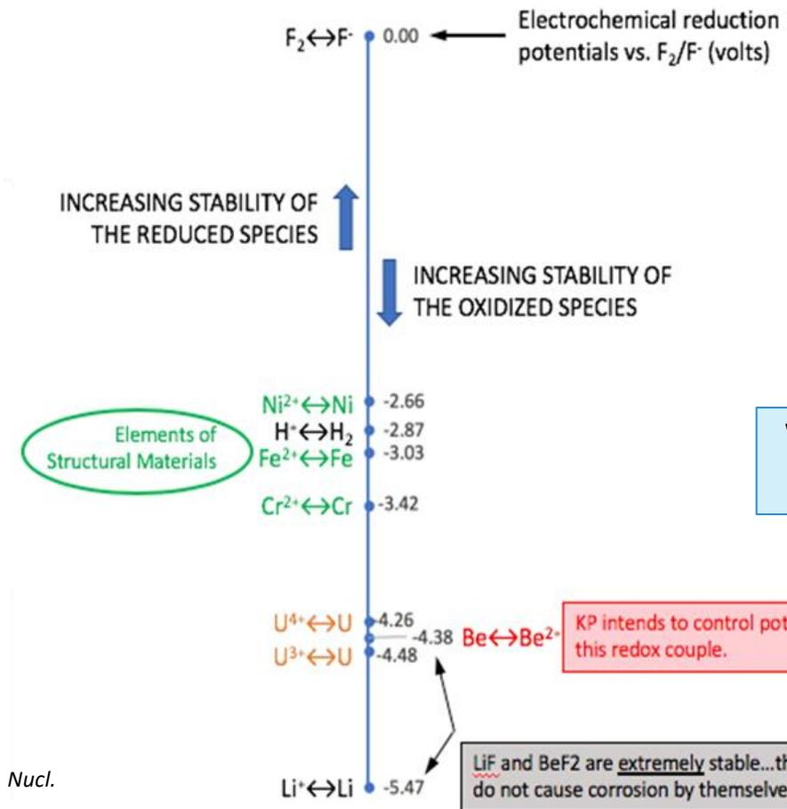
See Keiser, DeVan, and Lawrence, JNM Vol. 85&86, 1979. With Be addition, 316 corrosion rates  $\rightarrow$  < 2 microns per year
