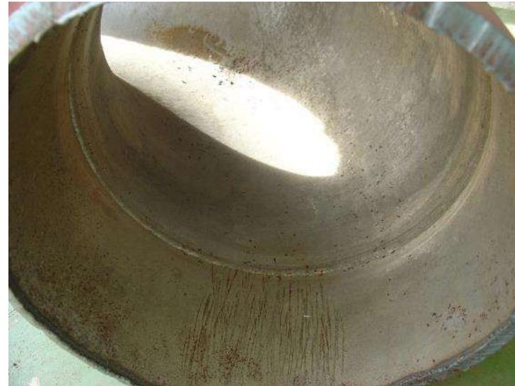
IHX outlet elbow inner and outer surface
