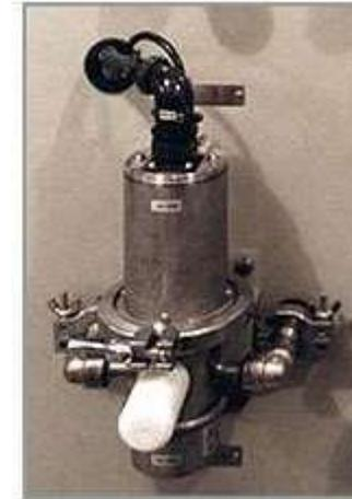
◆ **SID** is best suitable to detect sodium leak in the inert gas atmosphere (detector would burn if used in air).
