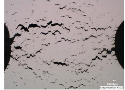
Creep cavitation (INL)
