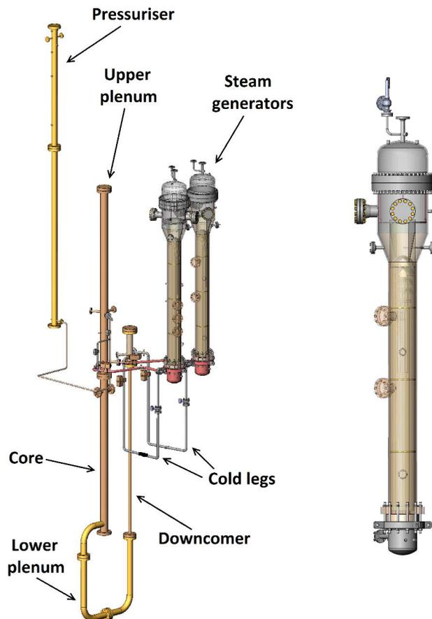
Figure 1 Schematic View of the PWR PACTEL Facility
