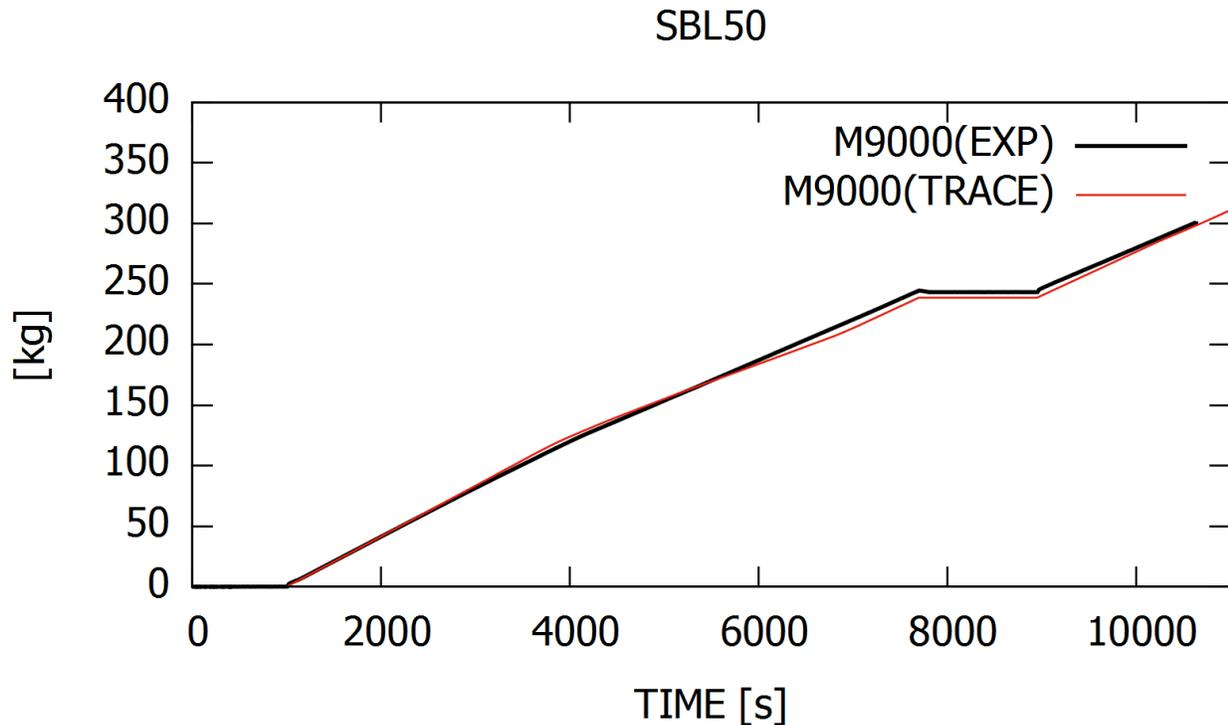
**Figure 5** Cumulative Break Flow in the PWR PACTEL Experiment SBL-50 vs. TRACE Calculation
