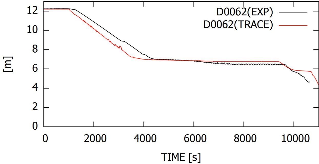
**Figure 7** Upper Plenum Collapsed Level in the PWR PACTEL Experiment (Exp) SBL-50 vs. TRACE Calculation
