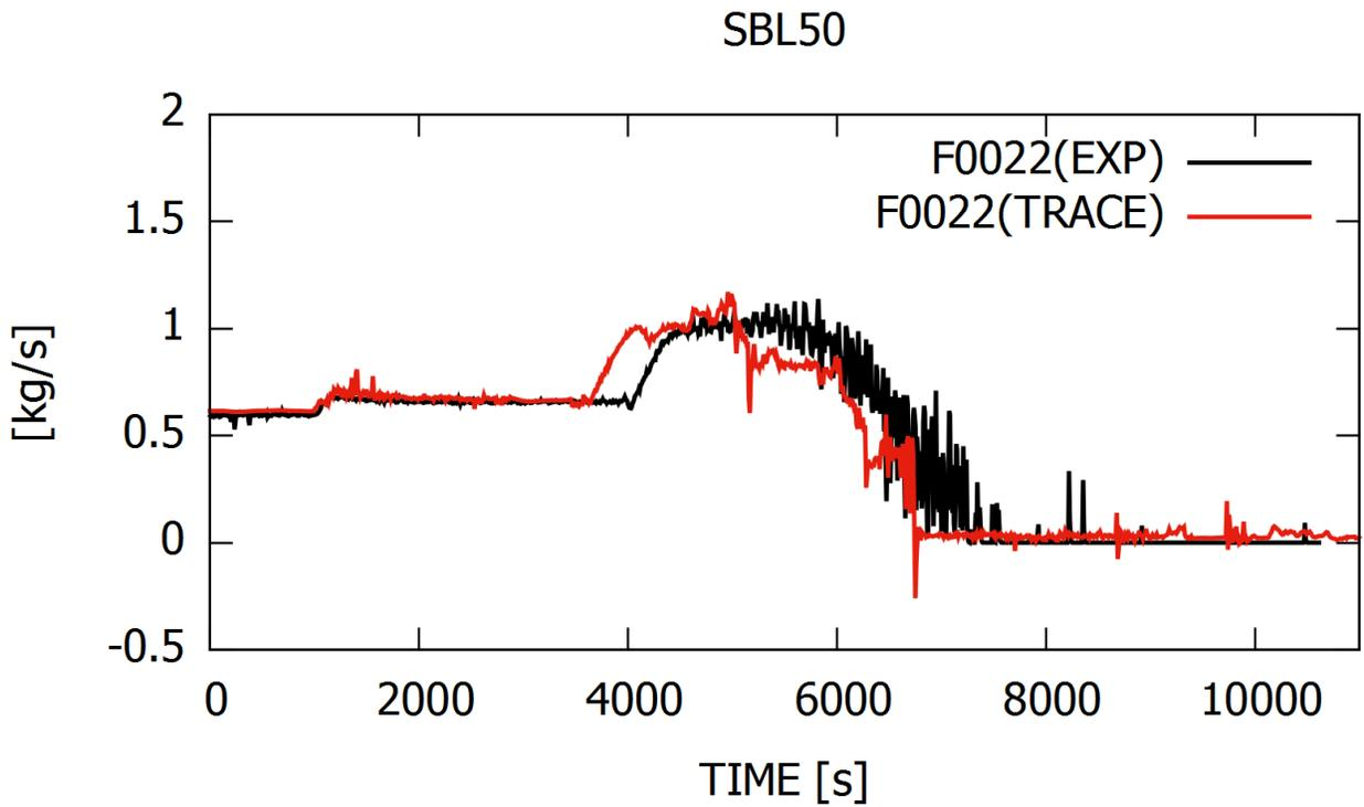
**Figure 10** Mass Flow Rate in Cold Leg 2 in the PWR PACTEL Experiment SBL-50 vs. TRACE Calculation
