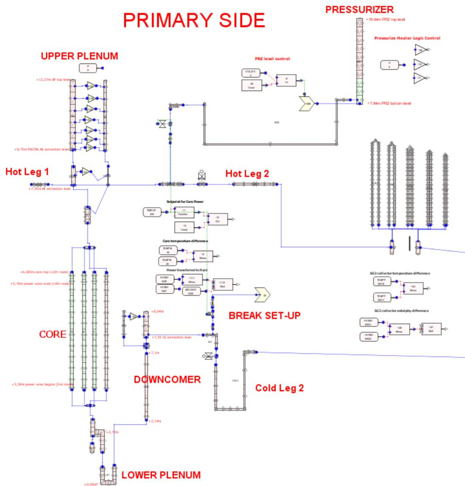
Figure 3 Primary Side of the PWR PACTEL TRACE/SNAP Model
